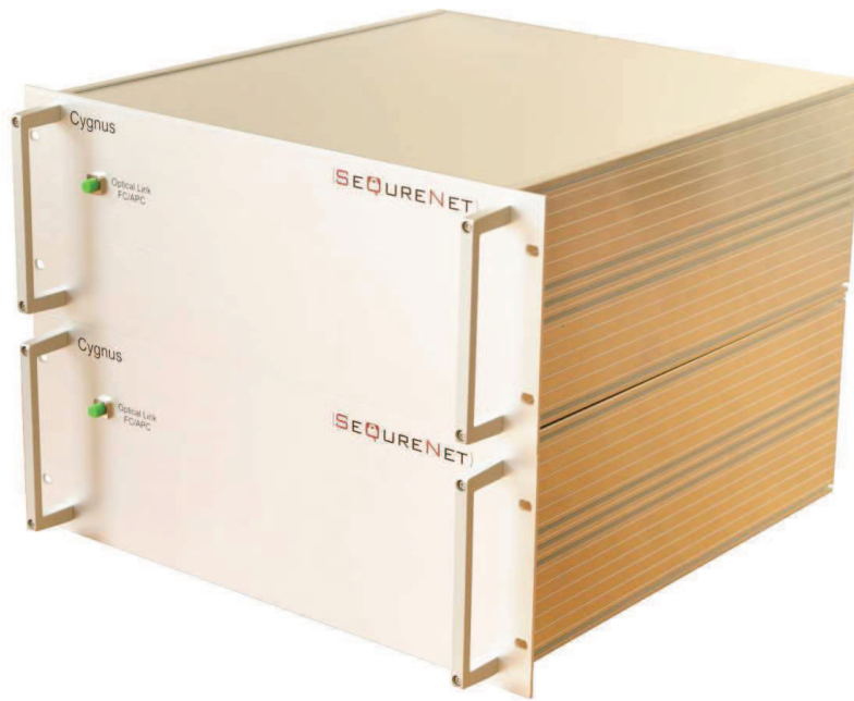
Figure 1: Cygnus: a quantum key distribution product commercialized by SeQureNet. The optical part is composed of two standard 19 inches rackable boxes of 4U, one for Alice and the other for Bob. They are driven by two computers that also perform the different post-processing steps.
