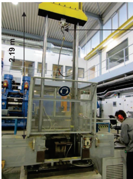
Figure II-3: Battelle drop weight tear test equipment
