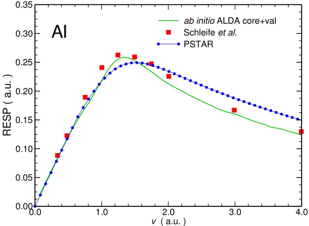
Figure 7.7: RESP of Al within ALDA in linear-response (solid green line) compared to the time-propagation results of Schleife and coauthors.[77] Experiment from the PSTAR database[7] (blue circle symbols) is given as a reference.
