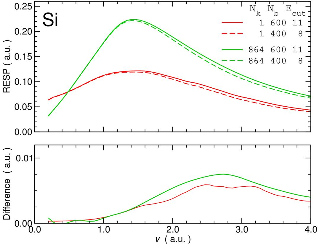
Figure 6.6: Comparison of the convergence rate for 2  $\mathbf{k}$ -point meshes:  $\Gamma$  (red lines) and 864 BZ points (green lines). The upper panel shows the RESP for two levels of convergence, whereas the lower panel shows their difference.
