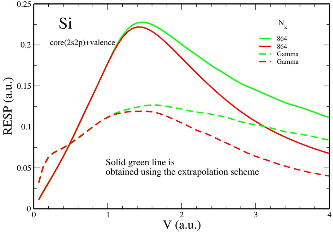
Figure 6.10: The fully Converged RESP of (2s2p3s3p) electrons in Si target for proton ( $Z_1=1$ ) within the linear response of RPA calculated by extrapolation scheme in Eq. (6.5). The green line obtained for highly converged parameters (2500 bands and  $E_{cut} = 35$  Ha) for the all electrons (without 1s), the red line obtained for low converged parameters (400 bands and  $E_{cut} = 8$  Ha) for valence only.
