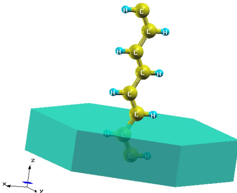
Figure 8.5: View of single isolated PA chain along the z-axis. The length of C=C bond is  $1.34 \text{ \AA}$  which is found in each unit  $\text{C}_2\text{H}_2$ , and the C-C bond length is  $1.451 \text{ \AA}$ .
