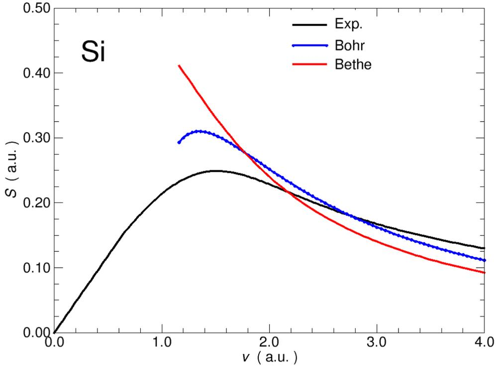
Figure 2.1: Electronic stopping power as a function of the projectile velocity calculated using both Bohr’s formula (blue line) and Bethe’s formula (red line). Experiment from the PSTAR database [7] (black line) is given as a reference.
