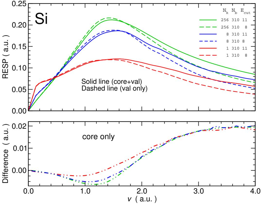
Figure 6.7: Comparison of the RESP core contribution calculated using 3  $\mathbf{k}$ -point meshes: 256 BZ points (green lines), 8 BZ points (blue lines) and  $\Gamma$  (red lines). The upper panel shows the RESP for two levels of electrons contribution, i.e., the 2s2p3s3p electrons and 3s3p electrons only whereas the lower panel shows their difference, i.e., the 2s2p electrons only).
