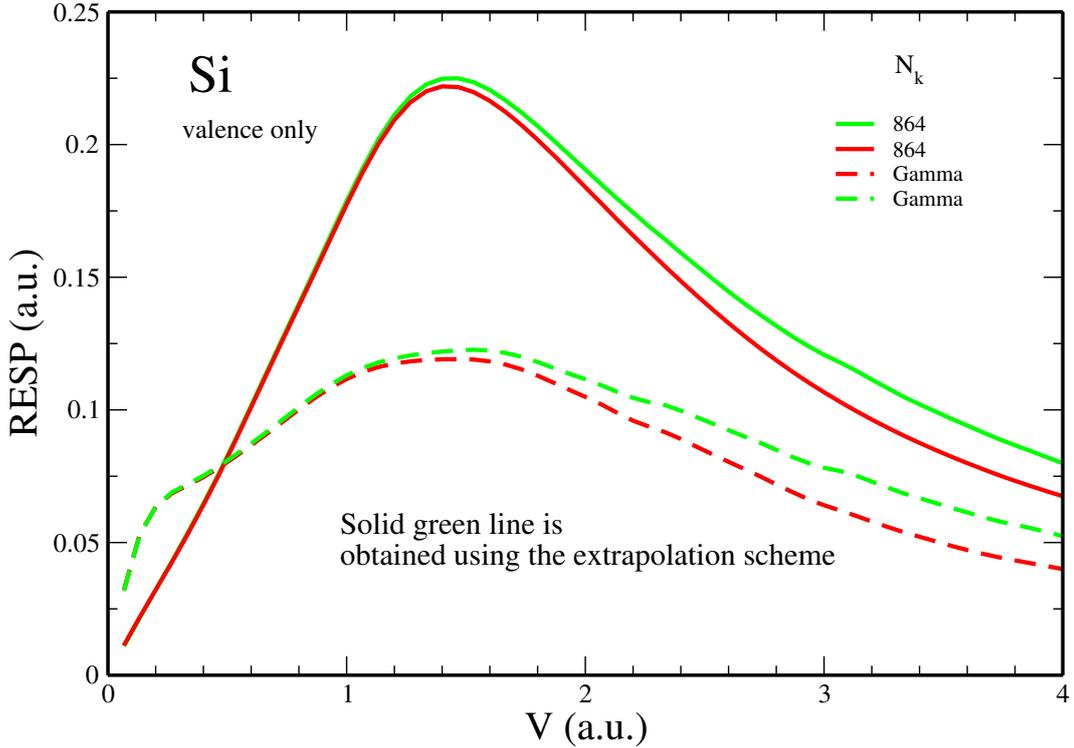
Figure 6.8: The fully Converged RESP of valence electrons in Si target for proton ( $Z_1=1$ ) within the linear response of RPA calculated by extrapolation scheme in Eq. (6.4). The green line obtained for highly converged parameters (2000 bands and  $E_{cut} = 25$  Ha), the red line obtained for low converged parameters (400 bands and  $E_{cut} = 8$  Ha).
