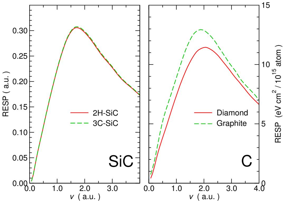
Figure 7.10: RESP of SiC (left-hand panel) and of carbon (right-hand panel) within ALDA including the  $2s2p$  electrons of Si. 3C-SiC and 2H-SiC phases are shown for silicon carbide, whereas graphite and diamond phases are shown for carbon.
