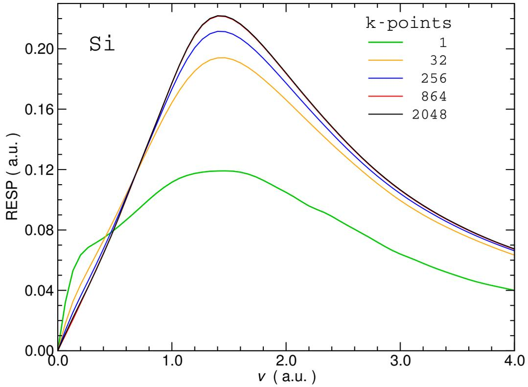
Figure 6.4: Convergence of the RESP of silicon within RPA as a function of  $\mathbf{k}$ -points. The convergence with respect to the  $\mathbf{k}$ -point grid was evaluated for a fixed number of bands (400) and a fixed dielectric matrix cutoff (8 Ha).
