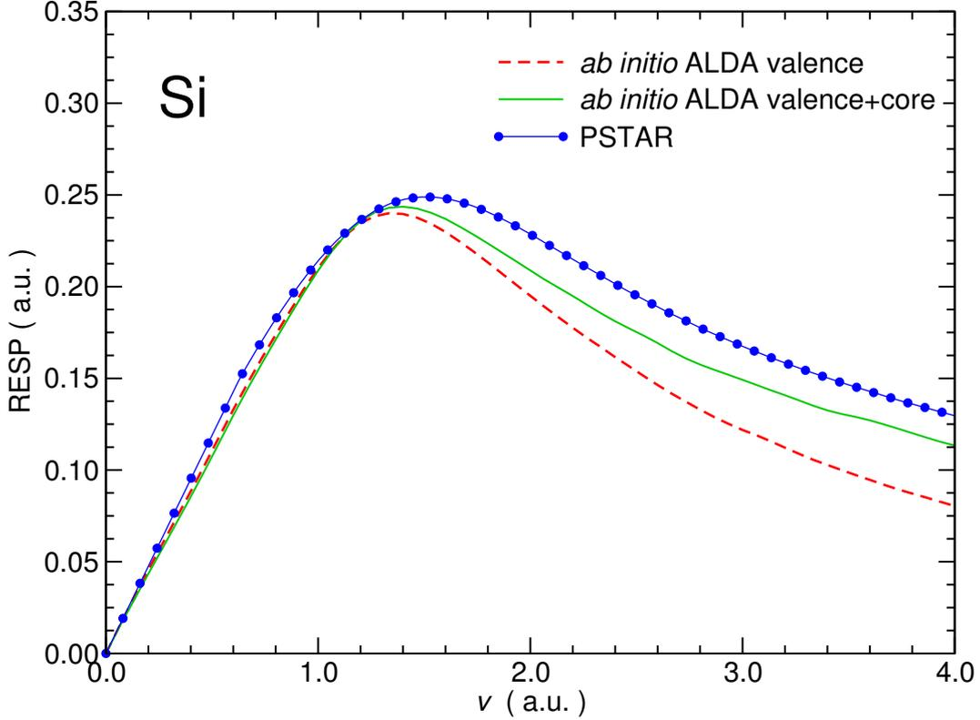
Figure 7.4: RESP of Si within ALDA including (solid green line) or not (dashed red line) the contribution from the core  $2s$  and  $2p$  electrons. Experiment from the PSTAR database[7] (blue circle symbols) is given as a reference.
