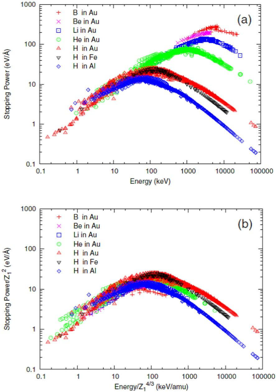
Figure 2.2: A demonstration of how simple scaling relationships (b) can capture much of the behaviour of the electronic stopping power (a) for a variety of projectile and target combinations. The scaling of stopping power by  $1/Z_1^2$  is informed by the prefactor in the fast particle stopping theories [79], [27] and [53] and the normalization of the particle velocity by  $1/Z_1^{2/3}$  is suggested by the Thomas-Fermi scaling of electronic velocities. Data are from the database of Paul[58]
