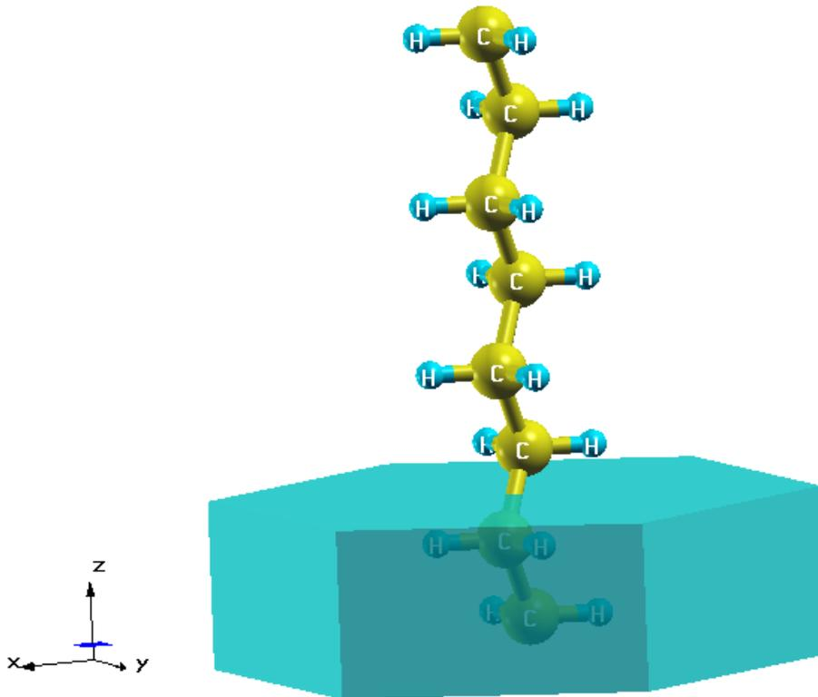
Figure 8.6: View of single isolated PA chain along the  $z$ -axis. The length of single bond ( $c$ - $c$ ) is  $1.535 \text{ \AA}$ .
