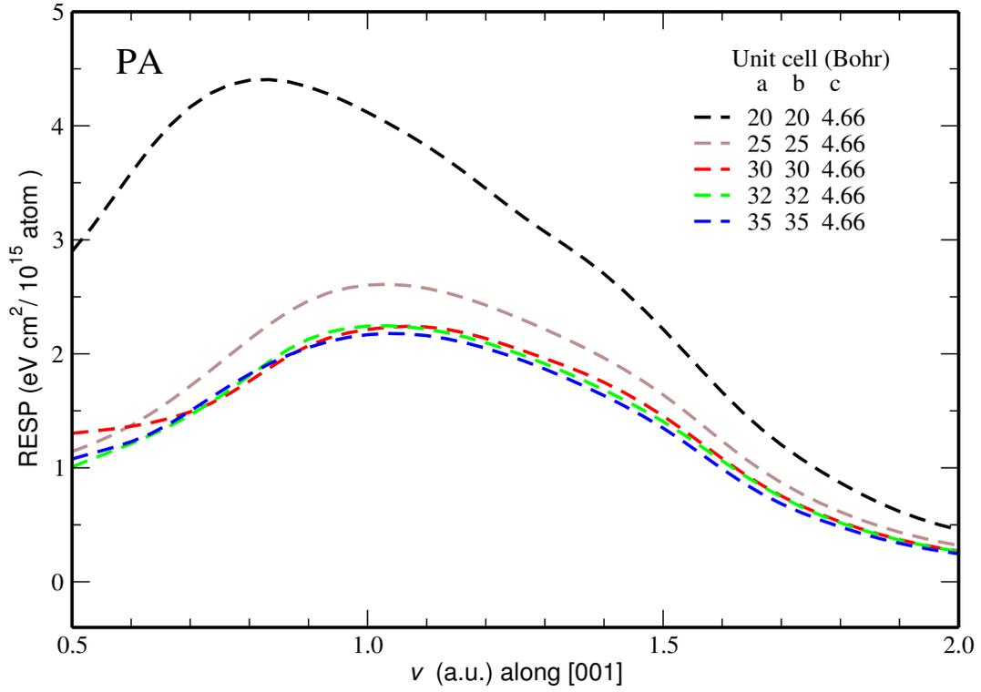
Figure 8.7: Volume convergence test of PA. RESP of proton in the PA target as a function of the cell volume  $V_c$  (The cell is orthorhombic P type). For all  $V_c$  the following parameters have been used:  $N_k = 1$  the gamma point,  $E_{cut} = 8$  Ha for  $\epsilon_{\mathbf{G}\mathbf{G}'}^{-1}(\mathbf{q}, \omega)$ ,  $\eta = 6$  eV and using  $\Delta E_{band} = 68$  eV energy band. The same excitation density is used for the all  $V_c$ .
