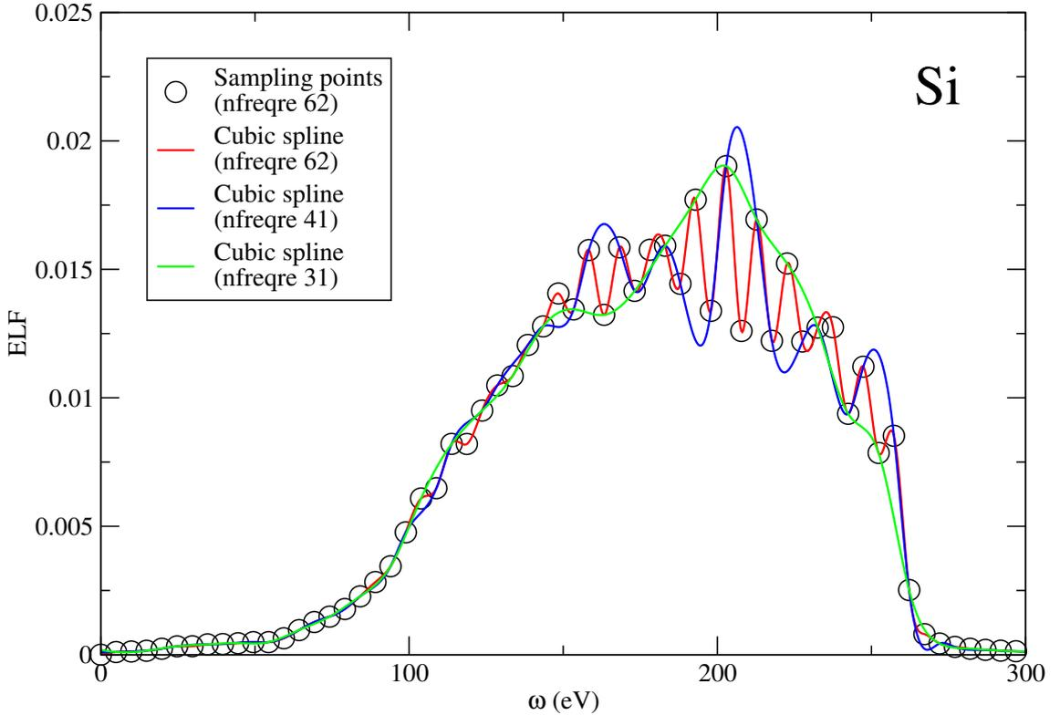
Figure 6.2: The accuracy of using the cubic spline interpolation with increasing the `nfreqre`. All the calculated values are obtained at  $|\mathbf{q} + \mathbf{G}| = 3.71$  a.u. along  $[111]$ . This study have been done using the following parameters:  $4 \times 4 \times 4$  with 4 shifts of  $\mathbf{q}$  point mesh, 400 bands and the broadening  $\eta$  is 1.5 eV.
