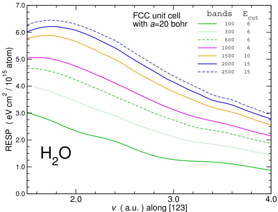
Figure 8.4: Convergence of the RESP of  $H_2O$  gas target within ALDA as a function of the number of bands and of the dielectric matrix cutoff. The convergence with respect to the number of bands and dielectric matrix cutoff was obtained for a fixed  $\Gamma$ -point sampling with  $\eta = 4$  eV. The convergence study is obtained for the all electrons (without 1s state of the oxygen atom).
