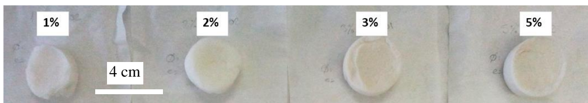
Figure VI.3: Visual aspect of CR aeropectins from different pectin initial concentrations in wt%.
