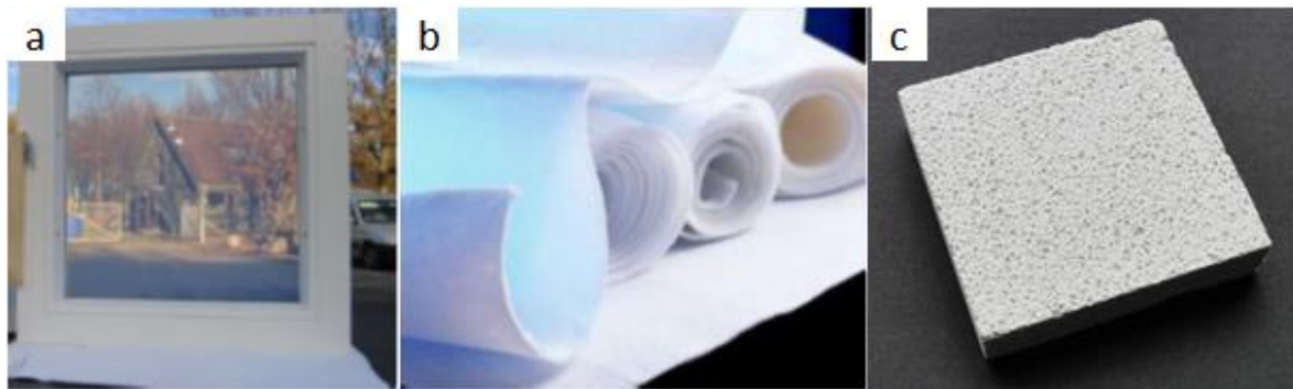
Figure I.25: Silica aerogel-based superinsulation materials aimed at various potential applications in the building domain. (a) Transparent aerogel glazing panel developed in the frame of the HILIT+ European project; (b) Aerogels blankets (here from the company Aspen Aerogels). (c) Render with dispersed aerogel granules developed by EMPA (Switzerland) and Fixit. Pictures taken from (Koebel et al., 2011 and Baetens et al., 2011), reproduced with permission from Springer and Elsevier respectively.
