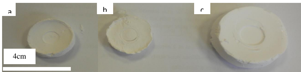
Figure V.13: Visual aspect of (a) tritylcellulose xerogel dried at 20°C ; (b) tritylcellulose xerogel dried at 60°C and (c) aerotritylcellulose dried in SC CO 2
