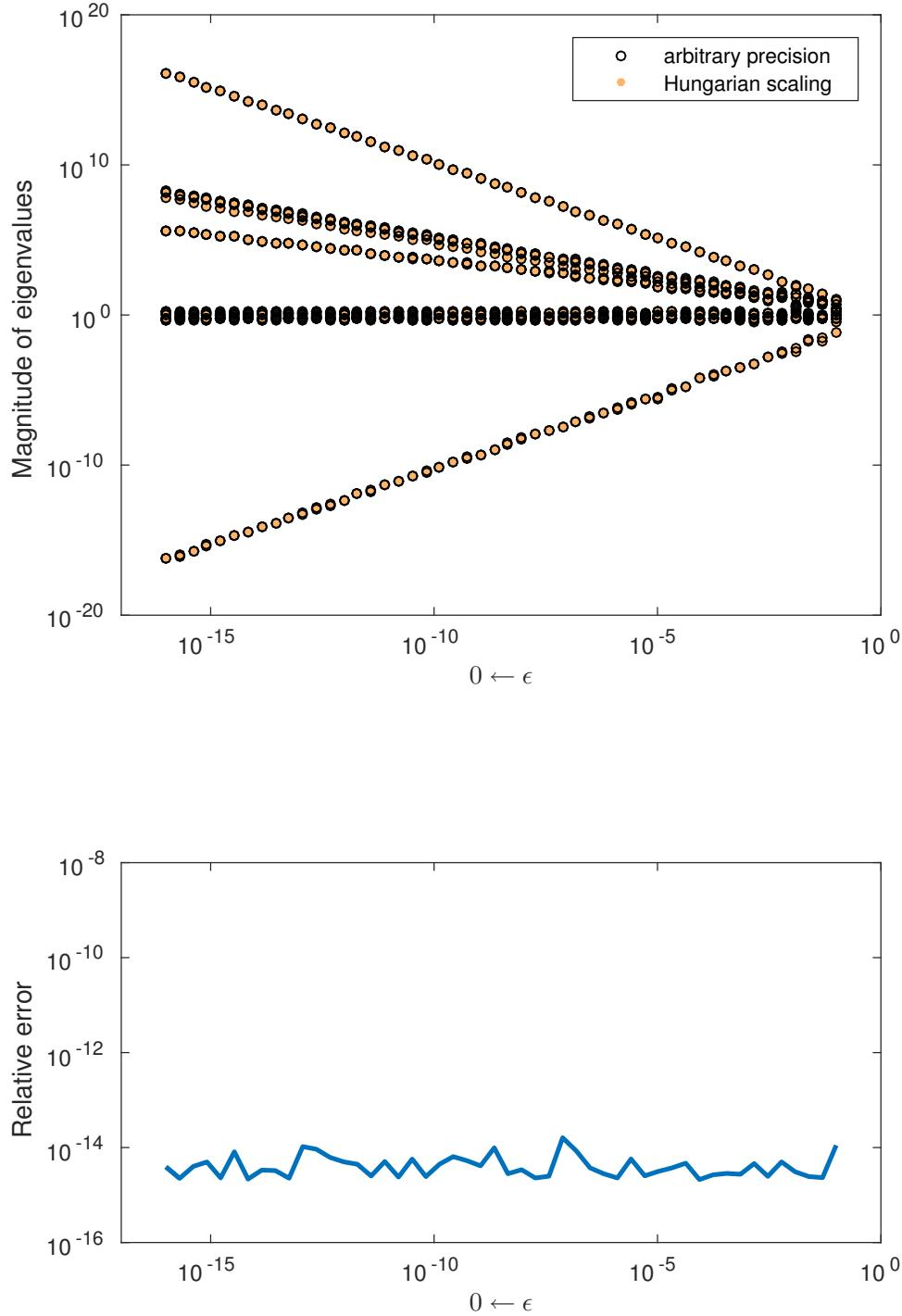
Figure 4.3: Comparison between the moduli of the true eigenvalues of (4.34) and the moduli of the eigenvalues obtained with `polyeig` after performing a diagonal scaling. Here the correspondence between true and computed eigenvalues is much better. The second graph shows, for each value of  $\epsilon$ , the largest relative error among the  $nd$  computed eigenvalues.
