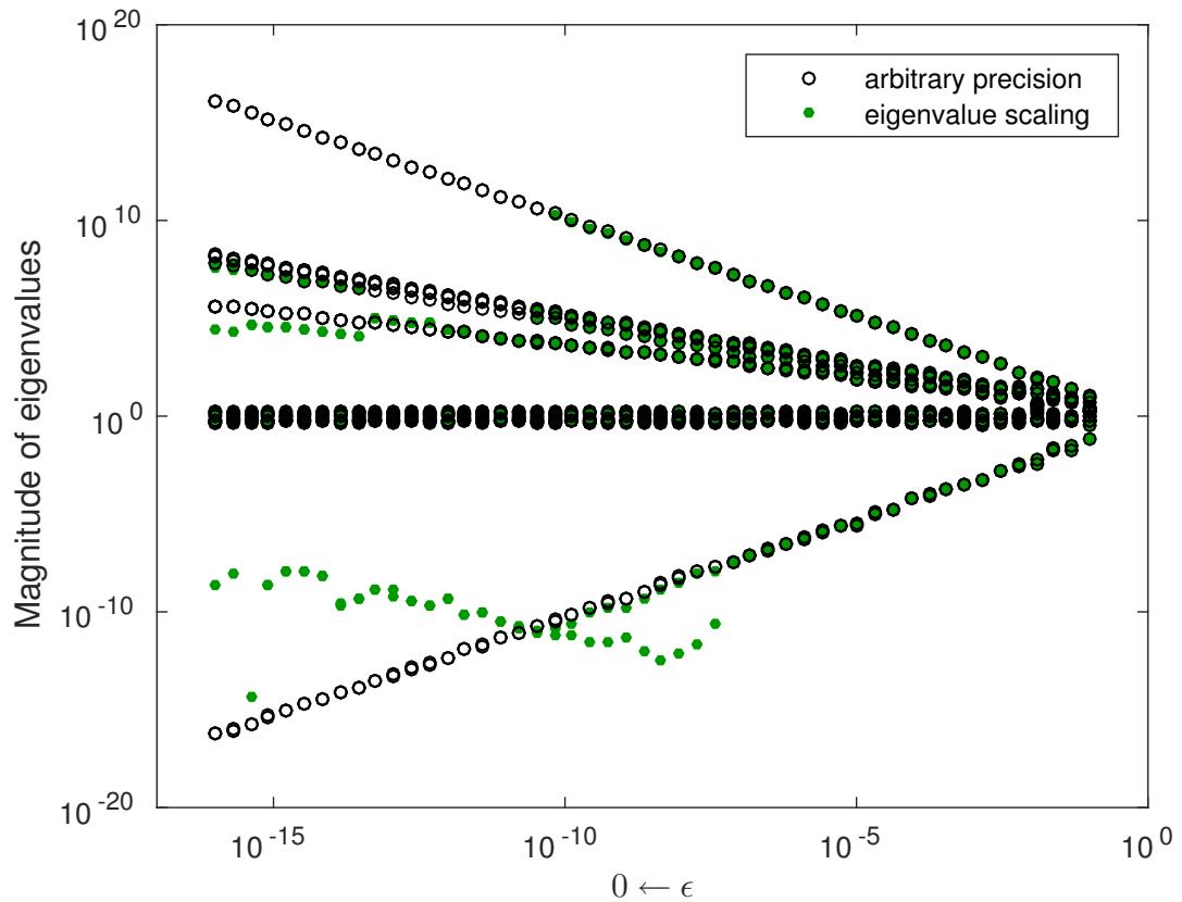
Figure 4.2: Comparison between the moduli of the true eigenvalues of (4.34) and the moduli of the eigenvalues obtained with `polyeig` after performing an “eigenvalue scaling”. The resulting figure is less chaotic than the previous one, but still far from satisfying, as approaching zero some spurious eigenvalues appear, while some other ones are computed as infinite by `polyeig` (and thus they are not plotted).
