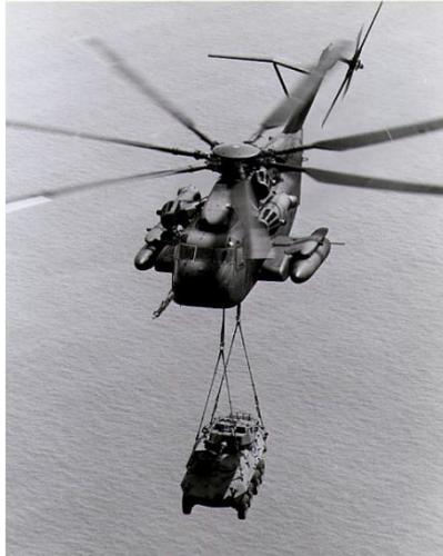
**Figure 3-2. Sikorsky CH-53E Super Stallion with external slung load**
