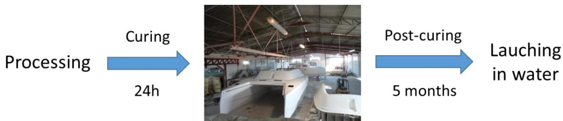
Figure III-IX Curing and post-curing steps of boat hulls before launching in water.
