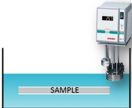
Figure II-VII Hydrothermal ageing water bath equipped with a thermostat.
