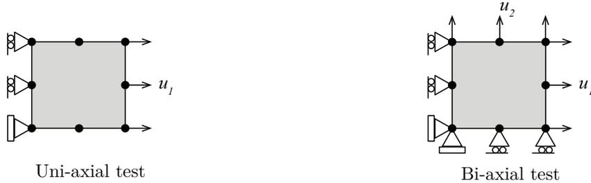
Figure 4.6: Configurations used for the single element tests in multisurface plasticity.
