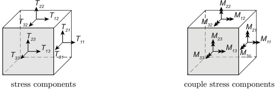
Figure 2.1: Stresses and couple stresses of a 3D Cosserat continuum. Stresses (left) are represented by polar vectors. Couple stresses (right) are represented by spin vectors.
