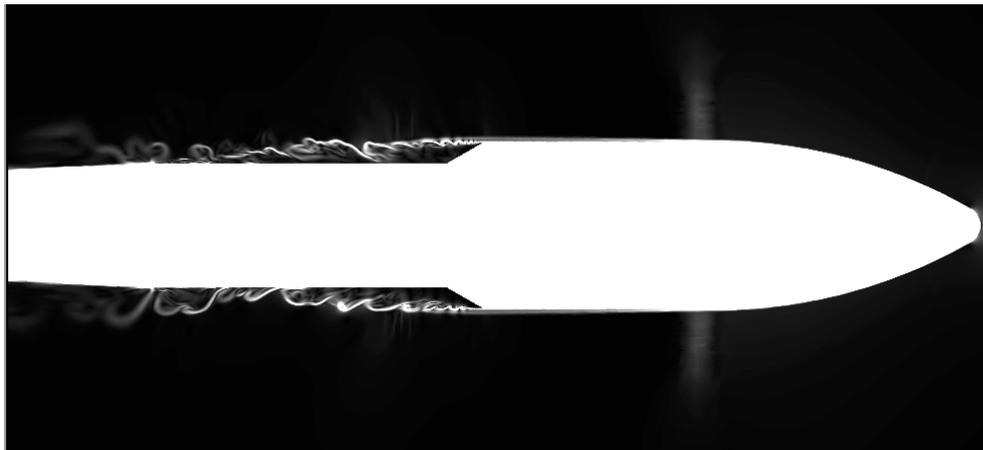
Figure 3.4: Instantaneous schlieren over a launcher shrinkage
