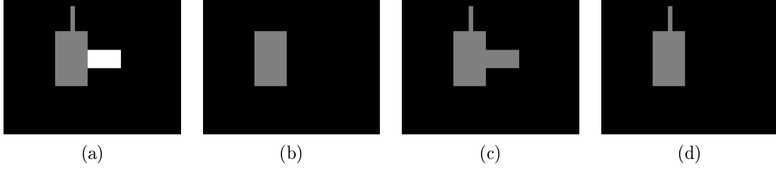
Figure 3.6.: Geodesic reconstruction of a 3-ary image: (a) reference image R , (b) marker image M , (c) classical grey-scale reconstruction, (d) n -ary reconstruction \gamma^{\text{rec}}(R; M) .
