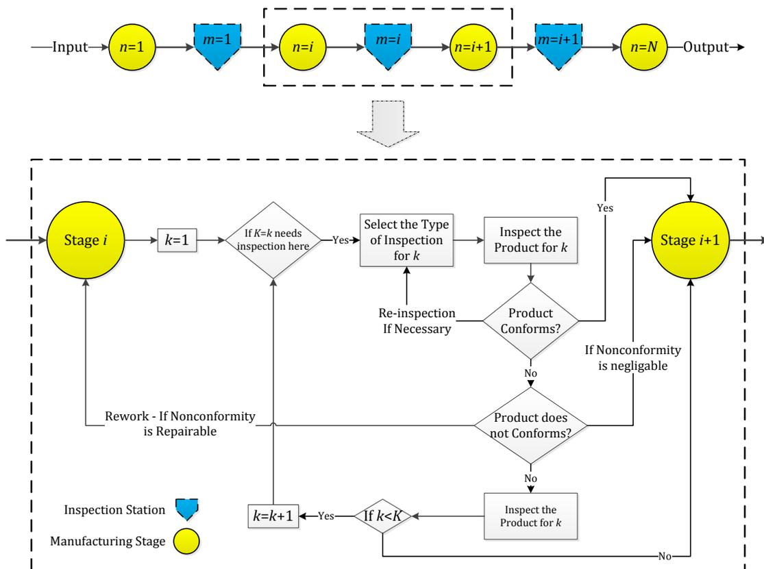
**Figure 1.1.** Inspection planning problem in a MPS
