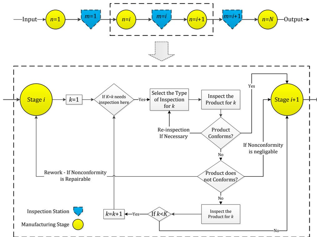
Figure 2. Inspection planning problem in a MPS
