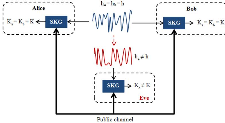
Figure 2-7: SKG in the presence of an eavesdropper.
