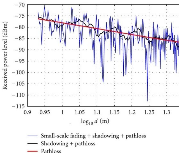
Figure 2-4: Path loss, shadowing and small scale fading.
