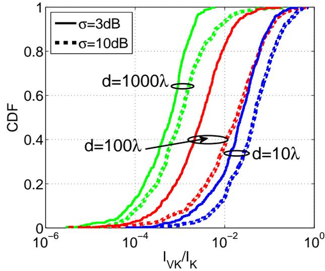
Figure 4-6: CDF of relative vulnerable key bits.
