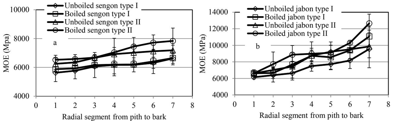
Figure 28 MOE values of LVL from pith to bark made of unboiled and boiled sengon (a) and jabon (b)
