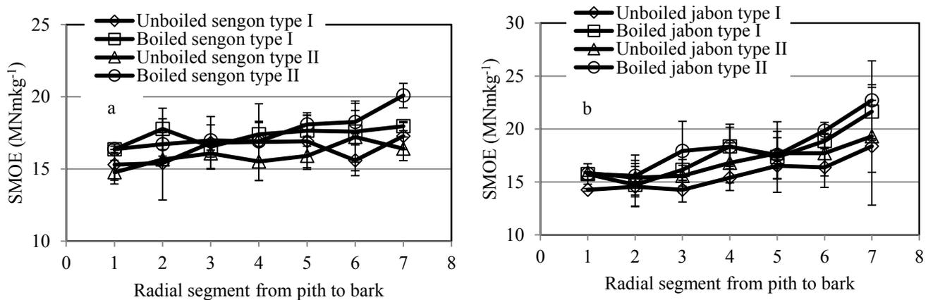
Figure 29 SMOE values of LVL from pith to bark made of unboiled and boiled sengon (a) and jabon (b)
