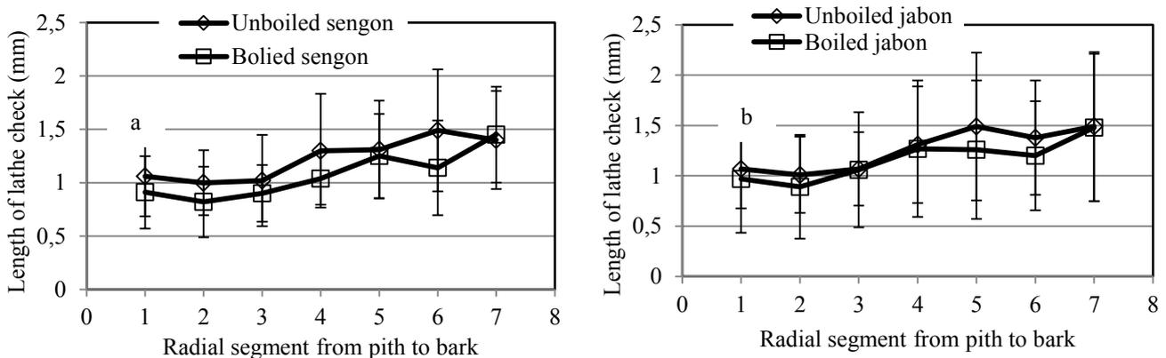
Figure 16 The progress of length of lathe check from pith to bark of sengon (a) and jabon (b) veneers
