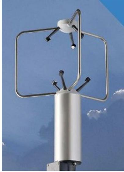
Figure 2.5 – 3D ultrasonic anemometer
