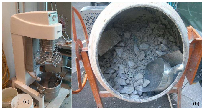
Figure III.4. (a) ITL soil fines mixing; (b) Ballast + gravel + fines mixer
