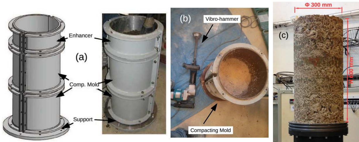
Figure III.14. (a) Scheme of parts constituting the compaction mould; (b) sample being compacted with a vibro- hammer; (c) view of a compacted sample after remoulding
