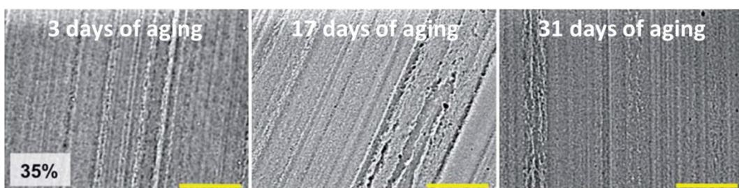
**Figure 18** Micrographs of aged PVA hydrogels (35 wt% of PVA). Scale bar is 80  $\mu\text{m}$ .<sup>44</sup>
