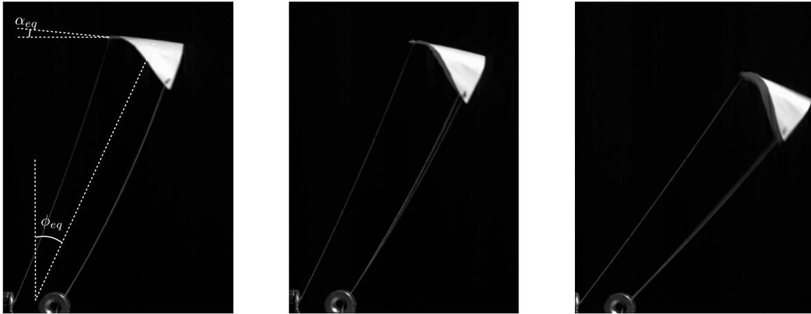
(a)  $L_g = 0.121 \text{ mm}$  et  $\alpha_{eq} = 7^\circ$     (b)  $L_g = 0.118 \text{ mm}$  et  $\alpha_{eq} = 13^\circ$     (c)  $L_g = 0.115 \text{ mm}$  et  $\alpha_{eq} = 25^\circ$
