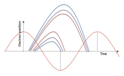
Figure 2.4: Representation of the electronic trajectories in the continuum as a function of the pulse cycle and the position of the electron on the atom
