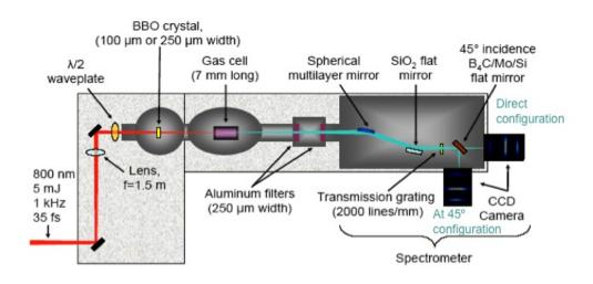
Figure 3.6: Proposed set-up to study the generation of harmonics in a two colour field. The introduction of a multilayer mirror at  $45^{\circ}$  is based on the proposition given by the  $\delta^3$  to study generation in this specific regime.
