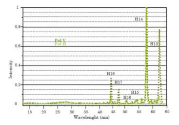
Figure 3.25: Experimental results. Spectre attained in direct configuration using a  $250\mu m$  thickness BBO. On light green the horizontal, p polarisation is represented and on darker green the vertical, s polarisation is shown.
