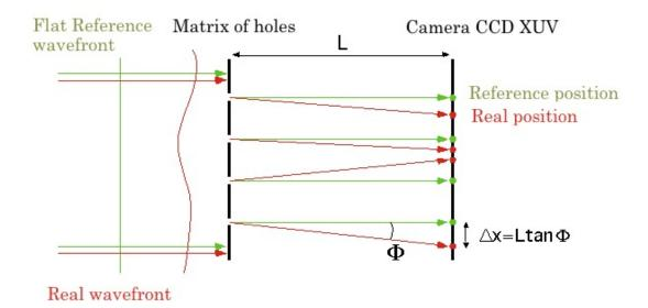
Figure 2.15: Wavefront principle of actuation
