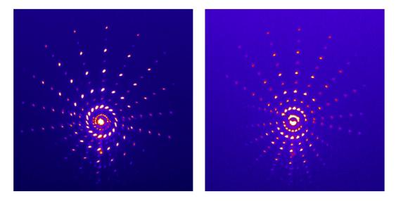
Figure 3.37: Acquired data for both BBO crystals. For the maximum generation approximately. The first image corresponds to the maximum generation of energy using the  $100\mu m$  thickness BBO. The second corresponds to the maximum generation of energy using the  $250\mu m$  thickness BBO.
