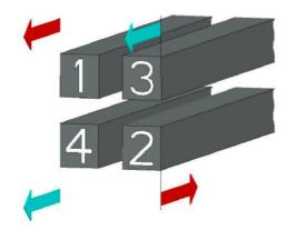
Figure 4.15: APPLE II undulator, schematic. Row 1 and 2 shift in opposite direction (dark arrows, anti-parallel shift, s1=-s2) which controls the inclination of the polarisation ellipse. Row 3 and 4 shift in the same direction (light arrows, parallel shift, s3=s4) which changes the ellipticity of the polarisation ellipse. [16]
