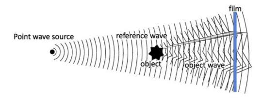
Figure 1.16: Principle of in-line Holography
