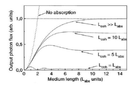
Figure 2.6: Number of photons of harmonics generated as a function of the length of the media for different lengths of coherence [6]
