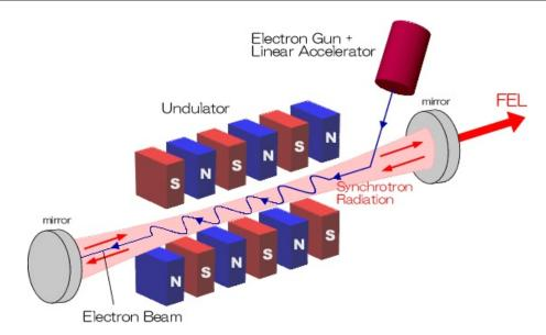
Figure 1.5: Free electron laser principle. As the electrons arrive the undulator they present an aleatory phase. The radiation emitted is incoherent. As the electrons interact with the radiation *bunching* occurs. The train waves emitted are now in phase and the radiation is amplified in a coherent
