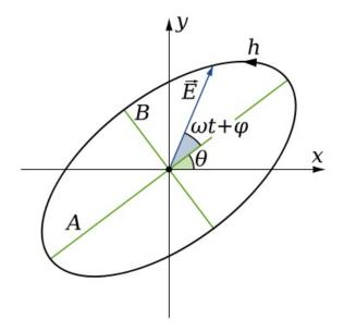
Figure 3.39: Representation of the elliptic polarisation scheme with the corresponding parameters.
