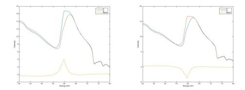
Figure 4.20: XMCD measurements on the Co(40nm)/Al(5nm)/SiN(50nm) sample. The angle of incidence was 30 degrees and the maximum signal can be seen at 60 eV as expected corresponding to the M-edge of Cobalt
