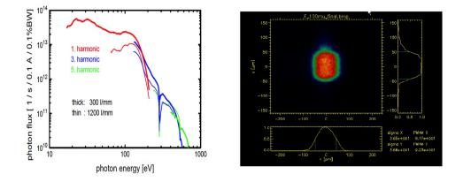
Figure 4.17: Source characteristics. Photon flux at UE112. Focal spot for 100 microns exit slit
