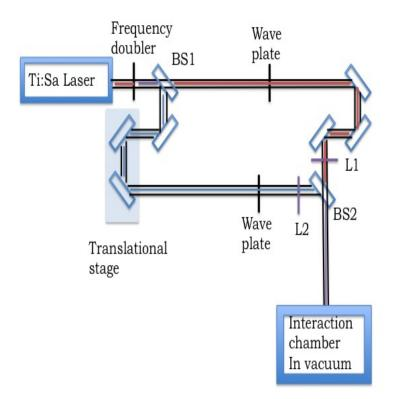
Figure 3.57: Example of a pump-probe experiment that can be used to adjust the delay between both fields and their relative intensity
