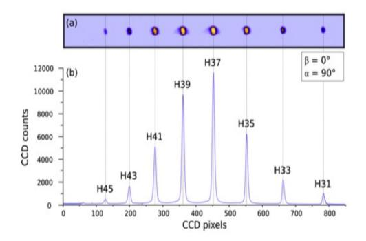
Figure 3.30: Experimental data: (a) Harmonic spectrum acquired on the CCD with the polariser for  $\alpha = 90^{\circ}$  and  $\beta = 90^{\circ}$ . Accumulation of 40000 thousand pulses. (b) Cross section of the image with the intensity of each harmonic shown and the distance in pixels between the grating and the CCD.
