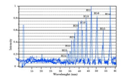
Figure 3.18: S polarisation High Harmonic odd and even spectre. The full line corresponds to the direct configuration and the dashed line to the  $45^{\circ}$  mirror configuration.
