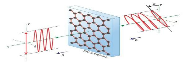
Figure 4.10: Scheme of a system showing Faraday rotation.
