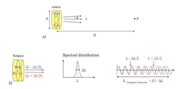
Figure 1.2: Coherence of a beam a) Spatial coherence scheme. Two distinct points taken from a beam cross section at the same instant will emit two fields that are correlated. b) Temporal coherence scheme. One point taken from a beam cross section at two different instants will emit two fields that are correlated. The temporal coherence length is the given by the propagation distance at which the two waves will show opposite phases.
