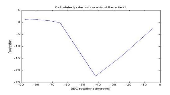
Figure 3.55: Calculated polarisation of the  $\omega$  axis, fundamental field as a function of the 100 $\mu$ m thickness BBO crystal.
