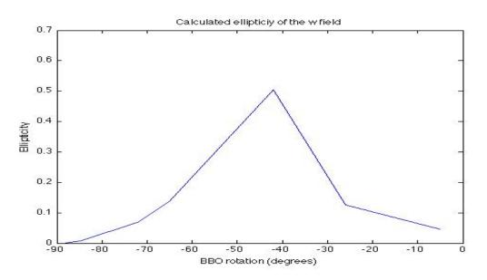
Figure 3.53: Calculated ellipticity of the fundamental field as a function of the  $100\mu m$  thickness BBO crystal.
