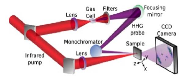
Figure 5.3: Pump probe setup. An intense IR laser pulse is split by a beam splitter resulting on a pump beam and a probe beam. The probe beam is focused by a lens onto a gas cell resulting in high harmonic generation. The IR is filtered and the remaining beam is reflected on a focusing mirror onto a monochromator onto the sample. The pump is directed onto the sample and focused by means of a lens. A CCD camera records the data.
