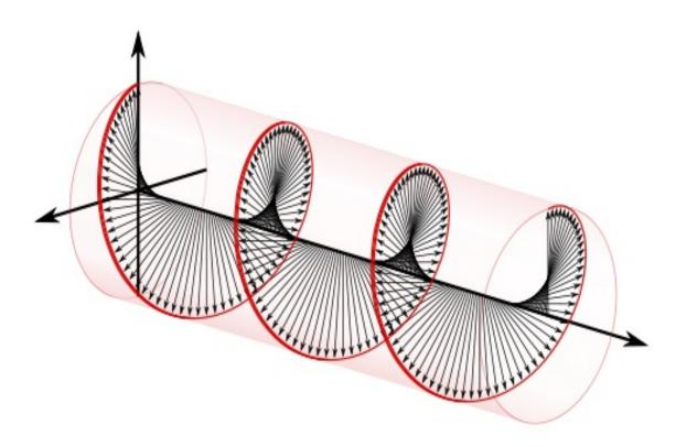
Figure 4.2: Scheme of circular polarised light. [13]
