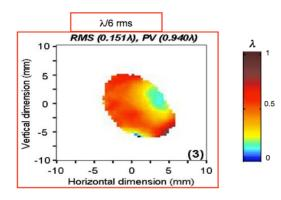
Figure 2.16: Wavefront measurement of an harmonic beam at salle orange In this case we are in the presence of a flat spectrum that is a spectrum having
