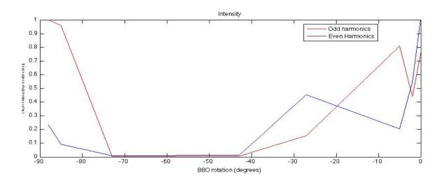
Figure 3.52: Normalised intensity of the even and odd harmonics as a function of the  $100\mu m$  thickness BBO crystal.
