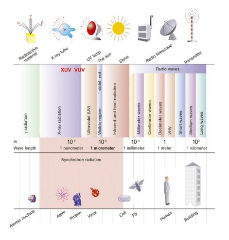
Figure 1.1: Electromagnetic spectra illustrated with sources for the radiation, its wavelenght and its penetration power from *Radio waves*; lower energy to *Gama radiation*; higher energetic.
