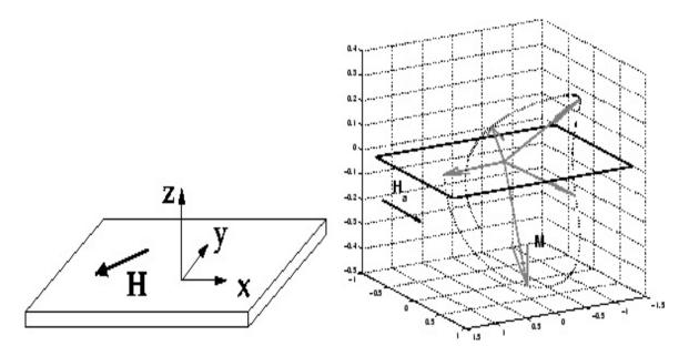
Figure 4.7: Example of precessional motion of magnetisation. [14]
