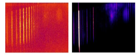
Figure 3.23: High harmonic (odd and even) signal registered on the CCD using a  $100\mu m$  thickness BBO. Using a  $250\mu m$  thickness BBO. The presented intensities on both images are different on order for the spectre to be apparent.
