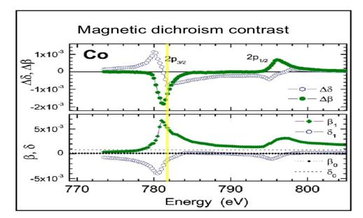
Figure 4.13: L-edge for Cobalt measured at BESSY [12]
