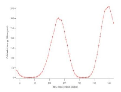
Figure 3.33: Measured BBO crystal generation of second harmonic in joules.
