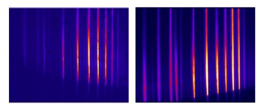
Figure 3.14: High harmonic signal registered on the CCD by varying the positioning of the mirror. On the left it is represented the obtained HHG signal at a direct configuration. On the right it is represented the obtained HHG signal at a configuration of  $45^{\circ}$ .
