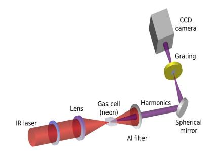
Figure 1.8: Scheme of the principle of installation of an High Harmonic Generation (HHG) line using Neon at *salle orange*
