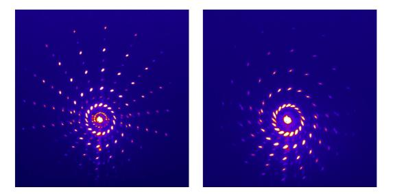
Figure 3.35: Data acquired with an  $100\mu m$  thickness BBO for a) the maximum generation of second harmonic and b) for the minimum generation of second harmonic. The images were acquired for different rotating stages of the BBO crystal.
