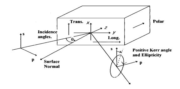
Figure 4.9: Schematic of MOKE geometry. [15]
