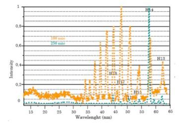
Figure 3.24: Experimental results for the influence of the BBO on the generation on the direct configuration. A  $100\mu m$  thickness BBO resulting spectrum is represented in orange and a  $250\mu m$  thickness BBO spectra is represented in blue.
