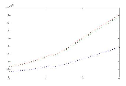
Figure 4.19: Calibration of the system for the different radiation polarisations, Linear (blue), circular positive (red), circular negative (green)
