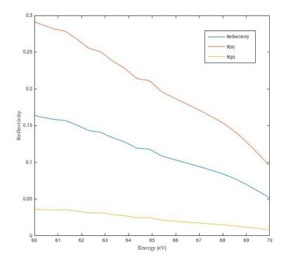
Figure 3.27: Multilayer theoretical reflectivity: Simulated reflectivity for the multilayer used (*IMD*)
