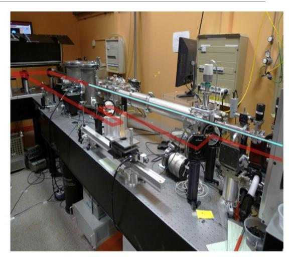
Figure 5.4: Image of pump-probe set-up at salle orange. The intense IR beam is split in two at the beginning of the table. The non covered beam is the pump and the probe will be in vacuum. When the probe beam crosses the first chamber containing the gas cell harmonics are generated here portrayed in light blue. The IR will be filtered by a metallic filter and the probe will be mainly XUV radiation.
