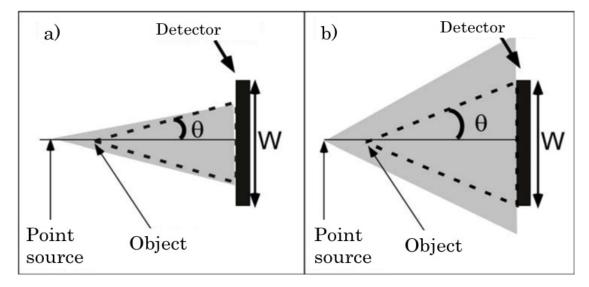
Figure 1.18: Numerical aperture defined by a) the divergence of the source and b) by the detector
