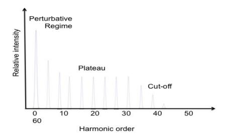
Figure 2.2: Typical High-Harmonic spectrum where the three zones: *Perturbative regime, Plateau* and *Cut-off,* are identified.
