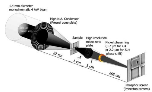
Figure 1.11: Example of a X-ray microscopy set-up. A zone plate focuses the monochomatised undulator beam onto the object and a micro zone plate objective forms a magnified image on a CCD camera. The phase ring selectively shifts the undiffracted light of the object.
