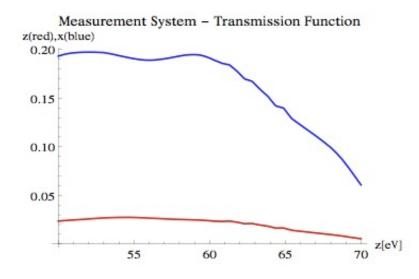
Figure 3.28: Multilayer theoretical reflectivity: Transmission function of the set-up in function of the energy for s (blue line) and p (red line) polarisation of light
