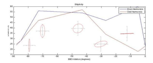
Figure 3.54: Ellipticity of the even (blue) and odd (red) harmonics in function of the BBO rotation. The inlets show the calculated polarisations of the fundamental field as a function of the  $100\mu m$  thickness BBO crystal.
