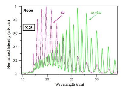
Figure 2.10: High harmonic spectra attained for a single colour field and a twocolour field laser pulse. The conversion efficiency is 25 times higher for Neon in these conditions. It is clear the effect of the doubling of the fundamental frequency: Odd and even harmonics appear. The red shift is also present.
