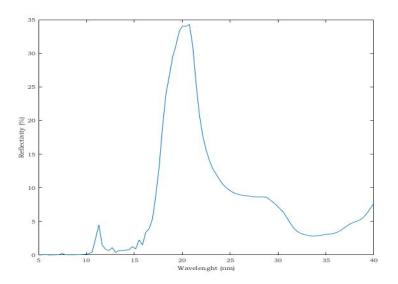
Figure 3.8: Multilayer theoretical reflectivity: Mirror reflectivity as a function of the wavelength. The mirror is set at  $45^0$  of incidence.
