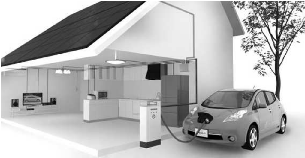
Figure 1.8: Vehicle-to-Home concept from Nissan motor corporation.
