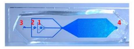
Figure 1 - Droplet-based microfluidic system.
