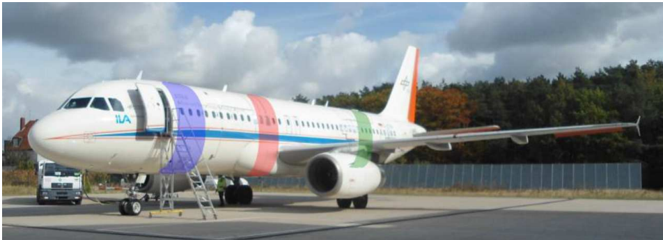
Figure 4.20 – ATRA aircraft from the DLR. The colors indicate the areas where measurements of panels accelerations have been performed: front cabin (blue), mid cabin (red) and aft cabin (green) - after Klabes et al. (2015).
