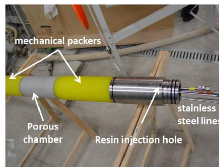
Fig. 1. 14. Measurement chamber of a PP system (from Armand et al. 2015b)
