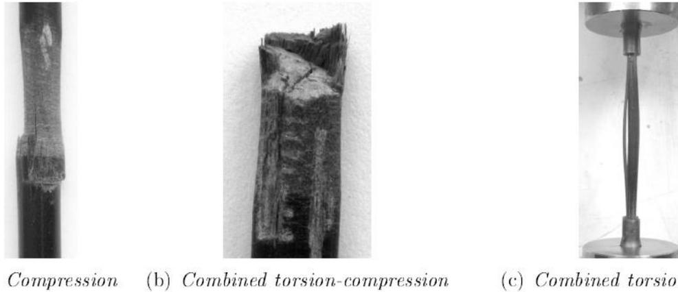
*Figure 1.17: Static rupture modes for a) compression, b) combined torsion-compression, c) combined torsion-traction. Kotelnikova-Weiler [2012]*
