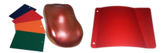
Figure 1.1: Several types of physical samples for automobile paints.
