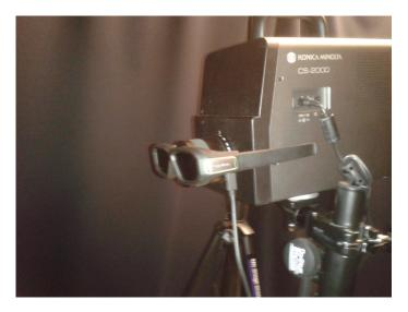
Figure 3.19: Stereoscopic characterization with a spectrometer and the Nvidia 3D shutter glasses.
