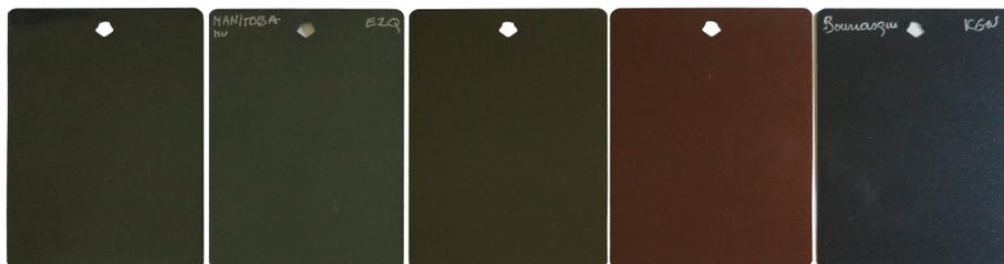
Figure 4.13: Paint samples. From left to right: GM1, GM2, HI, BC and BR. The first three samples possess an overall green tint —HI being slightly brownish—, whereas BC and BR have a red and blue tint respectively. All samples are shiny except for GM2, which is matte.
