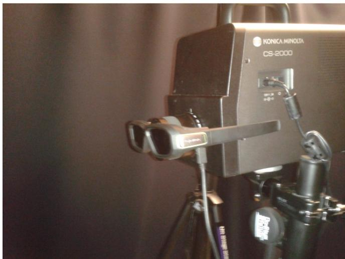
Figure 3.19: Stereoscopic characterization with a spectrometer and the Nvidia 3D shutter glasses.
