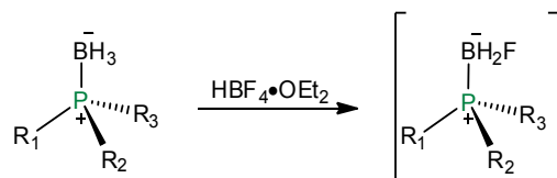
Scheme 46: Decomplexation of phosphine boranes using \text{HBF}_4 \cdot \text{OEt}_2 . The reaction is reported to go through the formation of a phosphine fluoroborate intermediate. 214,237
