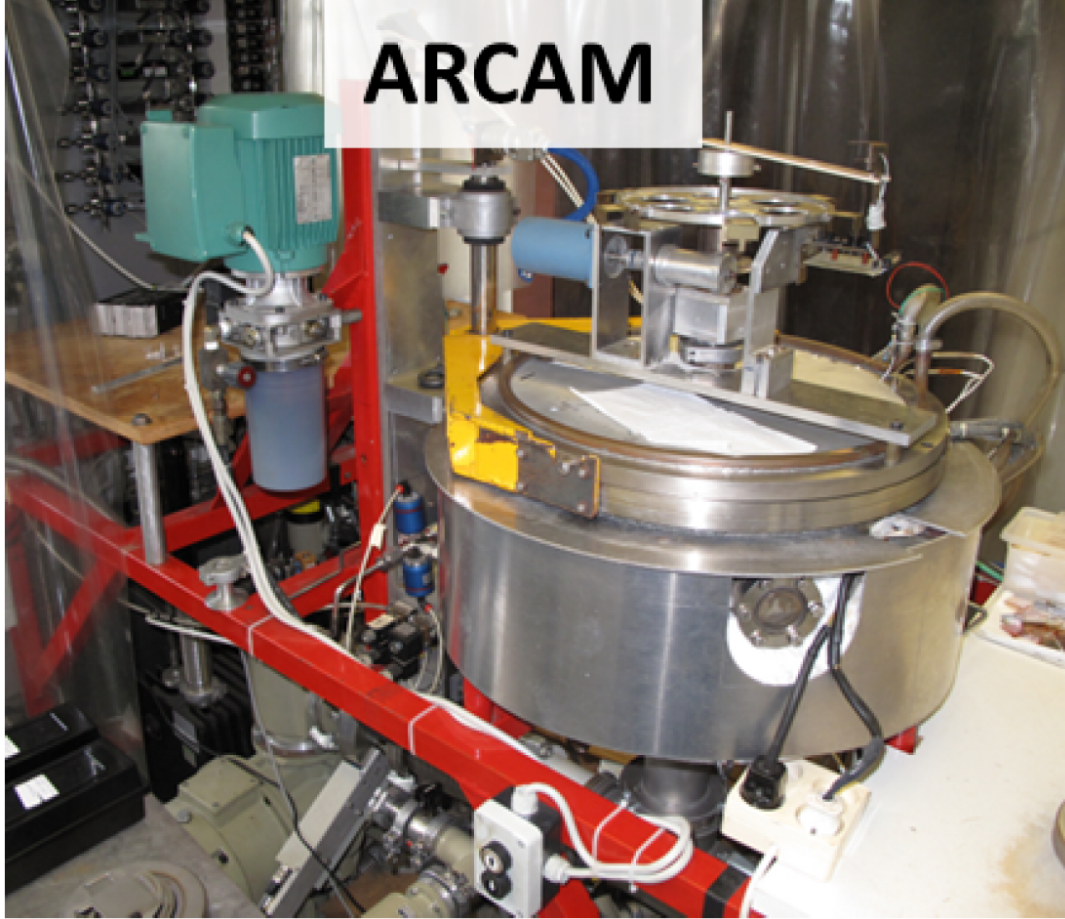
Figure 4.5 – Picture of the ARCAM multiplasma monochamber reactor in LPICM.
