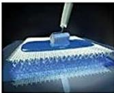
Evenly apply the remaining approximately 60 % of the recommended resin quantity over the fabric. The capillary forces in the Parabeam® 3D Glass Fabric will automatically impregnate the fabric. De-airing is not necessary since the layers are thin and air will escape on all sides.
