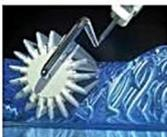
Gentle rolling of the top face of the fabric will secure a plain surface. For all fabrics up to 0.87 inches, the maximum height is achieved by finishing with gently rolling in weft direction against the pile direction.
