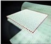
Calculate the Parabeam® 3D Glass Fabrics' weight for the surface area desired. Define resin quantity according to the fiber-resin ratio (see for resin consumption indicator overleaf). Precautions should be taken to avoid cure inhibition when using UP resins. A low styrene emission (LSE) type or alternatively the addition of a styrene emission reducer to the resin is recommended.
