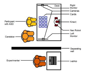
Figure 5.1: Setup of the Joint Attention task experiment
