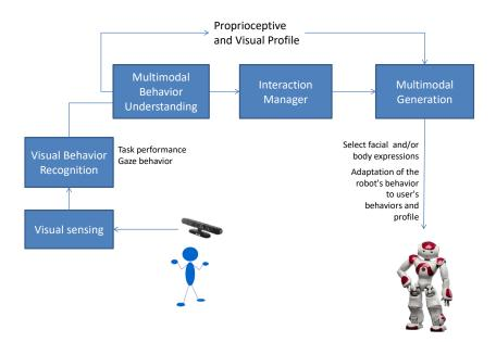
**Figure 7.1:** Proposed Framework. With this framework, the RGB-D data would enable the system to detect the profiles, the performance and the social behavior of the participants. With these, the system would modify the behavior of the robot accordingly to the participant's information.
