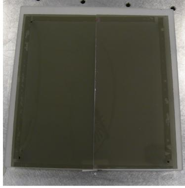
Figure 5.5: Polarization foil used for creating polarized illumination. It is attached with LED array in the experimental set up. Left rectangular portion of foil generates vertical polarized light while the right rectangular foil generates horizontal polarized light
