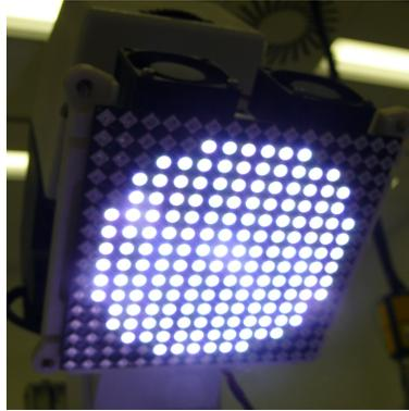
Figure 5.2: LED array illumination scheme. The optical condenser is replaced by a programmable LED array. The figure shows a circular illumination pattern.
