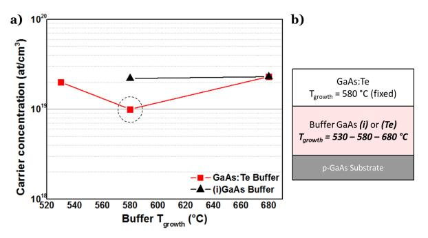
Figure 4.14 - Carrier concentration of the heavily doped GaAs:Te layer as a function of growth temperature of the previous buffer layer for three different buffers : Te-doped and intrinsic GaAs.
