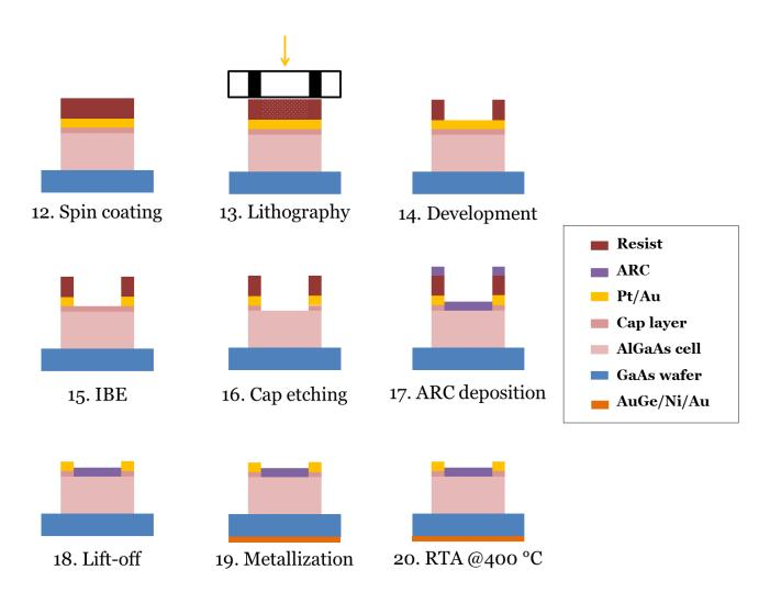
Figure 5.7 - Cross section schematics of the solar cell process flow: grid definition and ARC deposition
