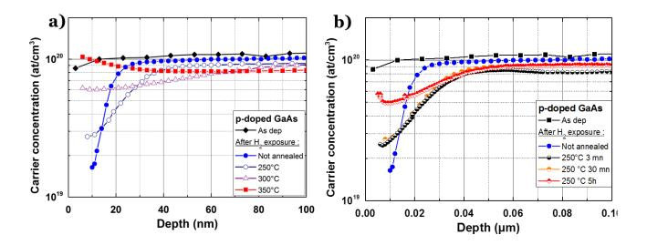
Figure 3.11 -ECV profiling of GaAs :C before H<sub>2</sub> exposure, after H<sub>2</sub> exposure and after a) 3-minutes annealing at various temperatures, b) annealing at 250 °C for various durations
