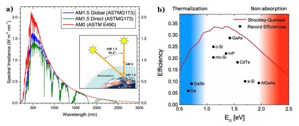
Figure 1.1 - a) Incident spectral irradiance from the sun for terrestrial applications (AM1.5G and AM1.5D) and space applications (AM0). b) Schockley-Queisser limit: maximum theoretical efficiency of a solar cell as a function of its bandgap, along with the best experimental efficiencies
