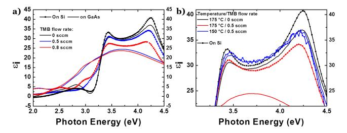
Figure 4.24 - a) Ellpisometric spectra of Si grown with TMB on Si substrate (squared) and on epi-GaAs (lines) with various TMB flow rates, b) Ellipsometric spectra on Si and epi-GaAs at various TMB flow rate and temperatures
