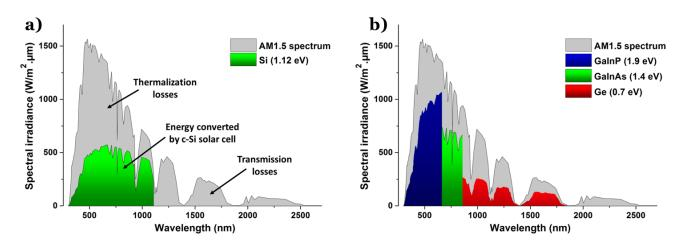
Figure 1.3- AM1.5G spectrum and the fraction theoretically converted by a) a Si solar cell, b) a triple junction GaInP/GaInAs/Ge (from ref<sup>9</sup>)
