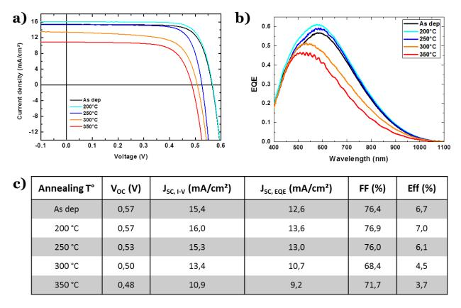
Figure 2.24 - a) J-V characteristics at low-temperature and b) external quantum efficiency of all the solar cells processed after various annealing temperatures, c) Solar cells characteristics calculated from I-V measurements and EQE
