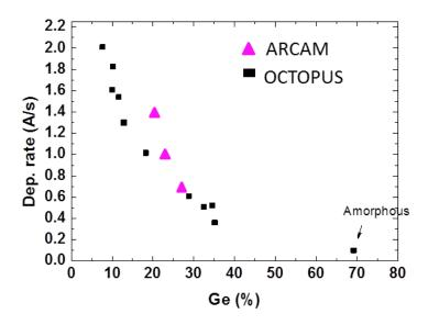
Figure 2.16 - Deposition rate as a function of Ge content for various calibration samples in Octopus reactor (squares) and Arcam reactor (triangle): Deposition rate strongly decreases with %Ge. Too high %Ge leads to amorphous growth.
