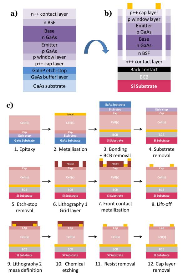
Figure 5.13 - Structure of a single GaAs (a) before and (b) after bonding an processing. c) Cross-section schematics of the process flow of inverted single or tandem solar cells
