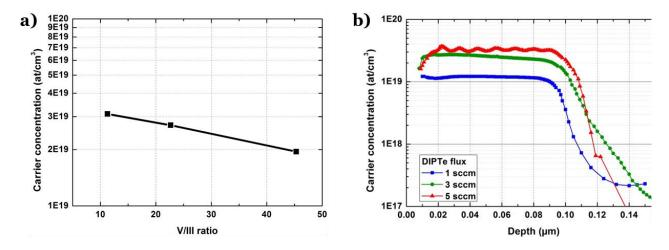
Figure 4.12 - a) Carrier concentration as a function of III/V ratio with fixed growth conditions of T = 580 °C, on an undoped GaAs buffer. b) ECV measurements for three different DIPTe flow rates
