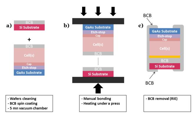
Figure 5.12- Schematics of the main technological steps of bonding with BCB
