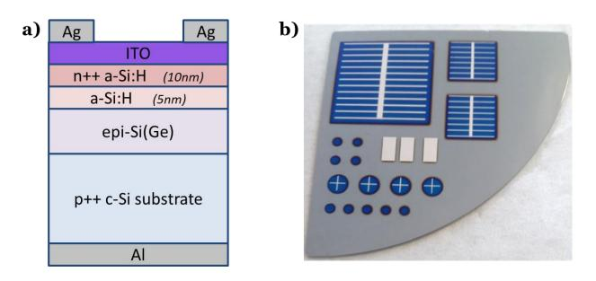
Figure 2.20 - a) Structure of the heterojunction solar cell grown and processed, b) top-view picture of the device after ITO deposition and metallization : one 2x2 cm<sup>2</sup> and two 1x1 cm<sup>2</sup> cells can be distinguished.
