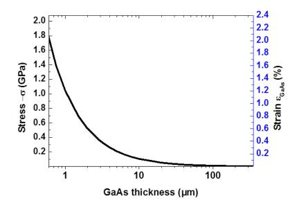
Figure 5.23 : Stress and strain in the III-V stack during GaAs substrate removal
