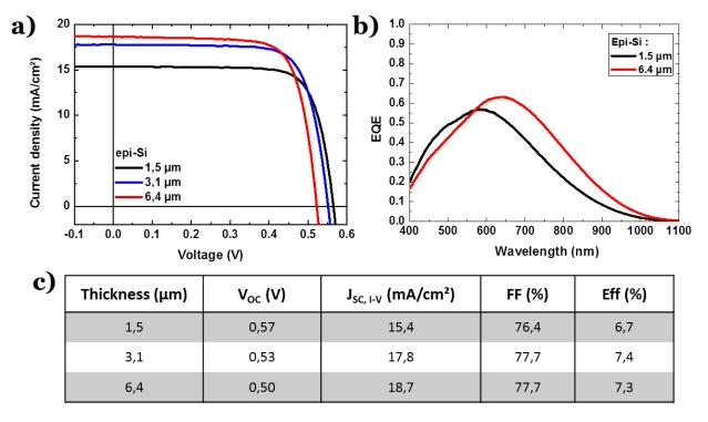
Figure 2.25 - J-V characteristics at low-temperature and b) external quantum efficiency of all the solar cells with various epitaxial thicknesses, c) solar cells characteristics calculated from J-V measurements
