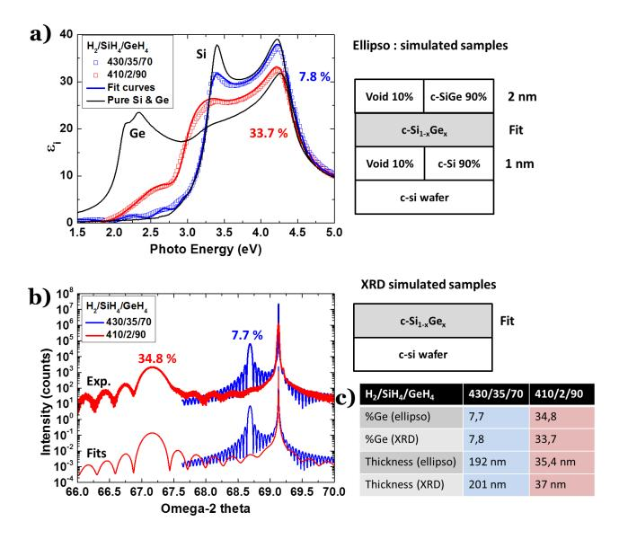
Figure 2.15 - a) and b):  $\omega$ -2 $\theta$  XRD scans and ellipsometric spectra of three Si<sub>1-x</sub>Ge<sub>x</sub> samples with various GeH4/(SiH4=GeH4) grown in Octopus reactor. c) Comparison of Ge content deduced from ellipsometry and XRD fits for several H<sub>2</sub>/SiH<sub>4</sub>/GeH<sub>4</sub> conditions.
