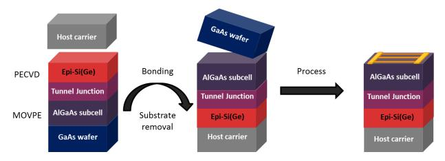
Figure 1.15 - Principle of the IMPETUS project. AlGaAs is grown on a GaAs substrate by MOVPE, followed by a tunnel junction and crystalline Si or SiGe grown by PECVD below 200 °C. The structure grown is then transferred to a low-cost carrier, the substrate removed, and the device is fabricated by standard clean room processes.
