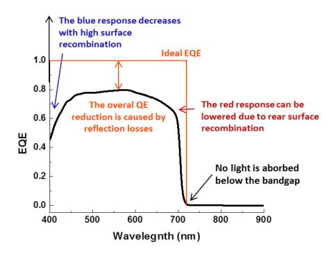
Figure 2.22 - Measured quantum efficiency of a AlGaAs solar cell, along with the main contributions responsible for possible EQE reductions.
