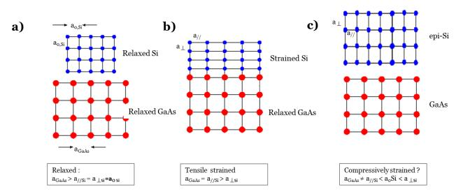
Figure 3.4 - Schematics of an heteroepitaxy in case of a larger substrate lattice constant than that of theepi-layer in the a) relaxed configuration, b) strained configuration (tensile strain) c) shematics ofour epi-Si/GaAs according to the lattice parameters deduced from XRD measurements
