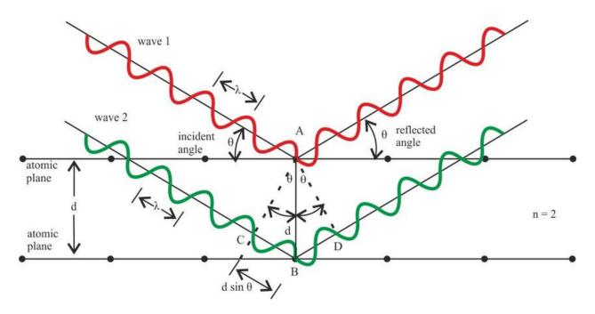
Figure 2.5 - Schematic representation of Bragg's law
