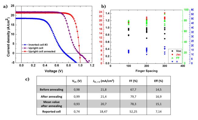
Figure 5.19 - a) JV curves of a bonded inverted solar cell (blue), and an uprigth solar cell before (purple) and after annealing (red) b) characteristics of the uptight solar cells after annealing as a function of the finger spacing, c) Details of the solar cell characteristics
