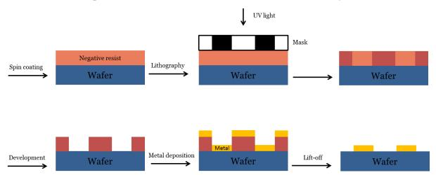
Figure 4.6 - Detailed process of a metal pattern by lift-off technique
