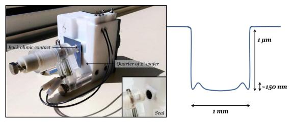
Figure 3.9 - a) Picture of the electrochemical cell used in ECV. Inset down right: picture of the seal that contacts the wafer surface b) Depth profile of a typical crater after etching.
