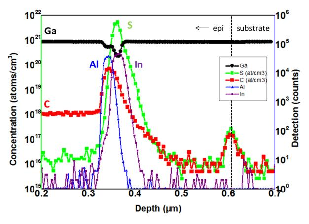
Figure 4.11 - SIMS analysis of AlGaAs/GaInP tunnel junction.
