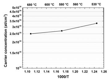
Figure 4.13 - Carrier concentration as a function of temperature
