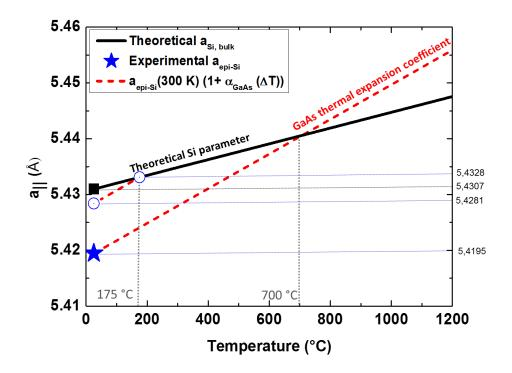
Figure 3.8 - Evolution of a// of a bulk Si as a function of temperature (black) and expected evolution of a// of epi-Si layer that follows the GaAs substrate expansion.
