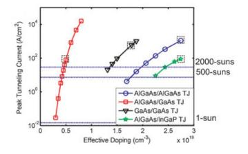
Figure 4.3- Peak tunnelling current as a function of the effective doping level for various TJ material combinations. (Simulation and experimental, from Wheeldon *et al.*<sup>158</sup>)
