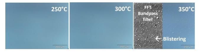
Figure 2.12 - Optical microscope images of the sample surface for different annealing temperatures
