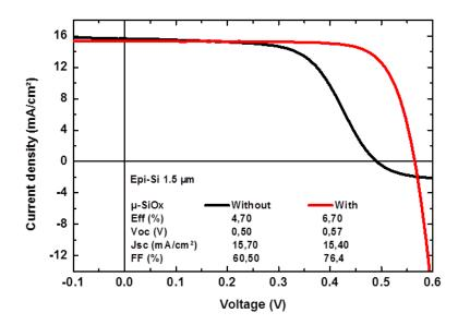
Figure 2.23 - J-V characteristics of as-deposited 1.5  $\mu$ m thick epi-Si without the addition of  $\mu$ -SiO<sub>x</sub> (black curve), and with (red curve)
