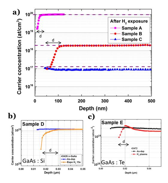
Figure 3.10 - a) Carrier concentration profiles measured by ECVof three p-GaAs:C samples with different initial doping levels, after hydrogen plasma exposure. Dashed lines show the nominal carrier concentrations of each sample. b)c) Carrier concentration profiles before and after plasma exposure for b) GaAs:Si, c) GaAs:Te
