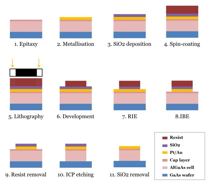
Figure 5.6 - Cross section schematics of the solar cell process flow detailing the 11 first steps required for the mesa etching
