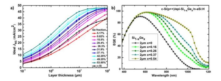
Figure 2.26 - Ideal J<sub>sc</sub> as a function of SiGe thickness for various Ge content. b) PC1D model of EQE variation with Ge content for a (p++)c-Si/epi-SiGe/n-a-Si:H solar cell. From Cariou thesis p155.
