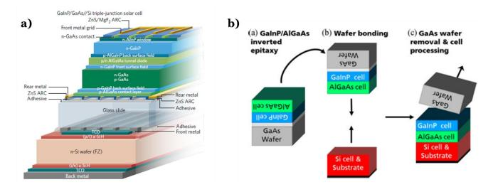
Figure 1.14 - a) Design of the four-terminal GaInP/GaAs//Si triple junction solar cell with 35.9 % efficiency (Essig et al. <sup>50</sup>) b) Design and process flow of GaInP/AlGaAs//Si triple junction wafer-bonded solar cell with 30.1% efficiency (Cariou et al. <sup>47</sup>)
