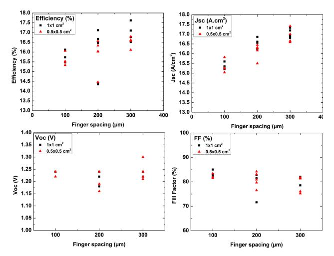
Figure 5.10 - Solar cell parameters as a function of the finger spacing. Black squares correspond to the large cells (1x1 cm<sup>2</sup>) and red triangles to the small ones (0.5x0.5 cm<sup>2</sup>)
