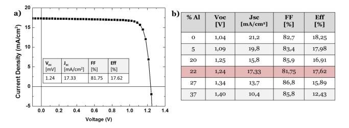
Figure 5.8 - a) J-V characteristics of the Al0.22Ga0.78As solar cell, b) detailed characteristics of the same cell as compared with results from Heckelmann *et al.*<sup>207</sup>
