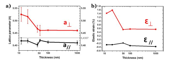
Figure 3.5 - a) evolution of the in-plane  $(a_{//})$  and out-of-plane  $(a_{\perp})$  lattice parameters as a function of the layer thickness, b) elastic deformation as a function of the layer thickness.
