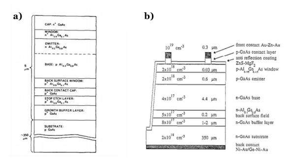
Figure 5.1 - a) Typical n on p structure (from Virshup et al.<sup>205</sup>) b) Typical n on p structure (from van Geelen et al<sup>216</sup>.)
