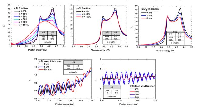
Figure 2.4 - Ellipsometric spetra (imaginary part of the dielectric function) simulated with DeltaPsi2 by varying a) c-Si/a-Si fraction, b) c-Si/p-Si fraction, c) native SiO2 thickness d) c-Si thickness e) roughness or defectivity of interface between substrate and epi-layer
