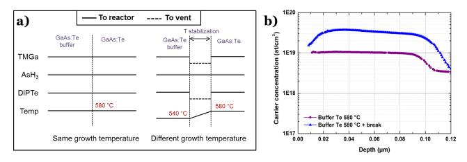
Figure 4.15 - a) Switching sequences of precursors in case of no temperature change (left) andwith a temperature change (rigth) b) Doping profile of the upper doped layer grown directly after the buffer layer (purple circles), and grown after an annealing (blue triangles)
