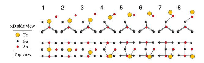
Figure 4.17 - Exchange process between Te surfactant and GaAs (From Consorte et al. <sup>187</sup>)
