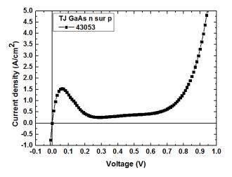
Figure 4.9 - J-V characteristics of n on p GaAs tunnel junction
