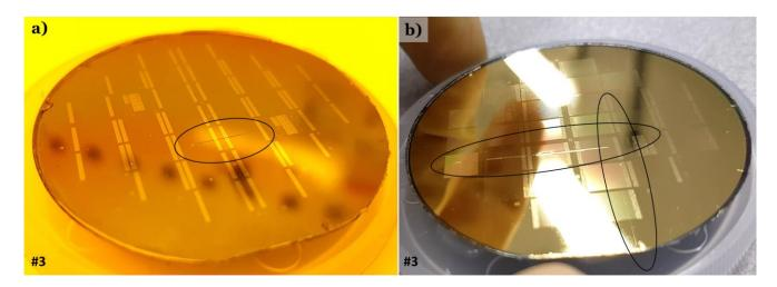
Figure 5.16 - Wafer #3 a) after resist deposition, b) after front metal deposition
