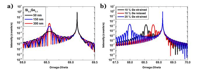
Figure 2.6 - Simulation with Leptos software of a)  $Si_{0.9}Ge_{0.1}$  layer with various thicknesses on a (100) Si substrate: the oscillation period and the peak intensity and FWHM are strongly dependent on the thickness b) Comparison of a strained  $Si_{0.8}Ge_{0.2}$  layer with a strained  $Si_{0.9}Ge_{0.1}$  and a relaxed one : the peak is shifted to the right when relaxed.
