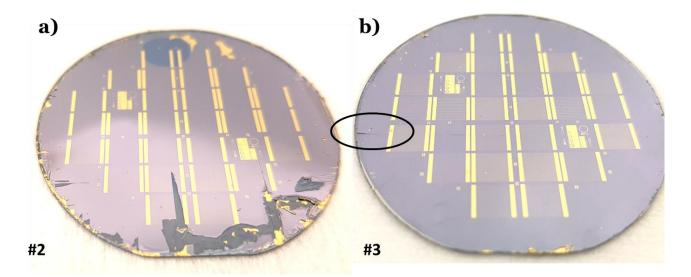
Figure 5.17 - a) Wafer #2 after metal lift-off: the active layer has been removed where the previous bubles were present. b) Wafer #3 after metal lift-off: the previous cracks have been enlarged.
