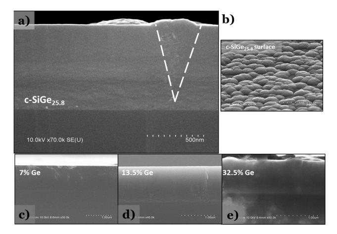
Figure 2.29 -SEM images of a)b) the cross-section and surface of SiGe<sub>25.8</sub> c)d)e) the cross-section for x = 7%, 13.5% and 32.5%.
