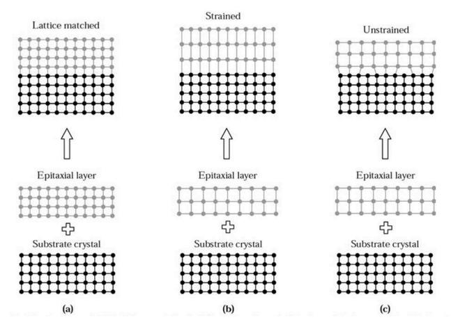
Figure 1.7 - Schematic illustration of (a) lattice-matched, (b) strained and (c) relaxed hetero-epitaxial structures. (b) and (c) are shown in case of  $a_{substrate} < a_{layer}$  (<sup>22</sup>)
