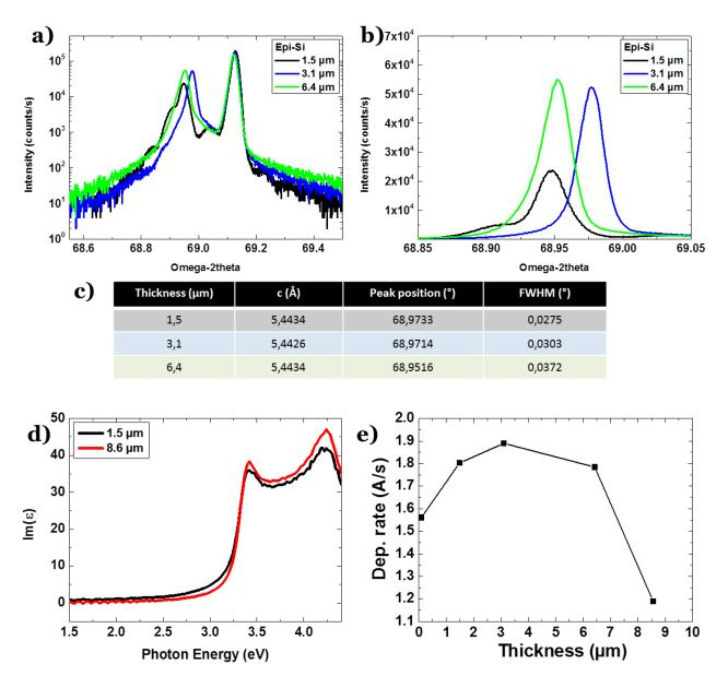
Figure 2.13 - a)  $\omega$ -2 $\theta$  XRD scans of samples with various thicknesses: 1.5  $\mu$ m, 3.1  $\mu$ m and 6.4  $\mu$ m, b) zoom on the epi layer peak in linear scale, c) lattice parameter, peak position and FWHM deduced from XRD data d) ellipsometric spectra of 1.5  $\mu$ m and 8.6  $\mu$ m samples, e) evolution of deposition rate as a function of the thickness of the film.
