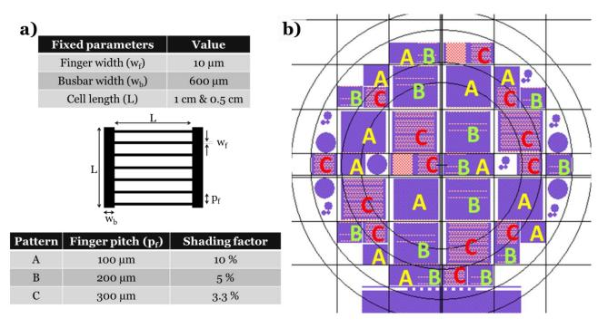
Figure 5.3- a) 3 different patterns with various busbars and finger dimensions of the tested cells. b) L-edit screenshot of the grid disposition on a 3 inch. wafer. The 3 configurations are tested on 1x1 cm2 and 0.5x0.5cm<sup>2</sup> cells.
