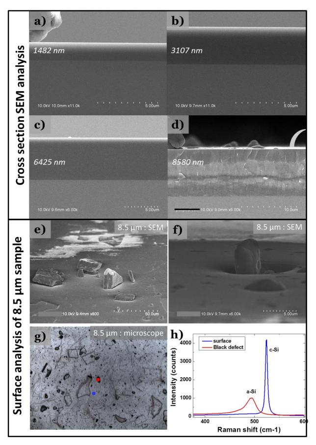
Figure 2.14 - a)b)c)d) cross-section SEM analysis of samples with thicknesses of 1.5  $\mu$ m, 3.1  $\mu$ m, 6.4  $\mu$ m, 8.5  $\mu$ m, along with the thickness measured thanks to this image. e)f) SEM images of the surface of the 8.5  $\mu$ m sample, g)h) Raman spectroscopy spectra of the material on different surface spots : a defect, and the smooth surface of the film
