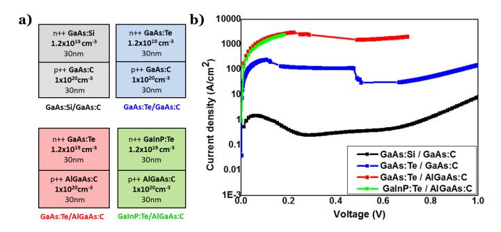
Figure 4.20 - a) Tunnel junction structures b) and J-V characteristics
