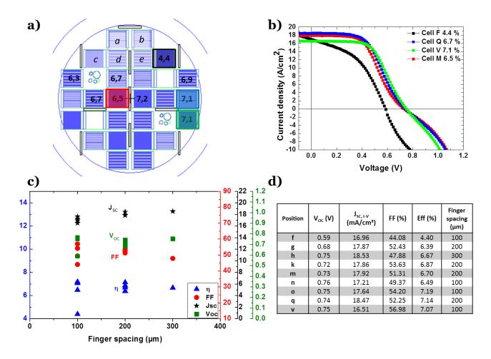
Figure 5.18 - a) Spatial repartition of the different cells that are not shunted with their efficiency. b) J-V curve of 4 of these functioning cells c)  $V_{oc}$ ,  $J_{sc}$ , FF and efficiency as a function of the finger spacing, d) Results on each functioning cell
