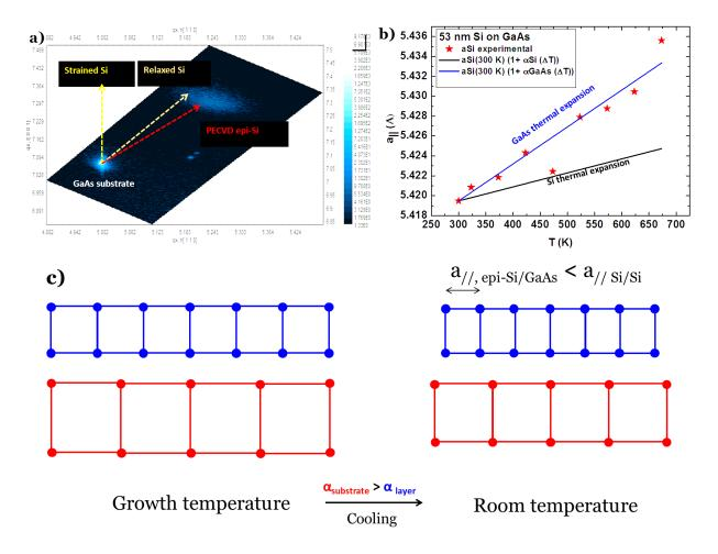
Figure 3.7 - a) {224} reciprocal space mapping of a epi-Si/GaAs sample, b) evolution of the lattice-parameter of an epi-Si while performing an annealing up to 400 °C, c) Schematics of the lattice of a relaxed Si layer on top of a GaAs during growth, and after cooling down to room temperature, considering that Si follows GaAs thermal expansion coefficient.
