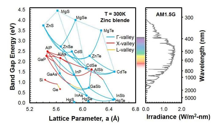
Figure 1.5 - Bandgap versus lattice constant at room temperature for various materials including Si, Ge, GaAs.
