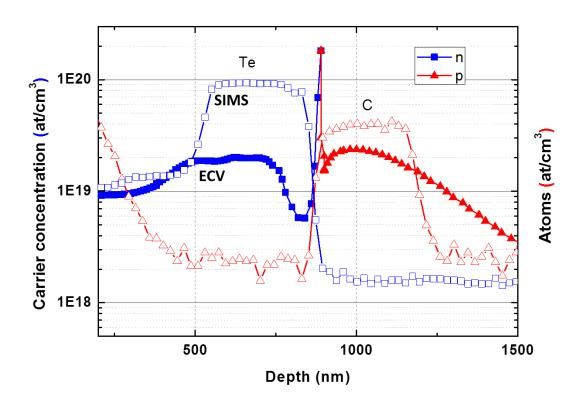
Figure 4.19 - ECV measurements (full symbols) as compared with SIMS analyses (open symbols) of a n on p GaAs/GaAs tunnel junction doped with Te and C.
