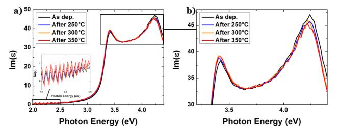
Figure 2.10 - a) Ellipsometric spectra of the samples as-deposited, and annealed at 250°C, 300 °C and 350 °C, along with a zoom on the low energy oscillations b) zoom on the characteristic peaks at  $E_1$  and  $E_2$
