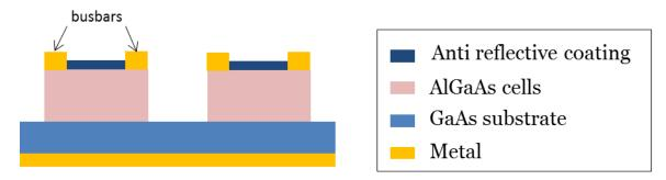
Figure 5.4 - Cross-section schematic of the targeted device after process
