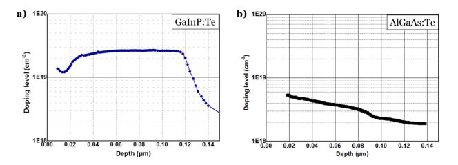
Figure 4.18 - ECV measurements : best doping profiles obtained for a. GaInP doped with Te, b. AlGaAs doped with Te.
