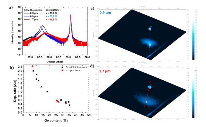
Figure 2.18 -  $\omega$ -2 $\theta$  XRD scans of SiGe25.8 with increasing thicknesses: 0.5  $\mu$ m, 0.9  $\mu$ m and 1.7  $\mu$ m, b) Deposition rate as a function of Ge content for the thin calibration layers (<200 nm) and the thick layers. c)d), RSM of 0.9 and 1.7  $\mu$ m samples: the latest is partly relaxed.
