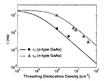
Figure 1.9 - minority carrier lifetime in GaAs as a function of threading dislocation dislocation density (Andre et al. <sup>26</sup>)
