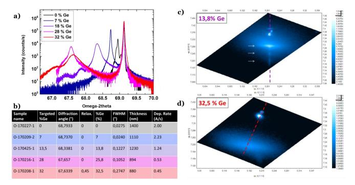
Figure 2.17 -  $\omega$ -20 XRD scans of Si<sub>1-x</sub>Ge<sub>x</sub> for various x values, aiming at a thickness of 1  $\mu$ m b) fitted parameters deduced from XRD (diffraction angle, Ge content, FWHM) and SEM (thickness) d), RSM of the samples with x=13.8% and x=32.5% samples: the latest is partly relaxed.
