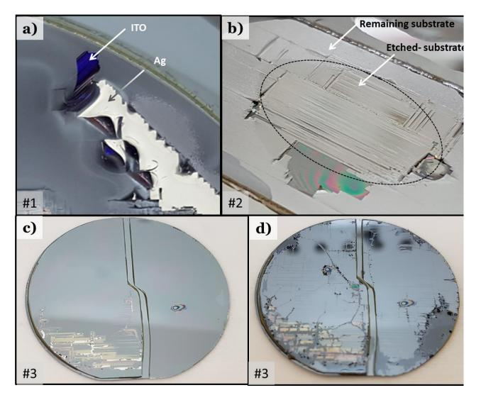
Figure 5.20 - a) Picture of layer detachment between Ag and ITO, b) picture of a tandem solar cell (#2) after 750  $\mu$ m-thick GaAs substrate removal, c) picture of a tandem solar cell (#3) after 350  $\mu$ m - thick substrate removal d) #3 after GaInP etch-stop etching
