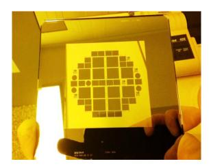
Figure 5.5 - Picture of the lithographic mask used to define the mesa etching pattern
