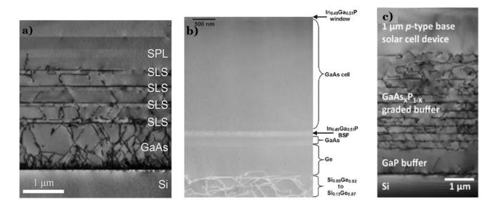
Figure 1.10 - TEM analysis of a) direct growth of GaAs on Si (Luxmoore et al. <sup>30</sup>), b) SiGe graded layers (Andre et al. <sup>37</sup>) (c) GaP buffer layer (Lang et al. <sup>39</sup>)
