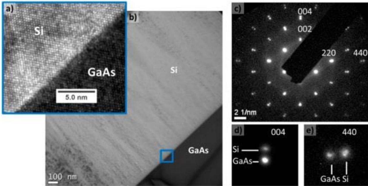
Figure 3.2 - a) Cross-section HRTEM image of epi-Si/GaAs interface. b) Low magnification cross section picture of a 650 nm thick epi-Si layer on GaAs. c) Diffraction pattern of PECVD epi-Si/GaAs interface: the double points visible for each reflection (see zooms (d,e)) are the signature of both Si and GaAs lattices. From Cariou *et al.*<sup>6</sup>
