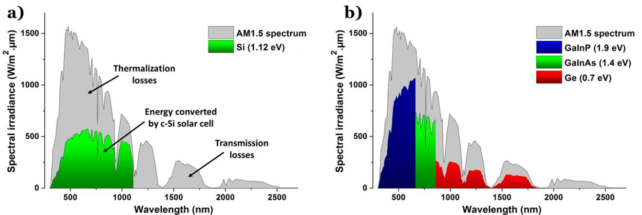
Figure 1.3- AM1.5G spectrum and the fraction theoretically converted by a) a Si solar cell, b) a triple junction GaInP/GaInAs/Ge (from ref<sup>9</sup>)
