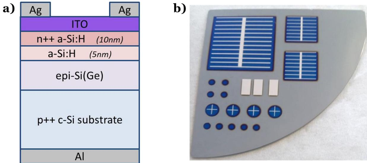
Figure 2.20 - a) Structure of the heterojunction solar cell grown and processed, b) top-view picture of the device after ITO deposition and metallization : one 2x2  $\text{cm}^2$  and two 1x1  $\text{cm}^2$  cells can be distinguished.
