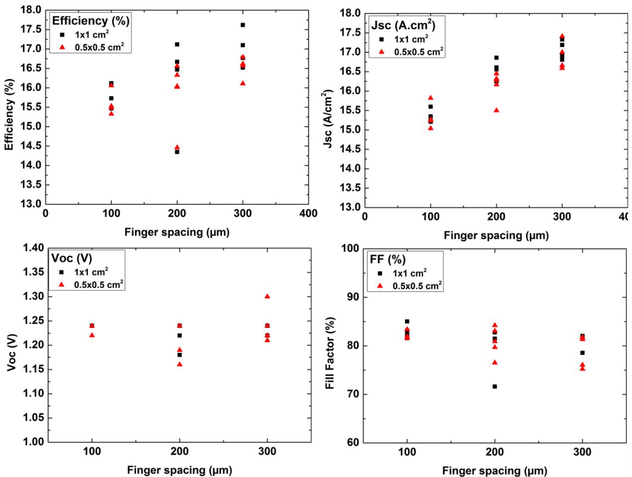
Figure 5.10 - Solar cell parameters as a function of the finger spacing. Black squares correspond to the large cells ( $1 \times 1\text{ cm}^2$ ) and red triangles to the small ones ( $0.5 \times 0.5\text{ cm}^2$ )
