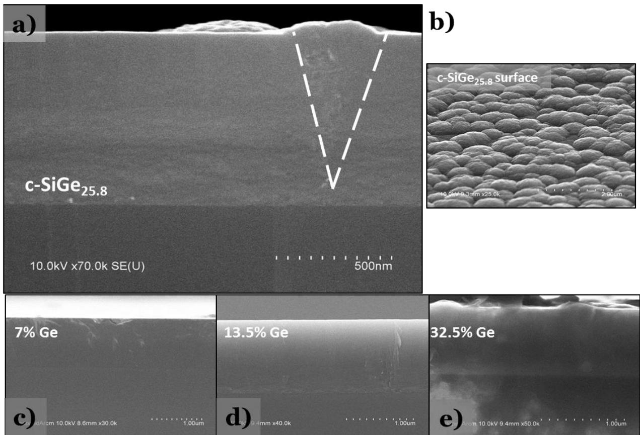
**Figure 2.29 -SEM images of a)b) the cross-section and surface of SiGe<sub>25.8</sub> c)d)e) the cross-section for x = 7%, 13.5% and 32.5%.**
