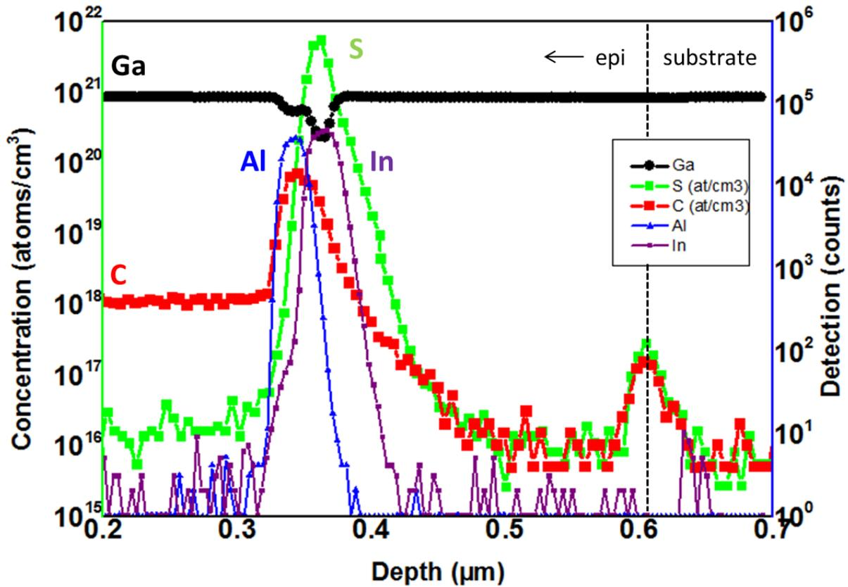
Figure 4.11 - SIMS analysis of AlGaAs/GaInP tunnel junction.
