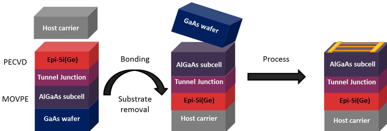
Figure 1.15 - Principle of the IMPETUS project. AlGaAs is grown on a GaAs substrate by MOVPE, followed by a tunnel junction and crystalline Si or SiGe grown by PECVD below 200 °C. The structure grown is then transferred to a low-cost carrier, the substrate removed, and the device is fabricated by standard clean room processes.
