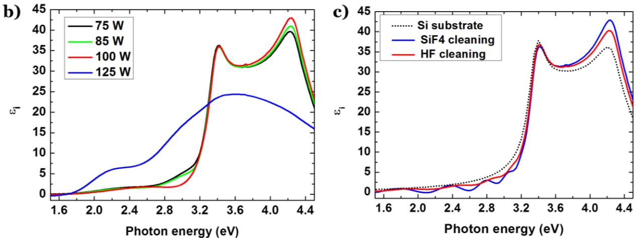
Figure 2.9 - a) Optimized cleaning and deposition conditions in Octopus reactor, b) ellipsometric spectra of 5 minutes growth Si after cleaning at various values of the RF power c) comparison of the best SiF<sub>4</sub> cleaning with HF cleaning, along with the substrate reference
