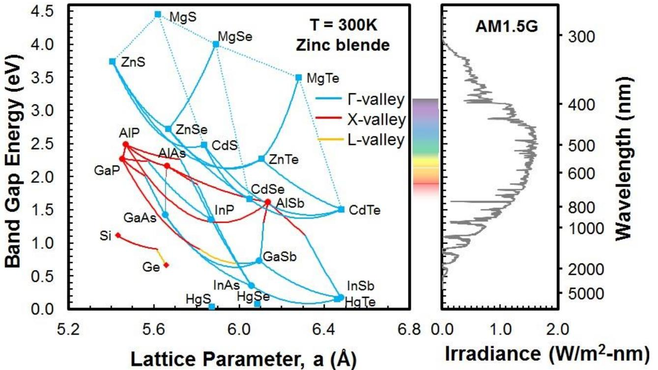
Figure 1.5 - Bandgap versus lattice constant at room temperature for various materials including Si, Ge, GaAs.
