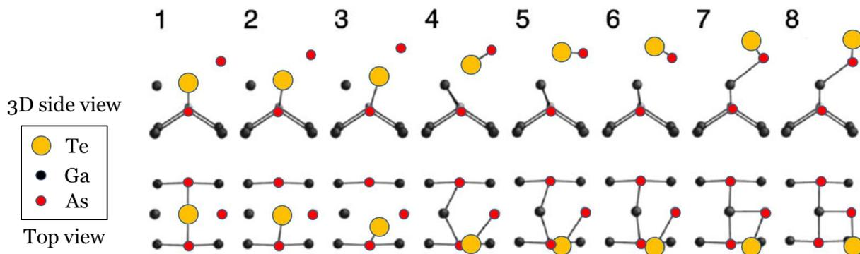
Figure 4.17 - Exchange process between Te surfactant and GaAs (From Consorte *et al.*<sup>187</sup>)
