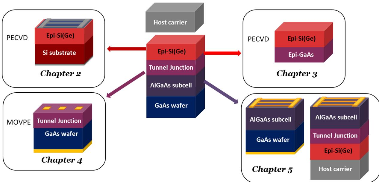
Figure 1.18 - Different building blocks of the tandem solar cell
