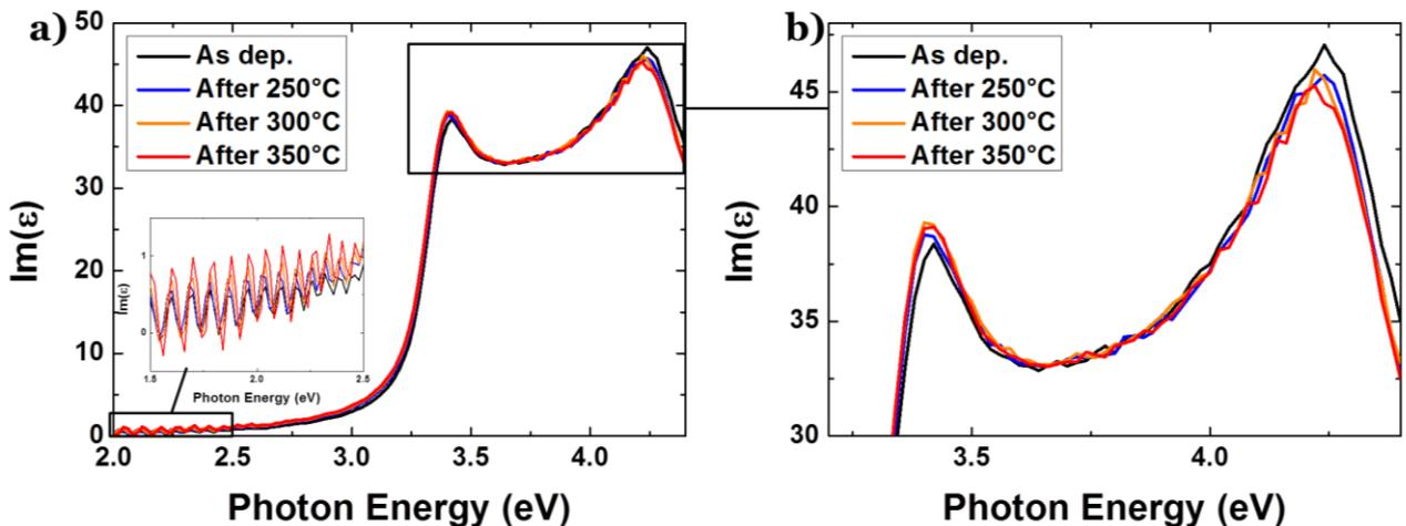
Figure 2.10 - a) Ellipsometric spectra of the samples as-deposited, and annealed at 250°C, 300 °C and 350 °C, along with a zoom on the low energy oscillations b) zoom on the characteristic peaks at  $E_1$  and  $E_2$
