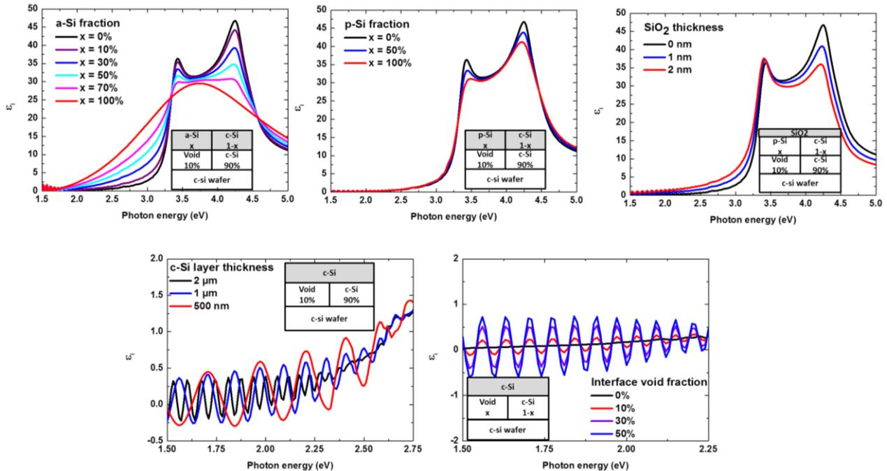
Figure 2.4 - Ellipsometric spectra (imaginary part of the dielectric function) simulated with DeltaPsi2 by varying a) c-Si/a-Si fraction, b) c-Si/p-Si fraction, c) native SiO<sub>2</sub> thickness d) c-Si thickness e) roughness or defectivity of interface between substrate and epi-layer
