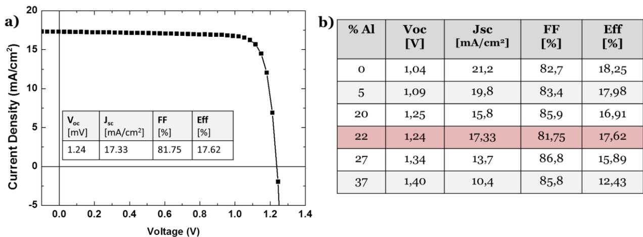
Figure 5.8 - a) J-V characteristics of the  $\text{Al}_{0.22}\text{Ga}_{0.78}\text{As}$  solar cell, b) detailed characteristics of the same cell as compared with results from Heckelmann *et al.*<sup>207</sup>
