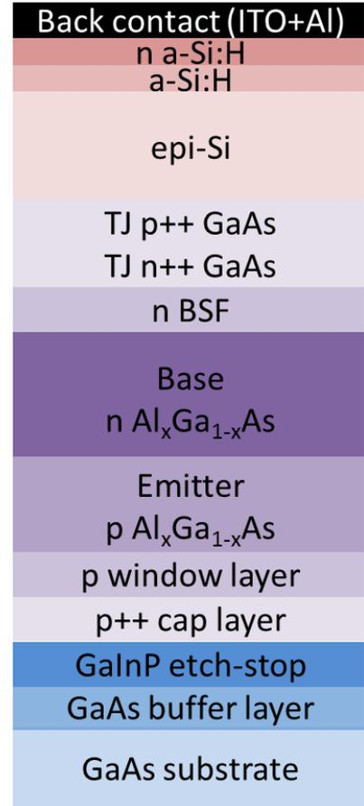
Figure 5.11 - Structure of the tandem device before bonding
