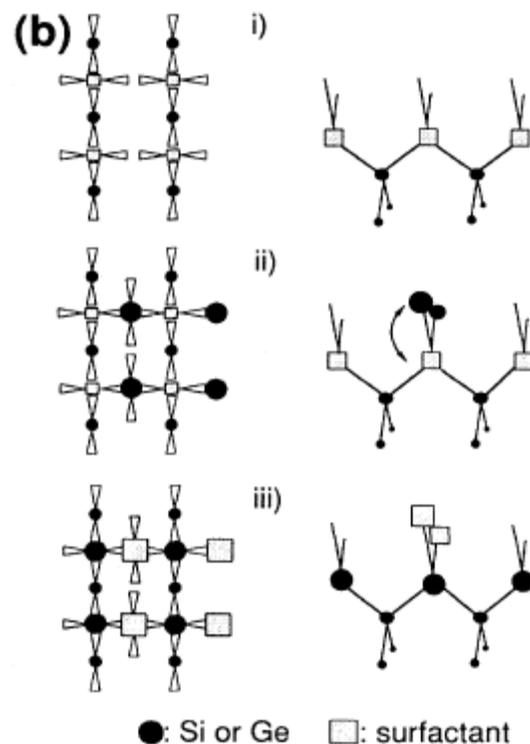
Figure 4.16 - Schematic representation of atomic mechanisms with reactive surfactant (from Grandjean *et al.*<sup>186</sup>)
