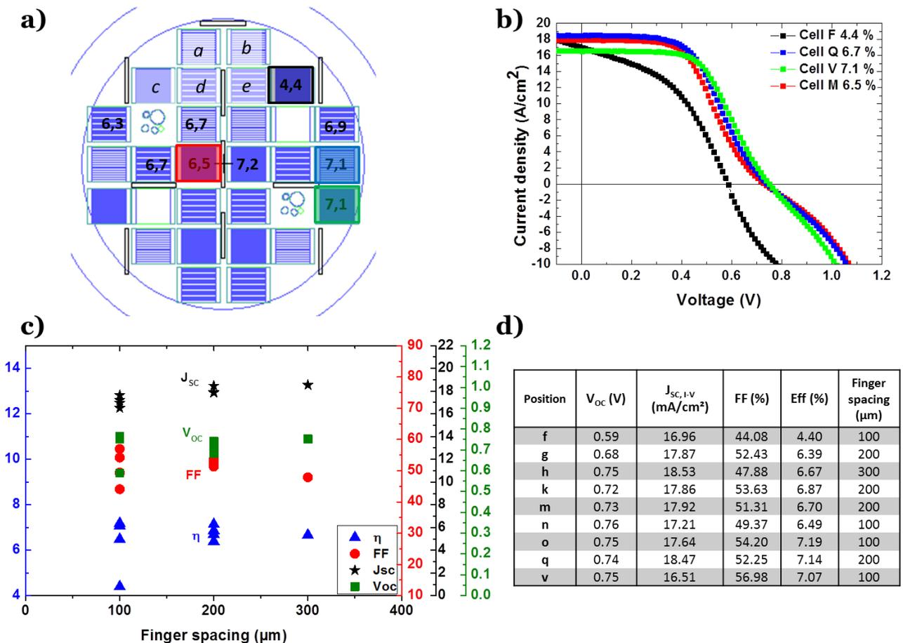
Figure 5.18 - a) Spatial repartition of the different cells that are not shunted with their efficiency. b) *J-V* curve of 4 of these functioning cells c) *V*<sub>oc</sub>, *J*<sub>sc</sub>, FF and efficiency as a function of the finger spacing, d) Results on each functioning cell
