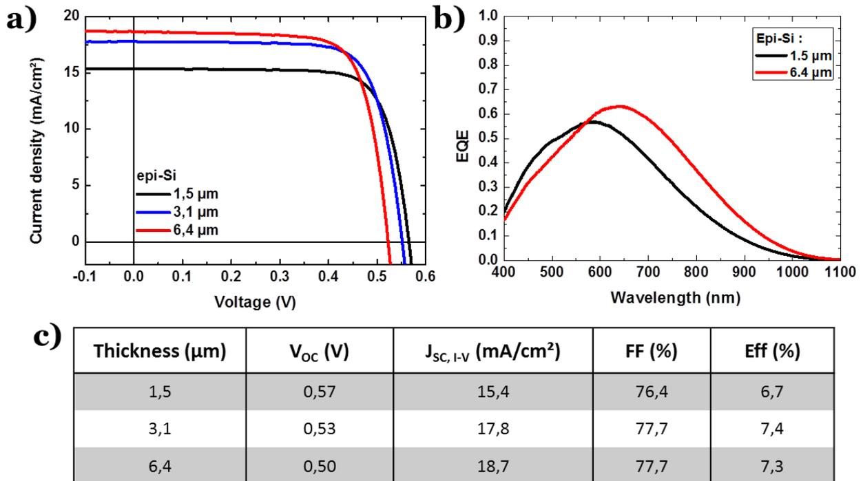
Figure 2.25 - J-V characteristics at low-temperature and b) external quantum efficiency of all the solar cells with various epitaxial thicknesses, c) solar cells characteristics calculated from J-V measurements
