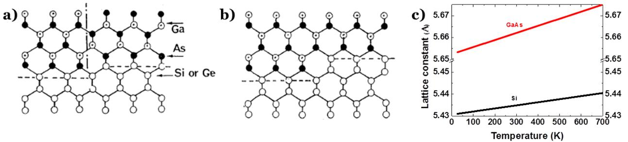
Figure 1.8 - (a) Mechanism of APB formation during the growth of zinc blende structure on (100) non polar surface presenting single-atomic high step, (b) Growth of a single domain zinc blende structure on a (100) non polar surface presenting double-atomic high step (from Freundlich<sup>23</sup>) (c) lattice constant of GaAs and Si as a function of temperature
