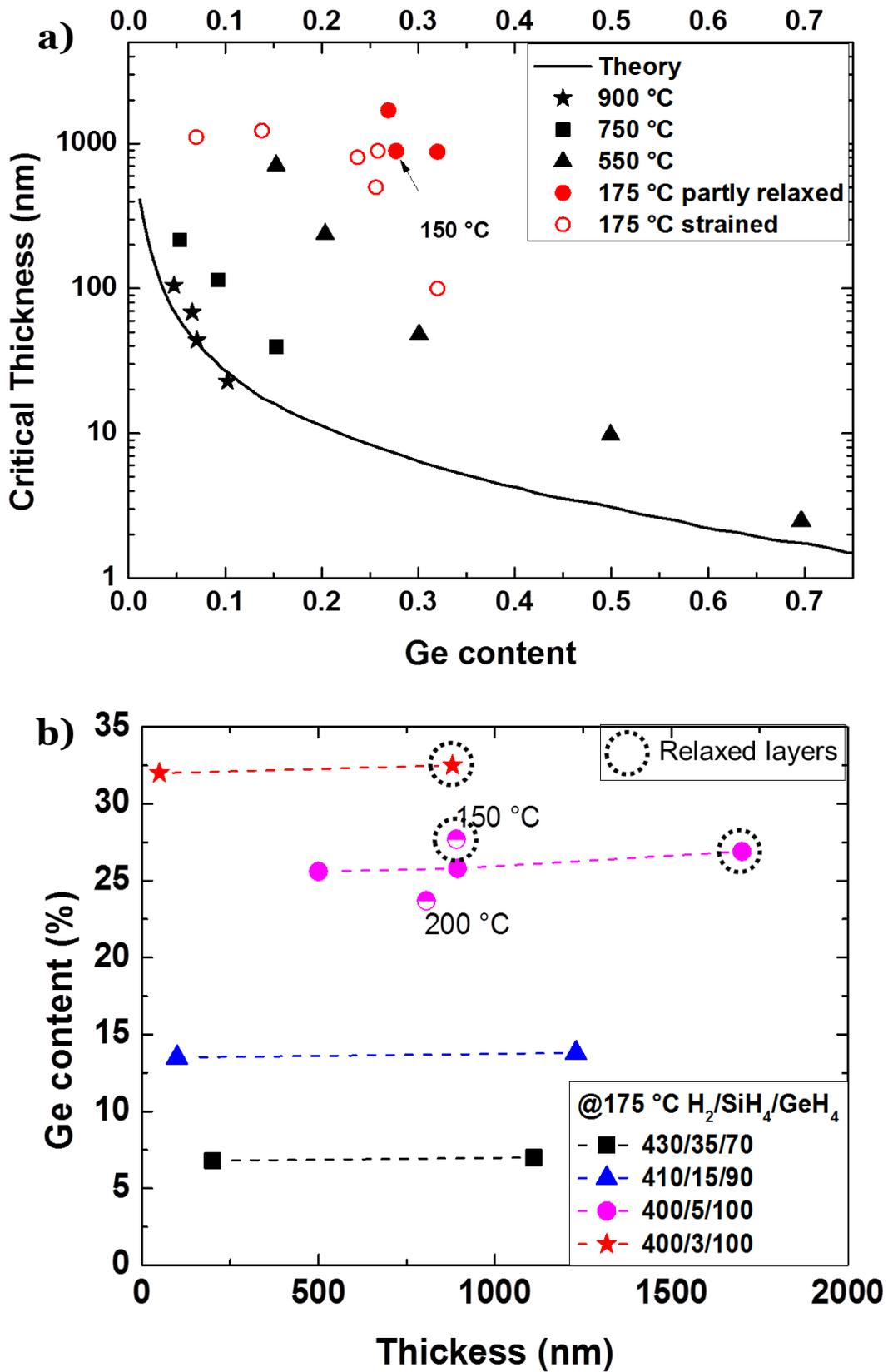
Figure 2.19 - a) Critical thickness of SiGe reported from Hull *et al.*<sup>107</sup> as a function of the growth temperature, compared to our samples. Low-temperature PECVD has a higher critical thickness than other techniques b) Ge content as a function of thickness for various growth conditions.
