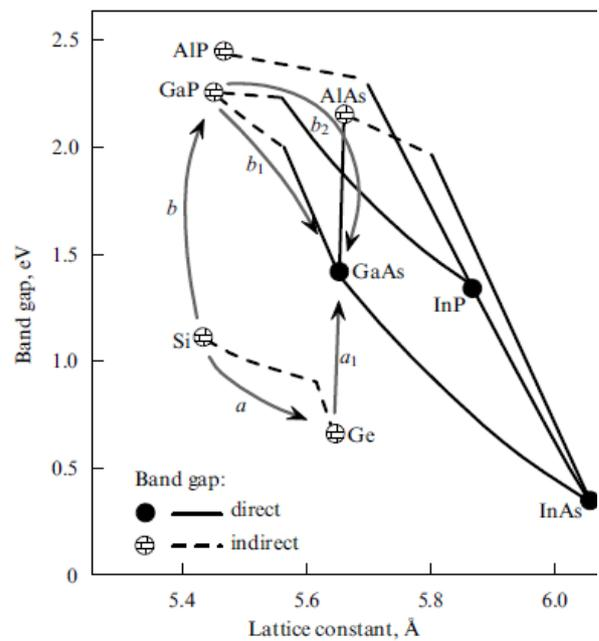
Figure 1.11 - Bandgap versus lattice constant for Si, Ge, and III-V compounds. Arrows indicate the possible pathways for integrating III-V on Si.
