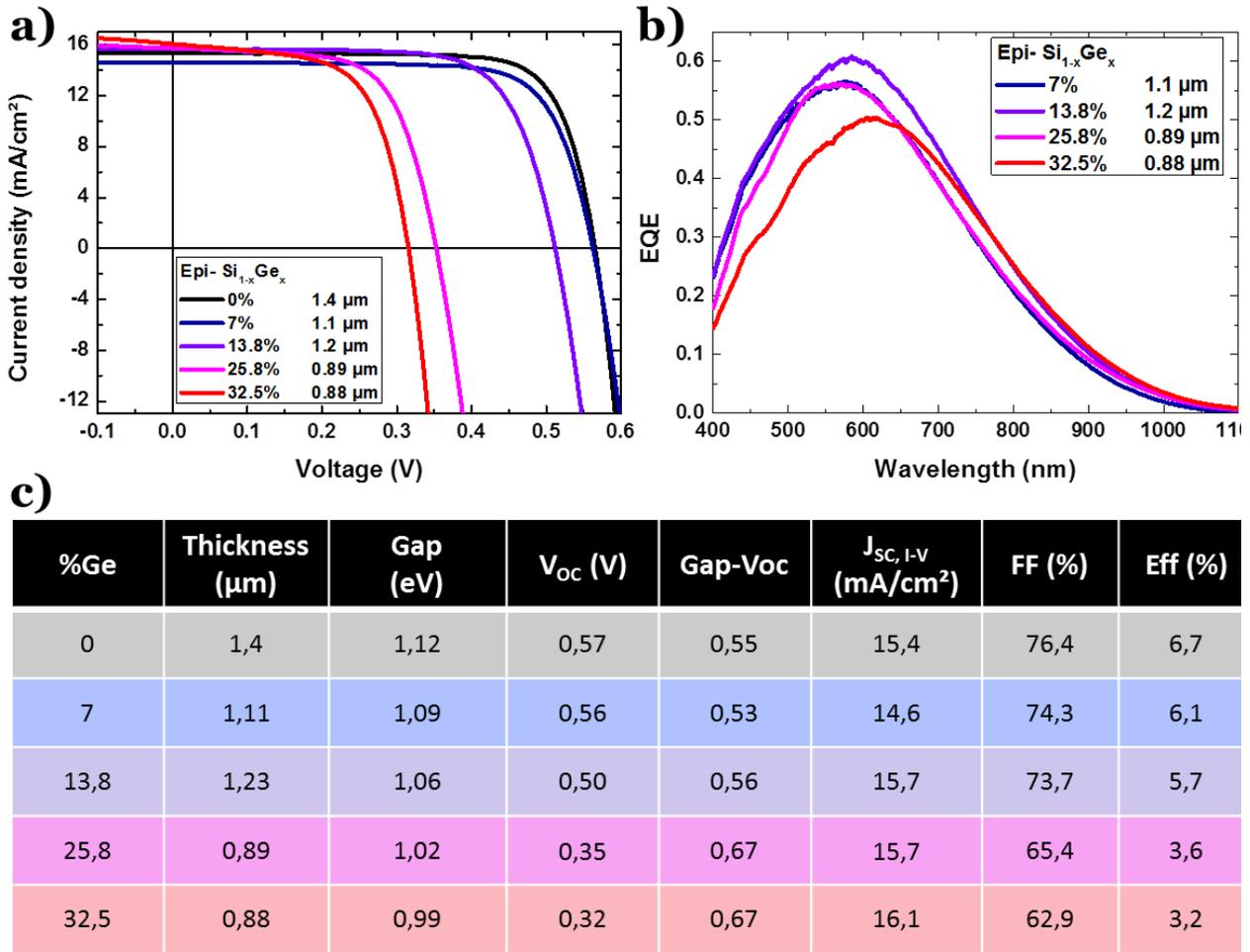
**Figure 2.28 - a) J-V characteristics at low-temperature and b) external quantum efficiency of all the solar cells processed after various annealing temperatures, c) summary of the material and cell parameters obtained**
