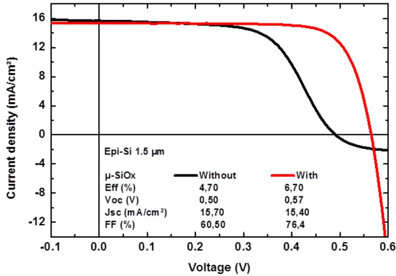
Figure 2.23 - J-V characteristics of as-deposited 1.5 μm thick epi-Si without the addition of μ-SiO<sub>x</sub> (black curve), and with (red curve)
