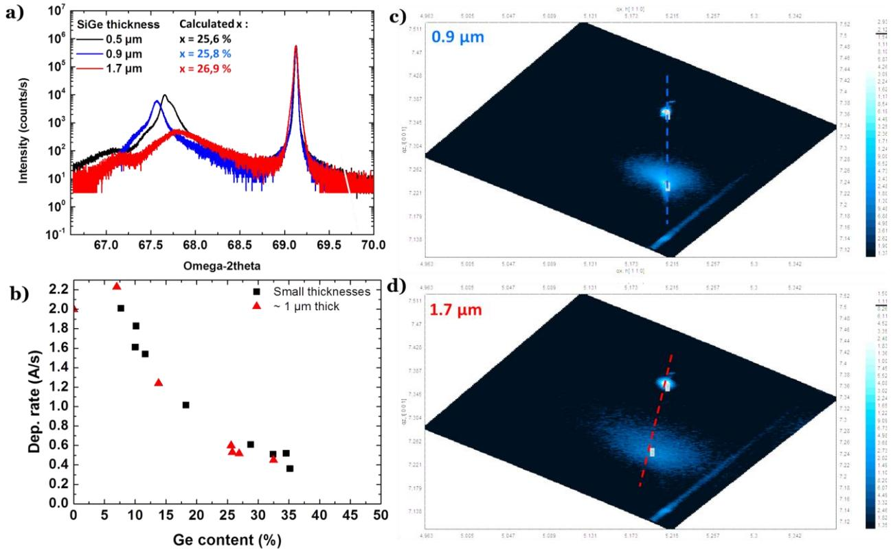
**Figure 2.18** -  $\omega$ - $2\theta$  XRD scans of SiGe<sub>25.8</sub> with increasing thicknesses: 0.5  $\mu\text{m}$ , 0.9  $\mu\text{m}$  and 1.7  $\mu\text{m}$ , **b)** Deposition rate as a function of Ge content for the thin calibration layers (<200 nm) and the thick layers. **c)d)** RSM of 0.9 and 1.7  $\mu\text{m}$  samples: the latest is partly relaxed.
