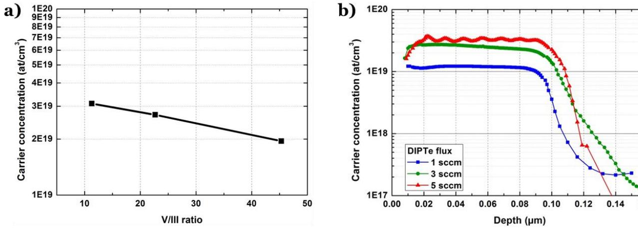
Figure 4.12 - a) Carrier concentration as a function of III/V ratio with fixed growth conditions of  $T = 580\text{ }^{\circ}\text{C}$ , on an undoped GaAs buffer. b) ECV measurements for three different DIPTe flow rates
