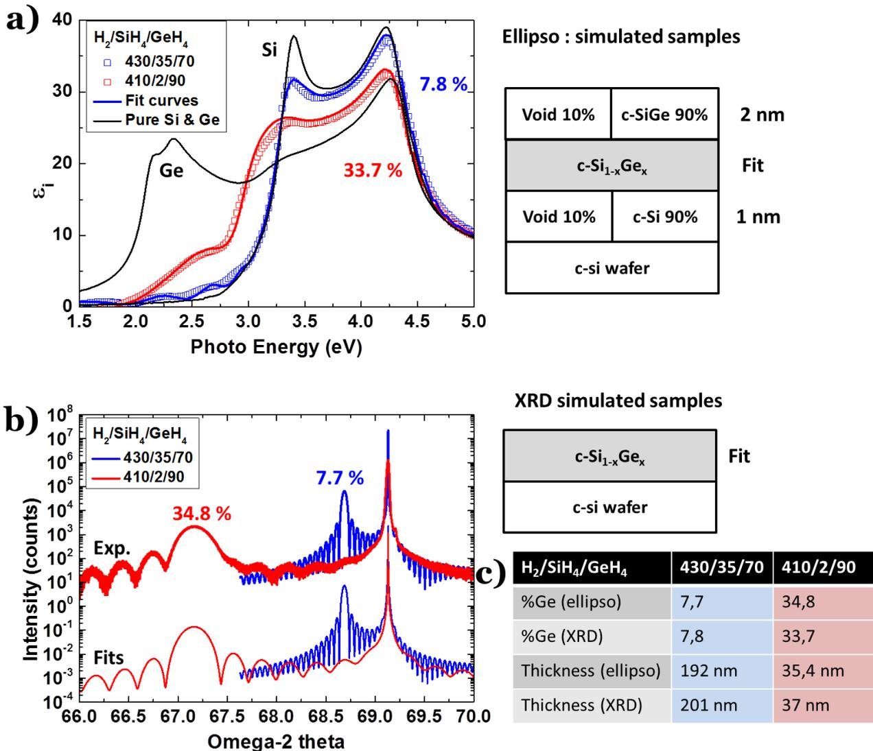
Figure 2.15 - a) and b):  $\omega$ -2 $\theta$  XRD scans and ellipsometric spectra of three  $Si_{1-x}Ge_x$  samples with various  $GeH_4/(SiH_4+GeH_4)$  grown in Octopus reactor. c) Comparison of Ge content deduced from ellipsometry and XRD fits for several  $H_2/SiH_4/GeH_4$  conditions.
