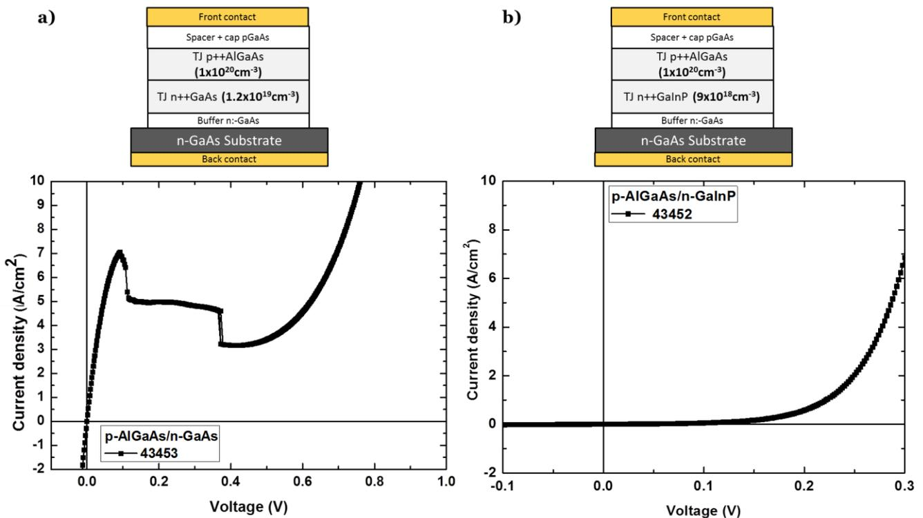
Figure 4.10 - Structure and J-V characteristics of a) AlGaAs/GaAs tunnel junction and b) AlGaAs/GaInP
