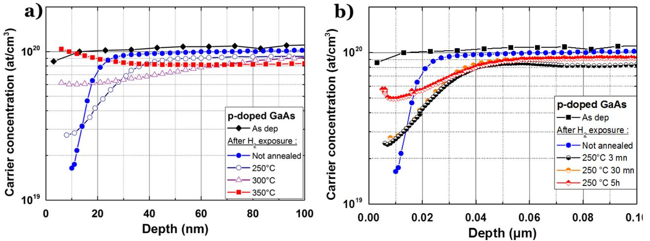
Figure 3.11 -ECV profiling of GaAs :C before H<sub>2</sub> exposure, after H<sub>2</sub> exposure and after a) 3-minutes annealing at various temperatures, b) annealing at 250 °C for various durations
