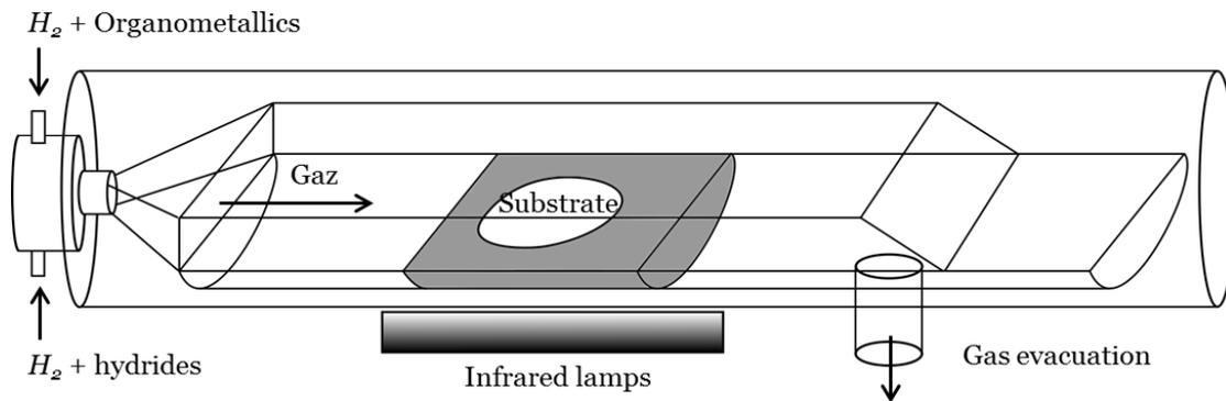
Figure 4.4 - Principle of the AIX200 reactor
