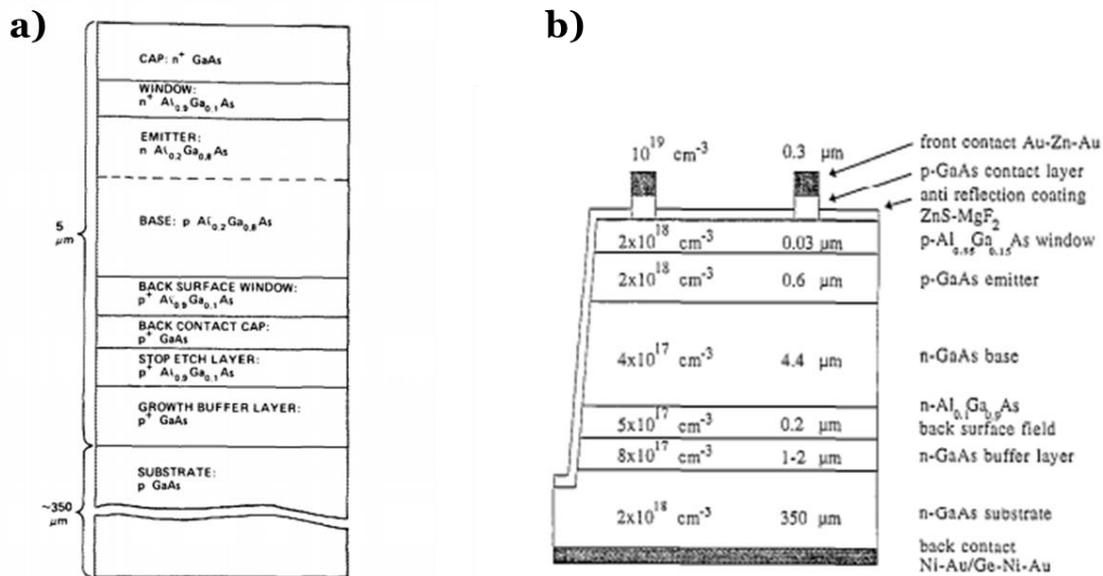
Figure 5.1 - a) Typical n on p structure (from Virshup et al.<sup>205</sup>) b) Typical n on p structure (from van Geelen et al.<sup>216</sup>.)
