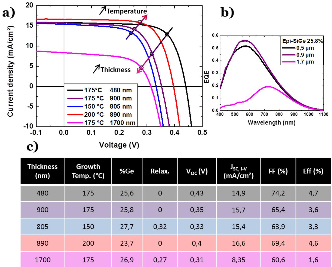
Figure 2.30 - a)  $J$ - $V$  characteristics at low-temperature and b) external quantum efficiency of all the solar cells processed after various annealing temperatures, c) summary of the parameters obtained
