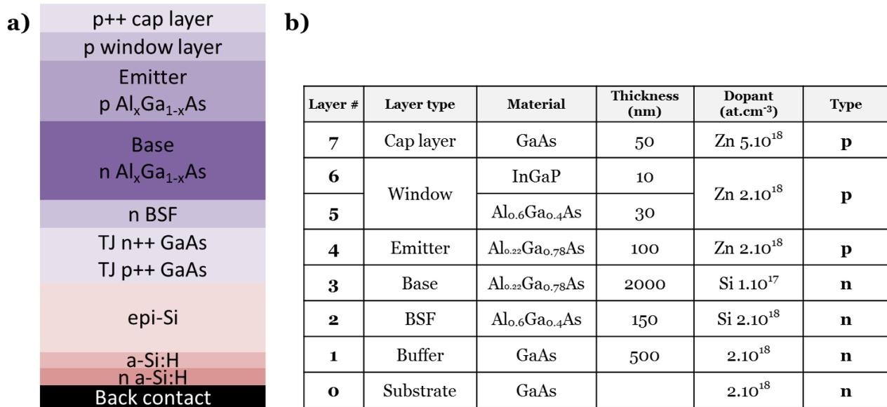
**Figure 5.2 - a) Complete structure of the tandem solar cell b) Al<sub>0.22</sub>Ga<sub>0.78</sub>As solar cell structure grown by MOVPE on GaAs substrate**
