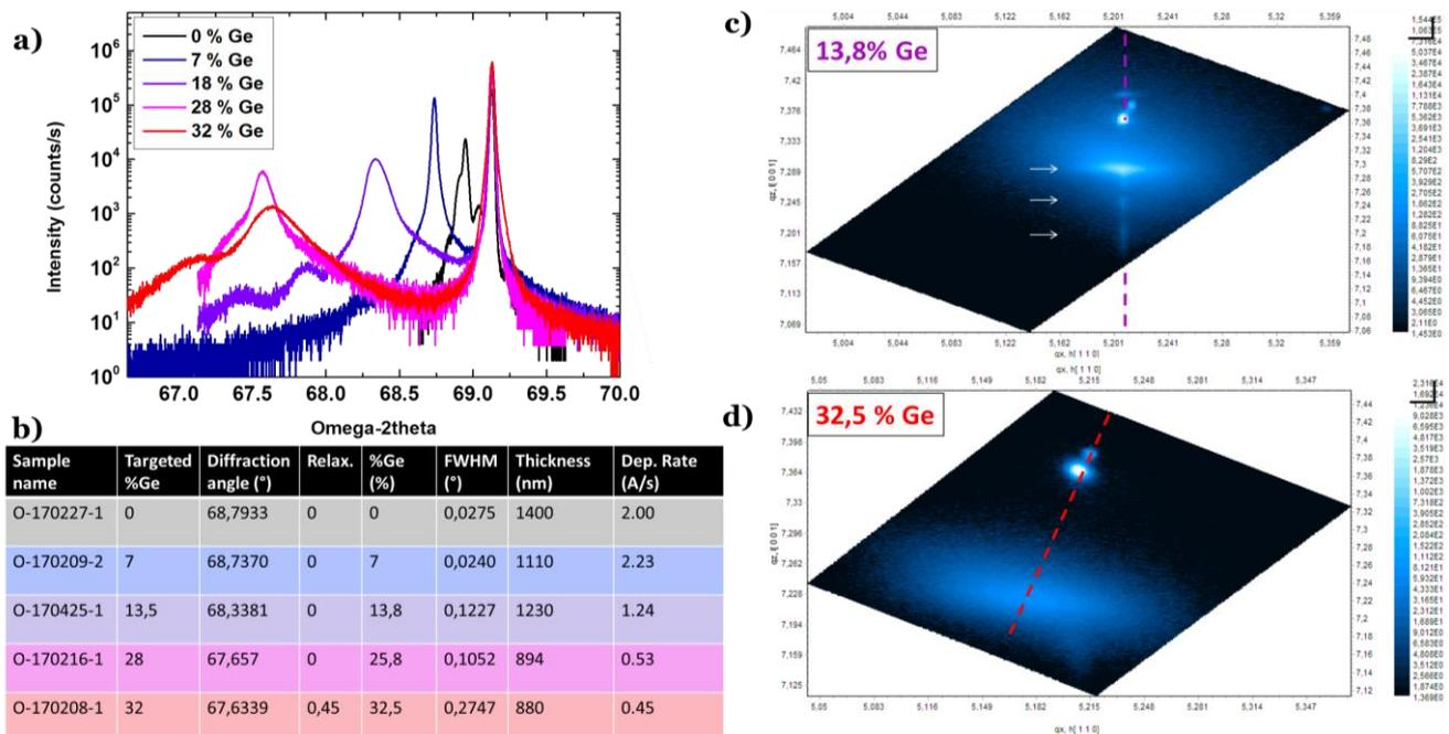
Figure 2.17 -  $\omega$ - $2\theta$  XRD scans of  $\text{Si}_{1-x}\text{Ge}_x$  for various  $x$  values, aiming at a thickness of  $1\ \mu\text{m}$  b) fitted parameters deduced from XRD (diffraction angle, Ge content, FWHM) and SEM (thickness) d), RSM of the samples with  $x=13.8\%$  and  $x=32.5\%$  samples: the latest is partly relaxed.
