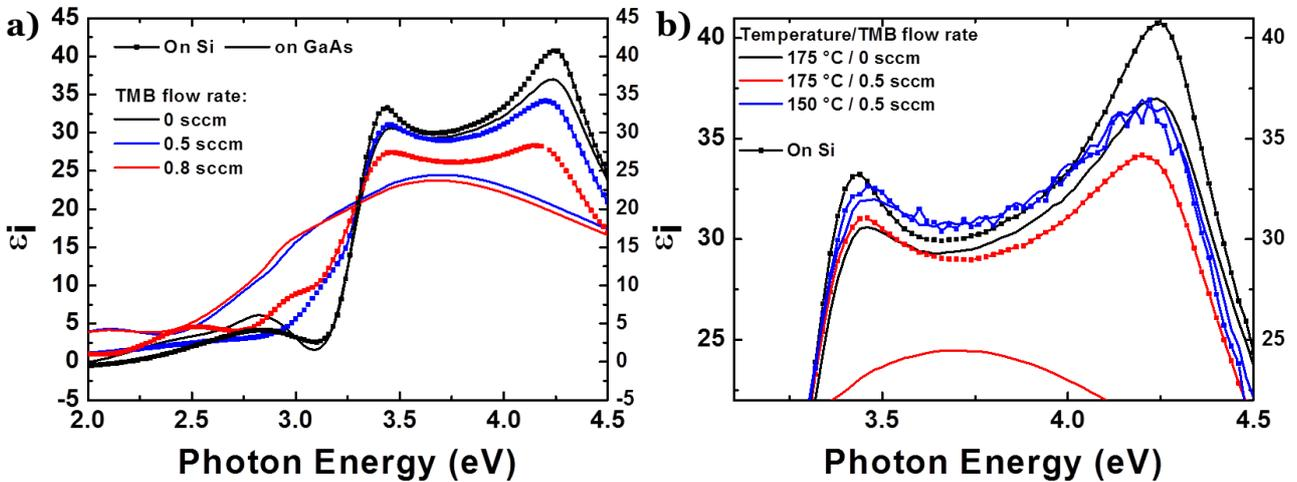
Figure 4.24 - a) Ellipsometric spectra of Si grown with TMB on Si substrate (squared) and on epi-GaAs (lines) with various TMB flow rates, b) Ellipsometric spectra on Si and epi-GaAs at various TMB flow rate and temperatures
