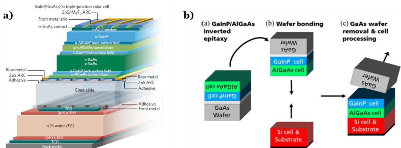
Figure 1.14 - a) Design of the four-terminal GaInP/GaAs//Si triple junction solar cell with 35.9 % efficiency (Essig et al. <sup>50</sup>) b) Design and process flow of GaInP/AlGaAs//Si triple junction wafer-bonded solar cell with 30.1% efficiency (Cariou et al. <sup>47</sup>)
