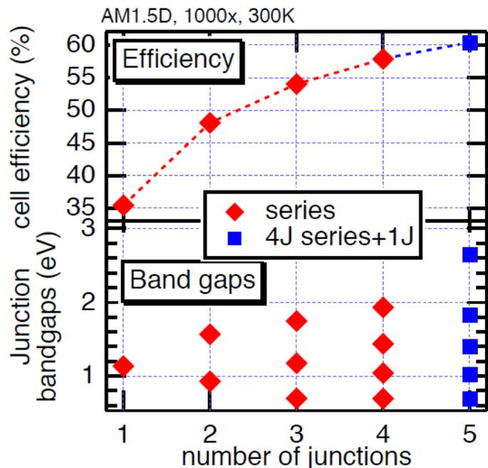
Figure 1.4 - Theoretical maximum efficiency of a multijunction as a function of the number of junctions, along with the corresponding bandgaps (NREL)<sup>11</sup>
