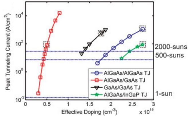
Figure 4.3- Peak tunnelling current as a function of the effective doping level for various TJ material combinations. (Simulation and experimental, from Wheeldon *et al.*<sup>158</sup>)
