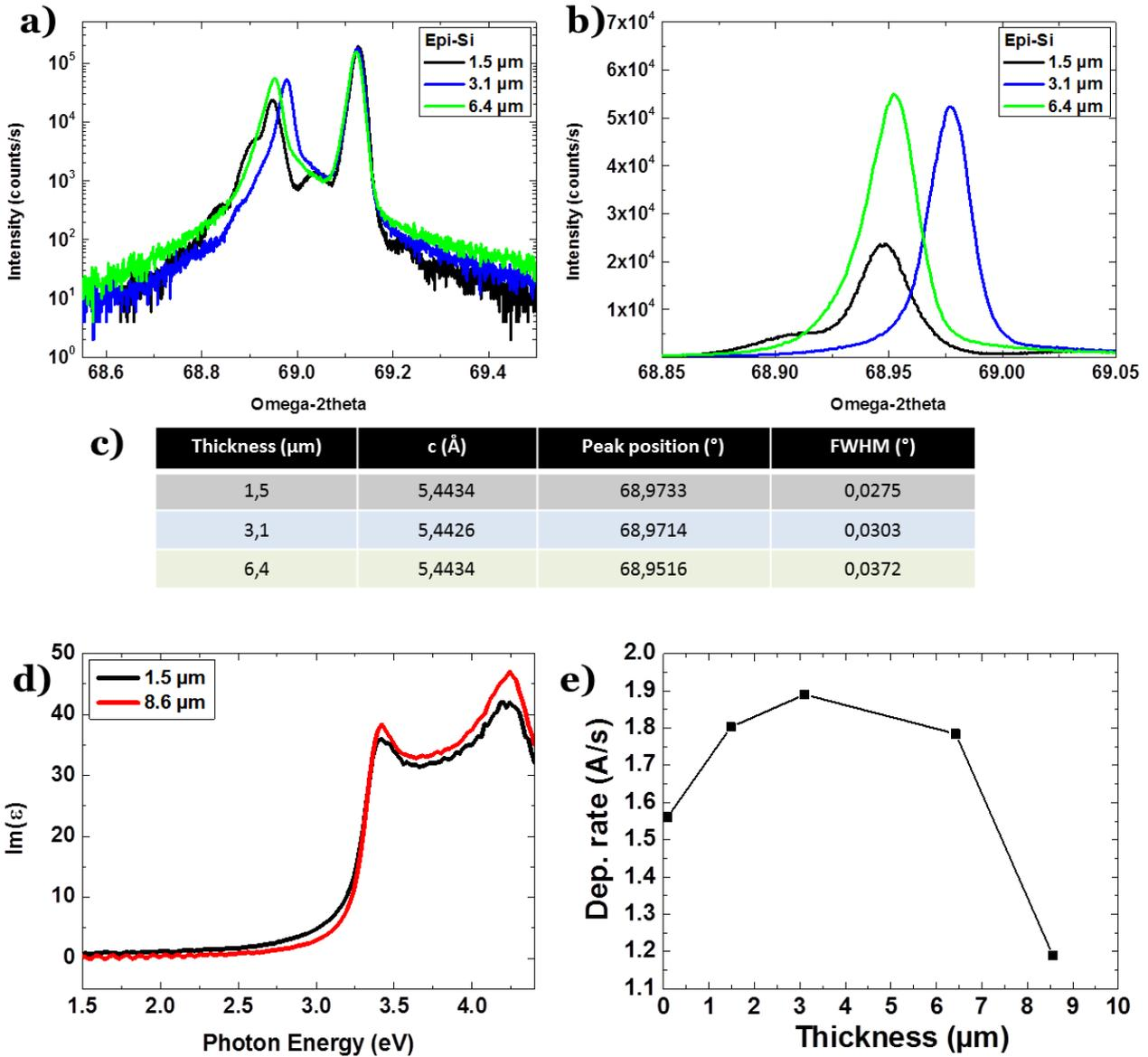
Figure 2.13 - a)  $\omega$ -2 $\theta$  XRD scans of samples with various thicknesses: 1.5  $\mu\text{m}$ , 3.1  $\mu\text{m}$  and 6.4  $\mu\text{m}$ , b) zoom on the epi layer peak in linear scale, c) lattice parameter, peak position and FWHM deduced from XRD data d) ellipsometric spectra of 1.5  $\mu\text{m}$  and 8.6  $\mu\text{m}$  samples, e) evolution of deposition rate as a function of the thickness of the film.
