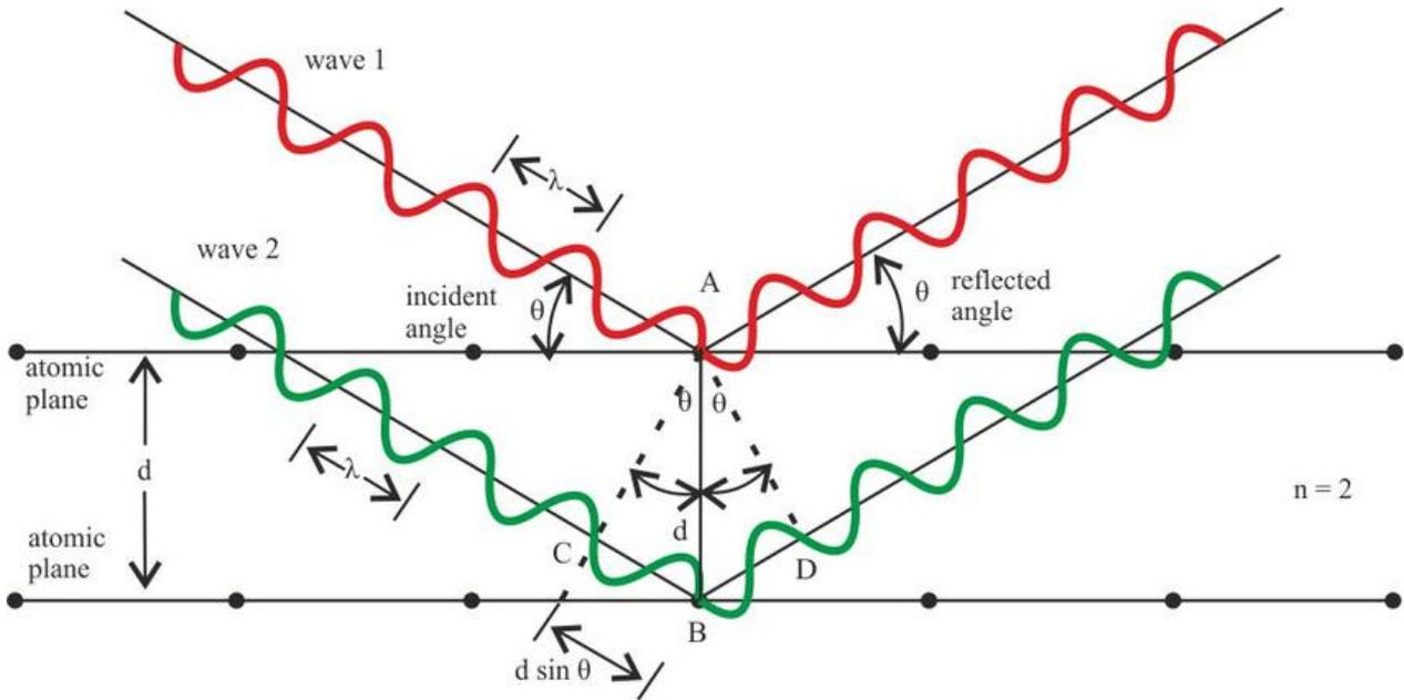
Figure 2.5 - Schematic representation of Bragg's law
