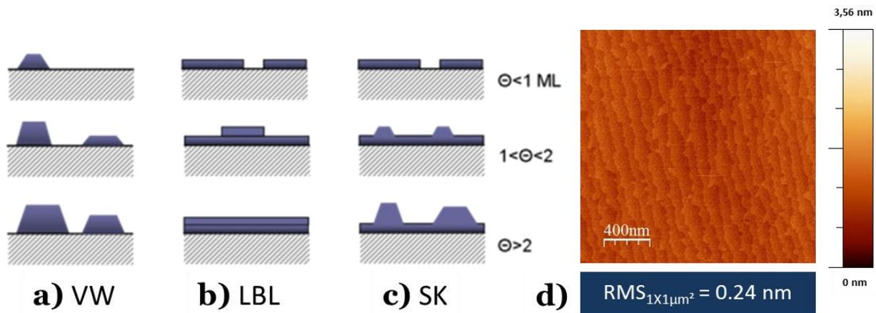
Figure 2.3 - Illustration of the three main growth modes: a) Volmer-Weber mode (VW) b) Frank-van der Merwe mode (Layer-By-Layer) c) Stranski-Krastanov (SK) d) Atomic Force Microscopy mapping of the surface of an GaAs layer grown by MOVPE
