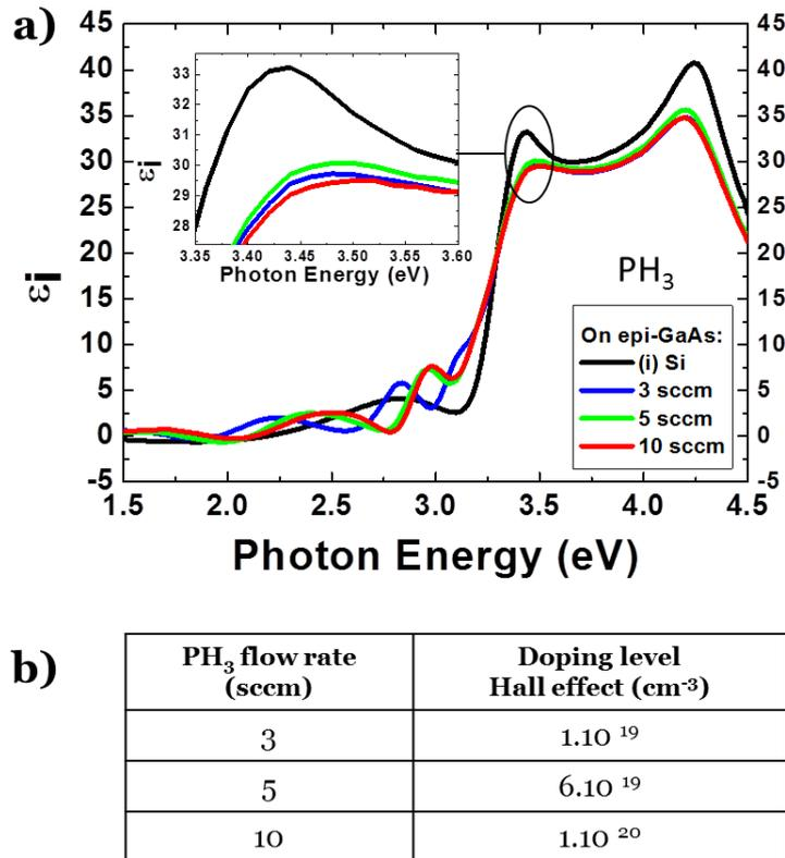
Figure 4.23 - Ellipsometric spectra of silicon thin films grown on epi-GaAs with various PH<sub>3</sub> flow rates
