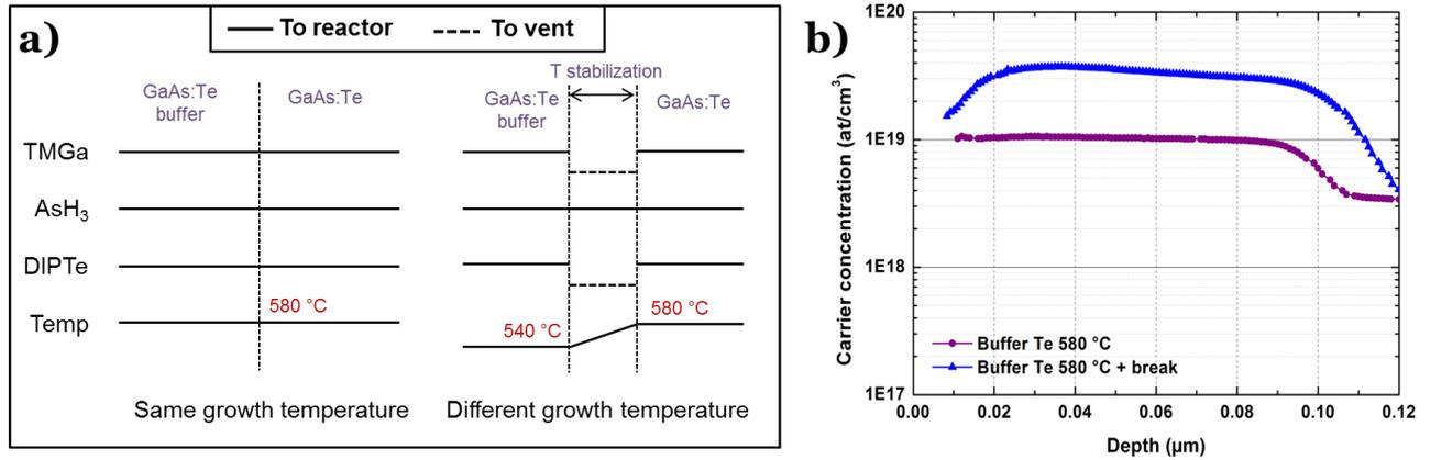
Figure 4.15 - a) Switching sequences of precursors in case of no temperature change (left) and with a temperature change (right) b) Doping profile of the upper doped layer grown directly after the buffer layer (purple circles), and grown after an annealing (blue triangles)
