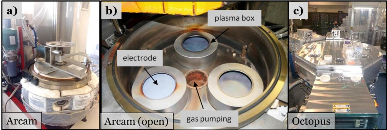
Figure 2.2 - a) Picture of Arcam reactor, b) picture of the inside of Arcam reactor with the three separated plasma boxes. c) picture of the Octopus reactor from IndeoTec.
