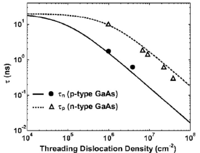
Figure 1.9 - minority carrier lifetime in GaAs as a function of threading dislocation density (Andre et al.<sup>26</sup>)
