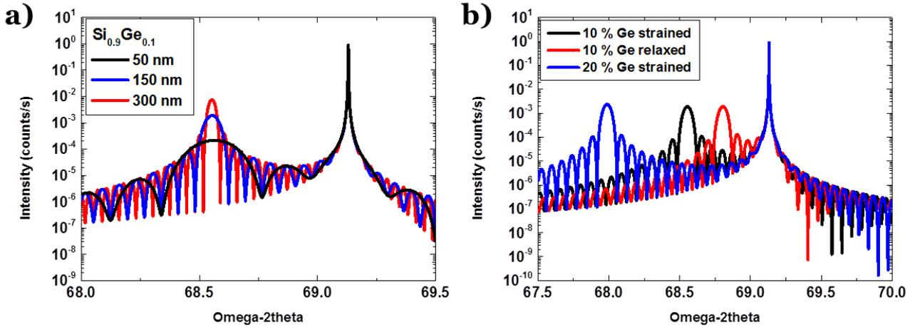
**Figure 2.6 - Simulation with Leptos software of a)  $\text{Si}_{0.9}\text{Ge}_{0.1}$  layer with various thicknesses on a (100) Si substrate: the oscillation period and the peak intensity and FWHM are strongly dependent on the thickness b) Comparison of a strained  $\text{Si}_{0.8}\text{Ge}_{0.2}$  layer with a strained  $\text{Si}_{0.9}\text{Ge}_{0.1}$  and a relaxed one : the peak is shifted to the right when relaxed.**
