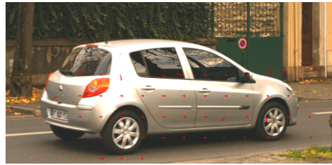
(f) Motion estimation result of (b) with larger block size 32 \times 32
