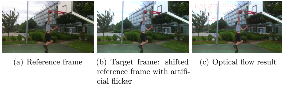
Figure 3.5. Block matching using the mutual information criterion, (b) is the reference frame manually shifted for few pixels, (c) shows motion vectors of blocks from the reference frame to the target frame.
