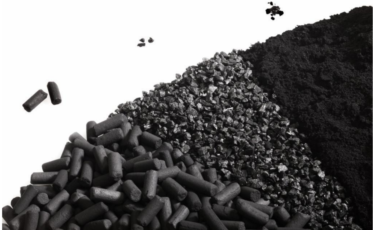
Fig. 20: Shapes of commercial activated carbons [53]
