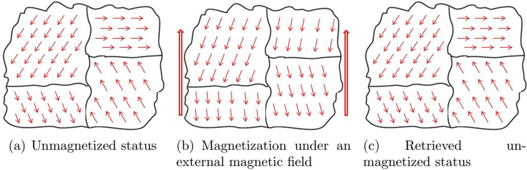
Figure 2.6: Behaviour of dielectric materials when subjected to an external magnetic field.
