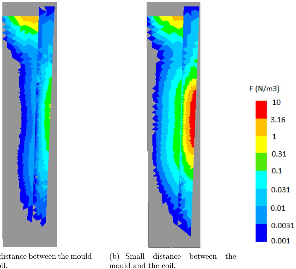
(a) Large distance between the mould and the coil.
