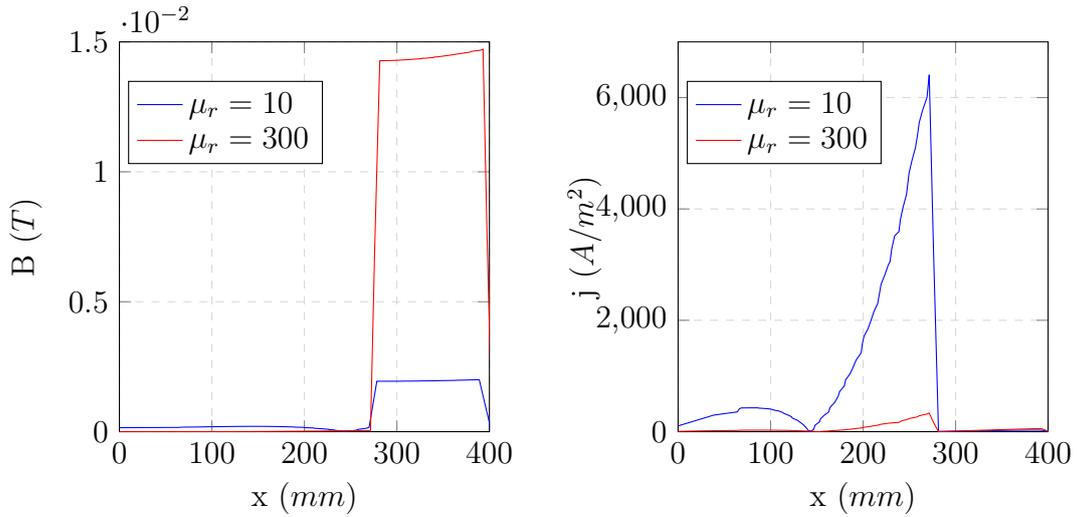
(a) Magnetic flux density vs distance from the mould's centre. (b) Current density vs distance from the mould's centre.
