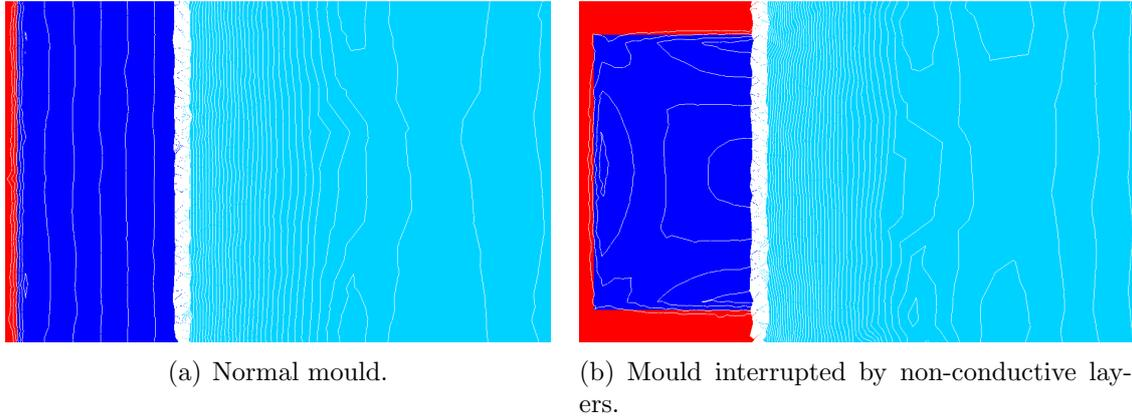
Figure 5.14: Current density isolines in the mould's section.
