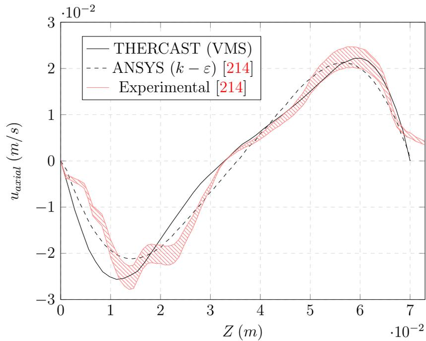
Figure 4.39: Axial velocity with frequency  $h = 150 \text{ Hz}$ .
