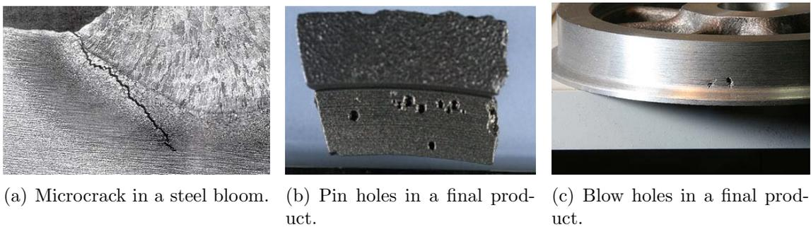
Figure 1.6: Examples of defects in the casting product.
