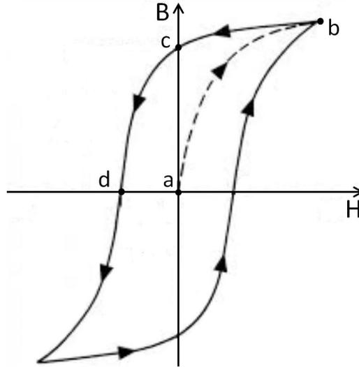
Figure 2.4: Magnetization hysteresis curve for a ferromagnetic material.
