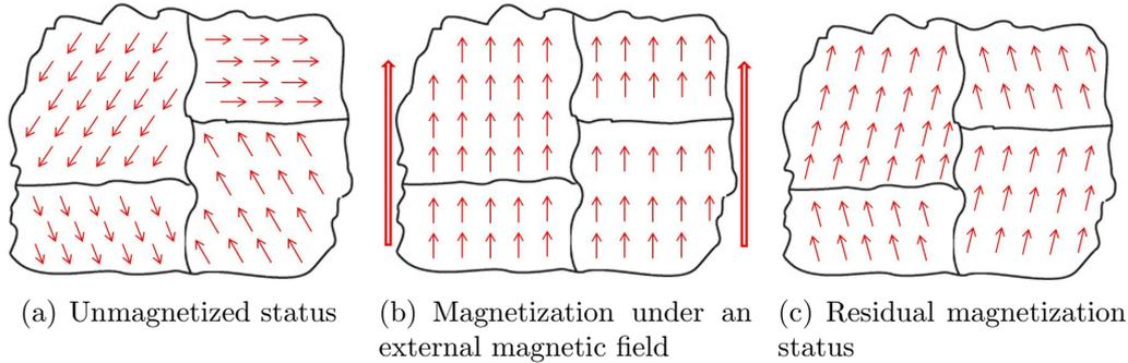
Figure 2.3: Behaviour of ferromagnets when subjected to an external magnetic field.
