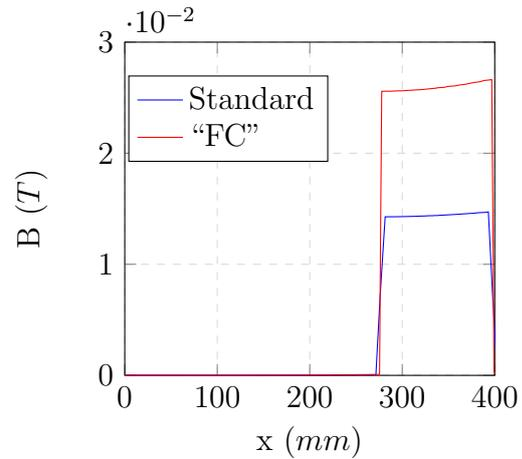
(b) Magnetic flux density vs distance from the mould's centre,  $\mu_r = 300$ .
