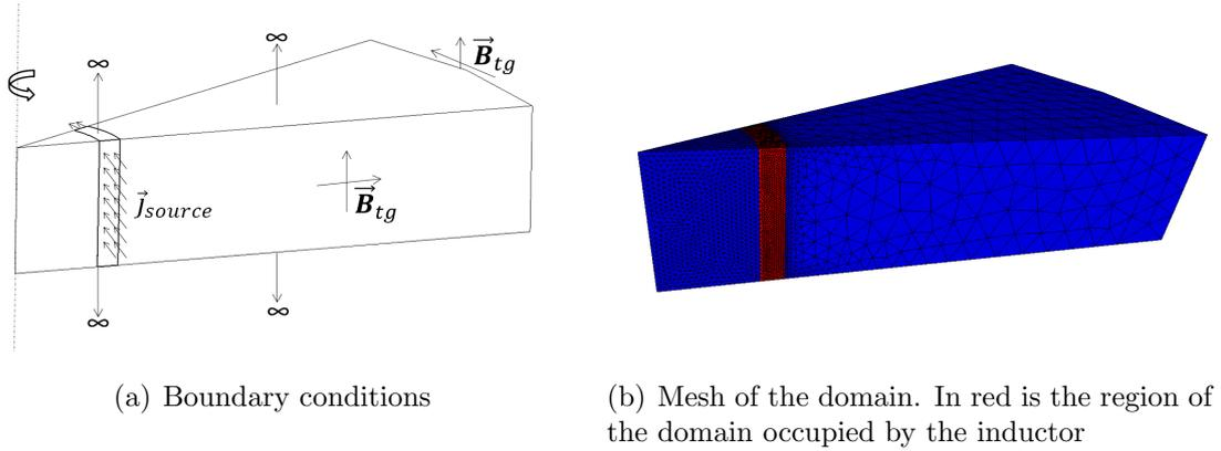
Figure 2.13: Simulation set-up: domain, mesh and boundary conditions
