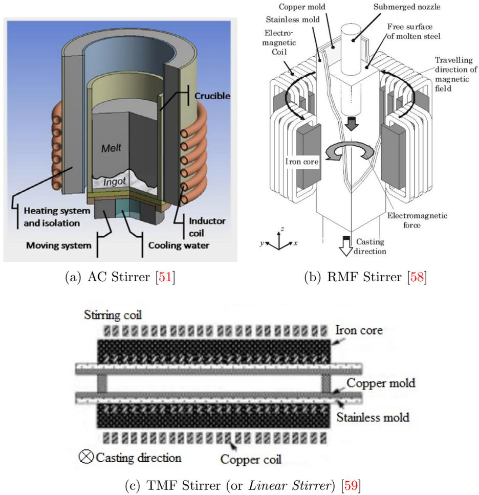
Figure 1.9: Different types of electromagnetic stirrers.
