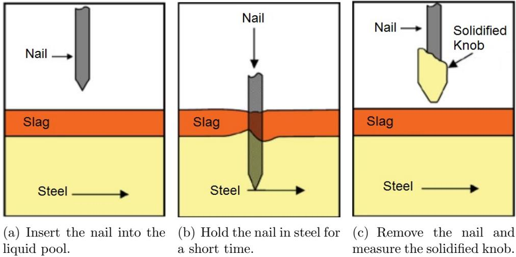
Figure 1.7: Procedure for the nail board test [33].
