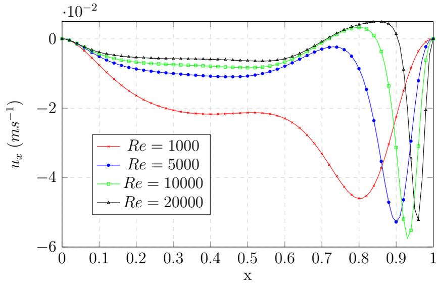
Figure 4.13:  $u_x$  plot over the center-line  $y = 0.5$  at different  $Re$  and  $N = 1.785$ .
