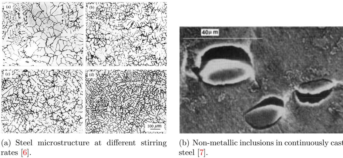
Figure 1.5: Microscopic structure and inclusions in steel.
