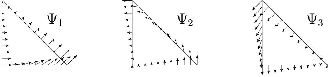
Figure 2.12: Edge base functions for the 2D element.
