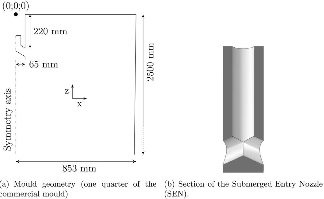
Figure 5.1: Geometrical features of the simulated process.
