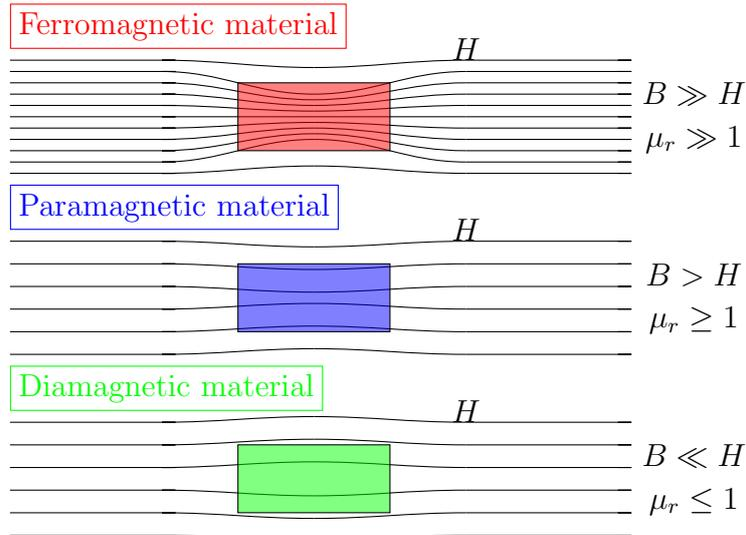
Figure 2.7: Comparison between the magnetic behaviour of material at a different magnetic state.
