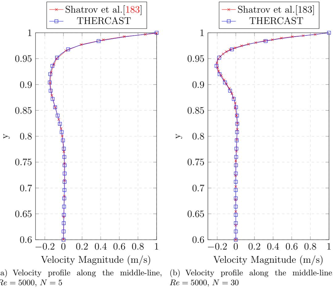
Figure 4.4: Velocity profile along the middle-line: validation.
