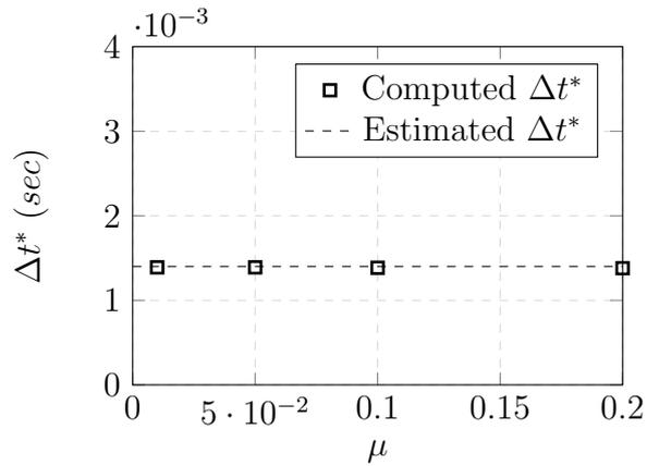
(e) Critical time-step variation at different material's viscosity
