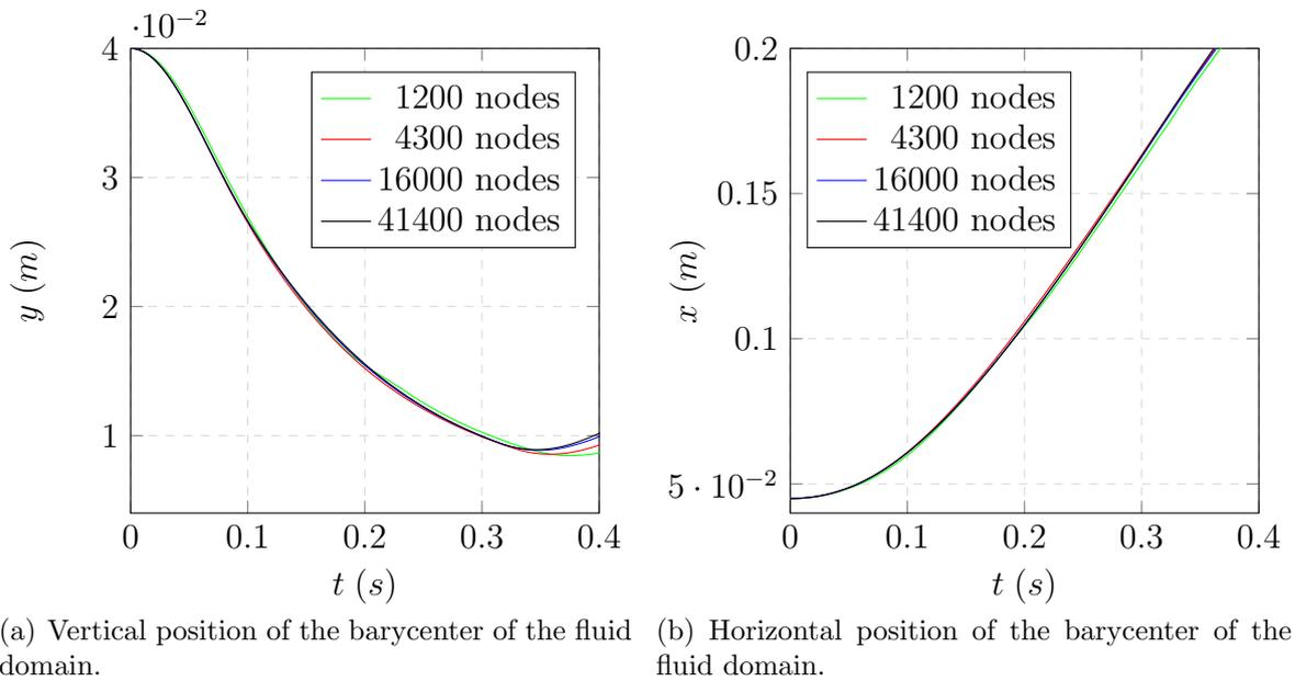
Figure 4.27: Barycenter position evolution at different mesh-refinement levels.
