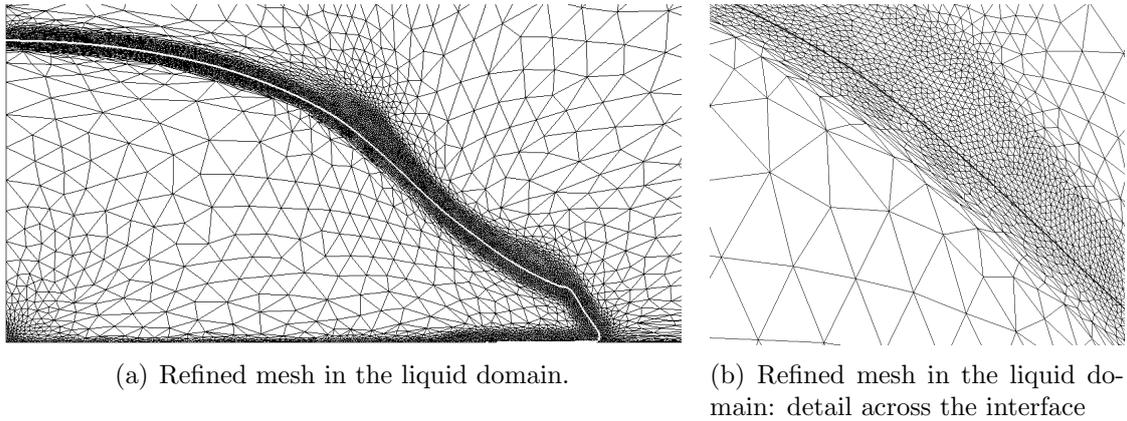
Figure 4.26: Anisotropic, unstructured mesh.
