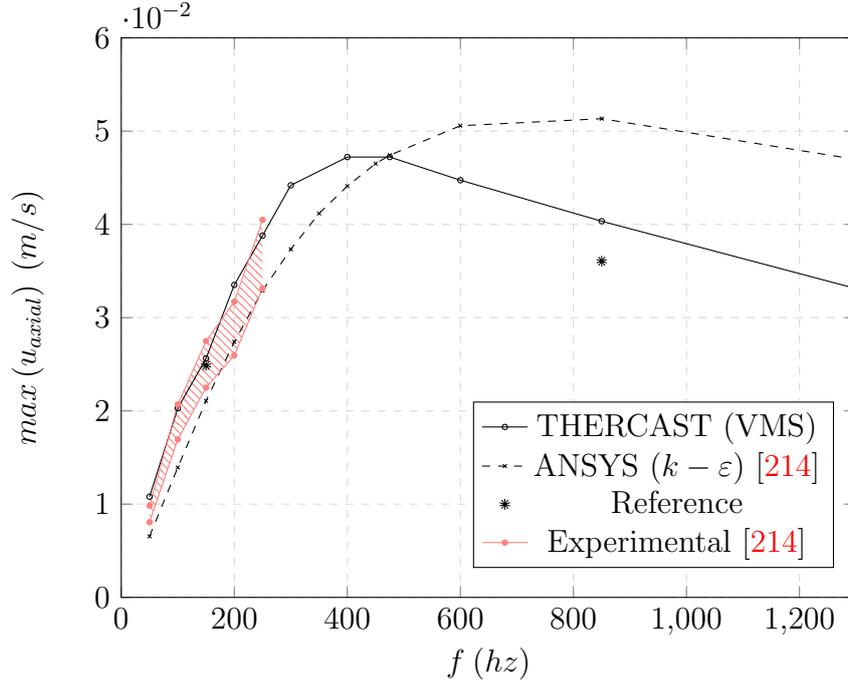
Figure 4.40: Maximum axial velocity at different frequencies.
