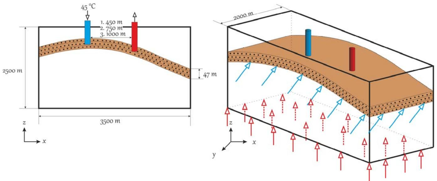
**Fig. 4.10.** Schematic drawing of the doublet model. Red and blue arrows indicate the direction of heat flow and movement of groundwater, respectively.
