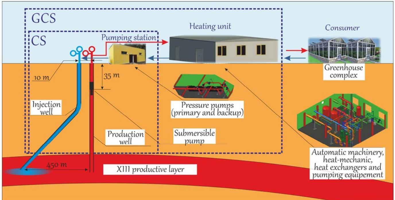
**Fig. 6.3.** The Khankala geothermal station with circulation scheme of heat extraction schematic drawing [Zaurbekov et al., 2015]
