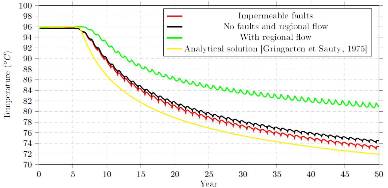
**Fig. 4.13.** Temperature in production well decrease (450 m distance between production and injection well bottoms)
