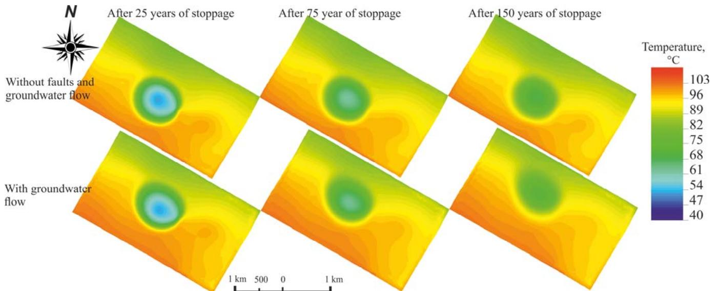
**Fig. 4.17.** The XIII productive layer of the Khankala geothermal waters deposit temperature change after 50-years exploitation stoppage: after 25, 75 and 150 years (450 m distance between production and injection well bottoms)
