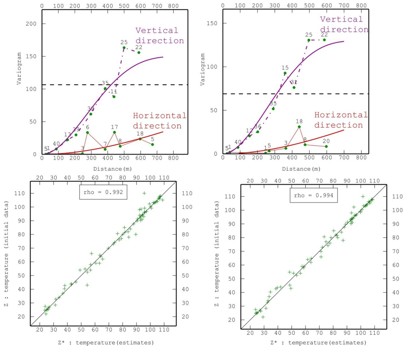
**Fig. 3.18.** Variogram models and the results of cross-validation for normal coordinate system (left) and the XIII layers top as the basis (right)
