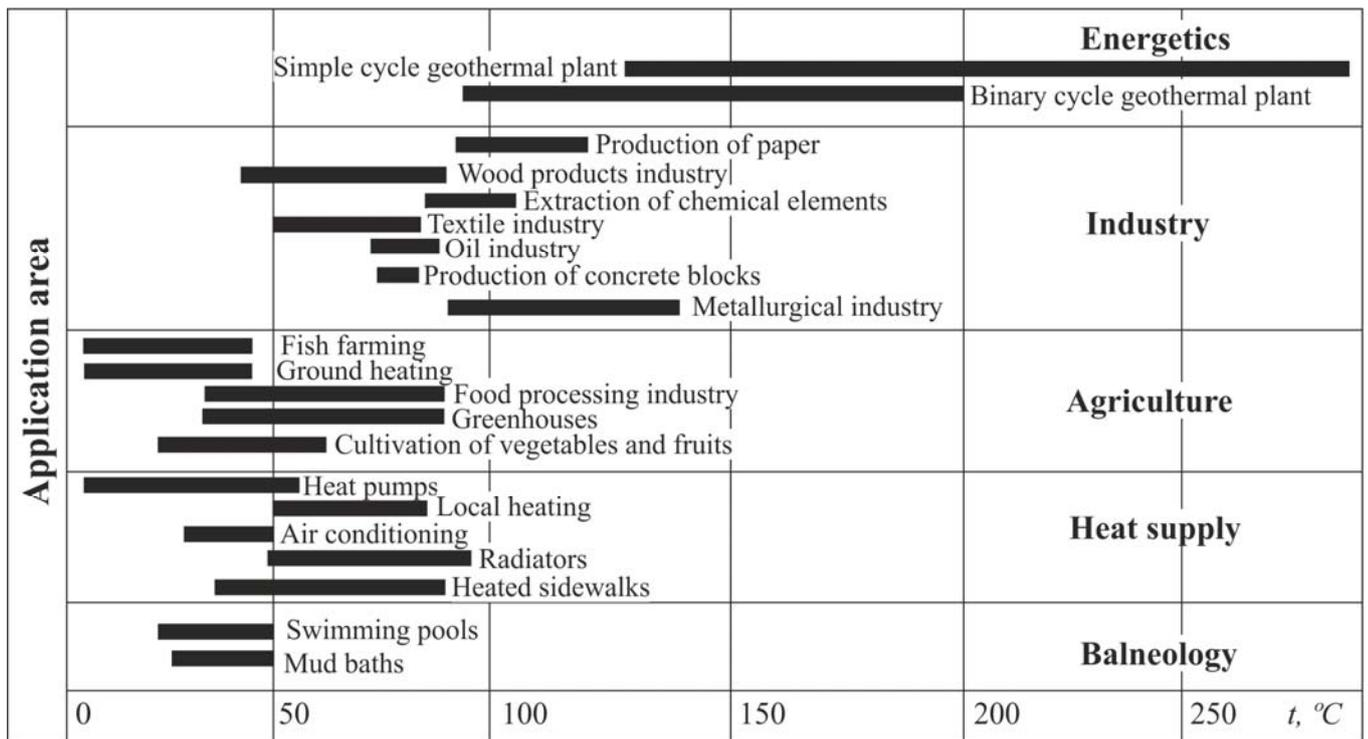
Fig. 1.1. Geothermal waters of different temperatures use [Povarov, 2003]
