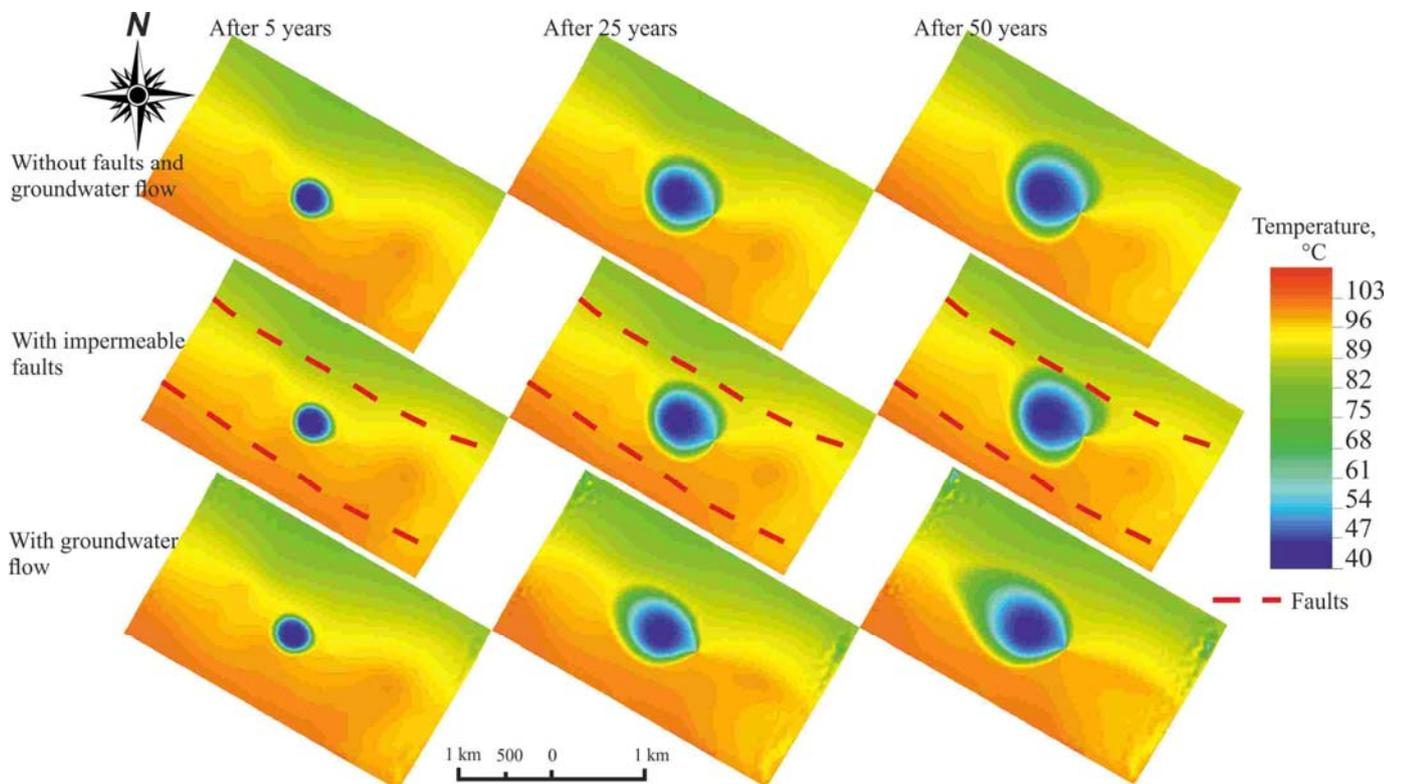
**Fig. 4.14.** The results of the modelling: temperature evolution in the XIII layer (450 m distance between production and injection well bottoms)
