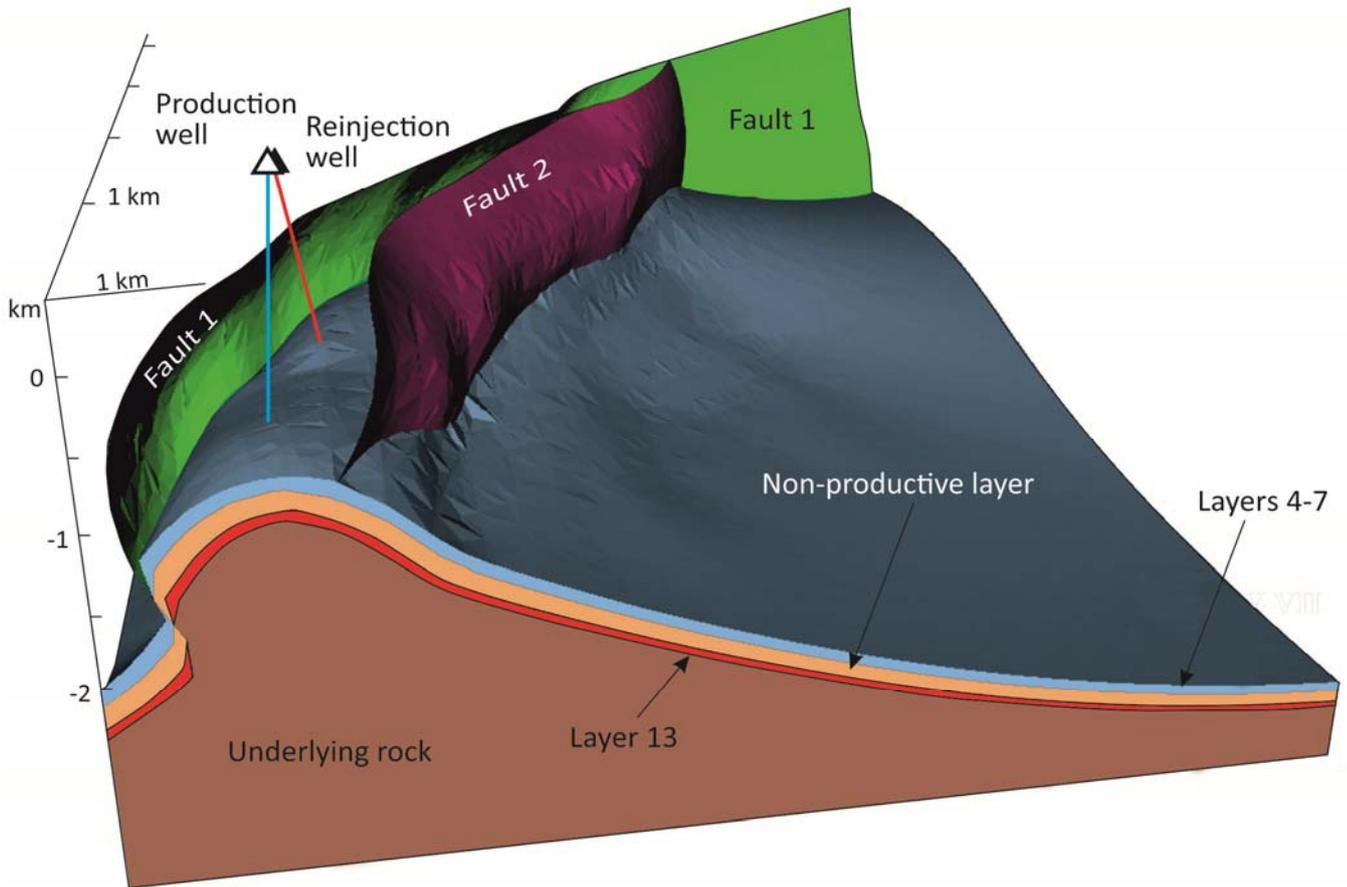
**Fig. 2.4.** The Khankala geothermal waters deposit 3-D geological model
