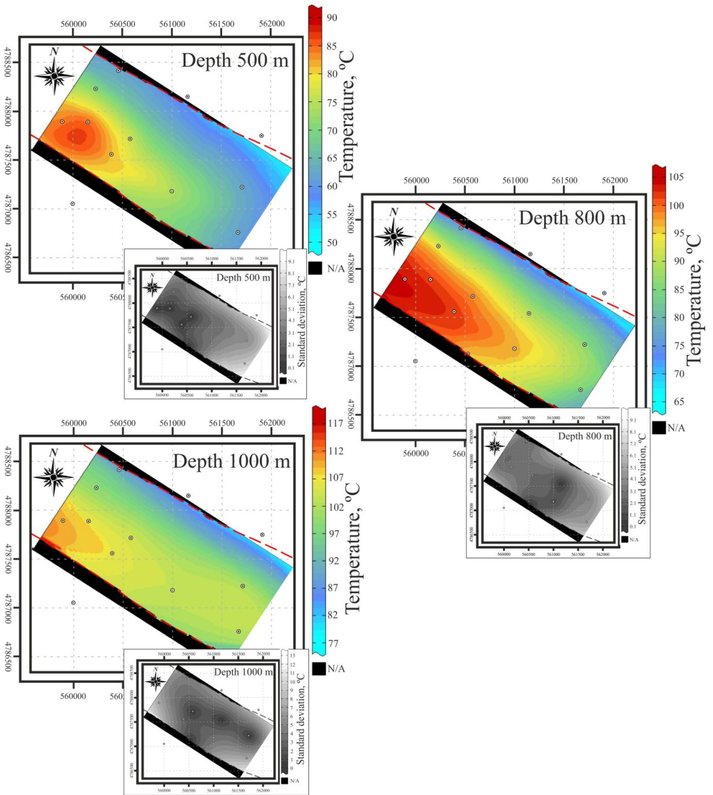
**Fig. 3.21.** Cross-sections of final estimation of the temperature distribution and its standard deviation on the 3D block
