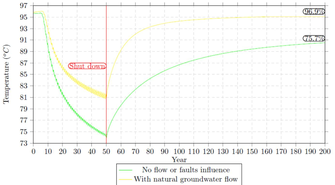
**Fig. 4.16.** Production well temperature for 50 year exploitation and then shut-down scenario (450 m distance between production and injection well bottoms)
