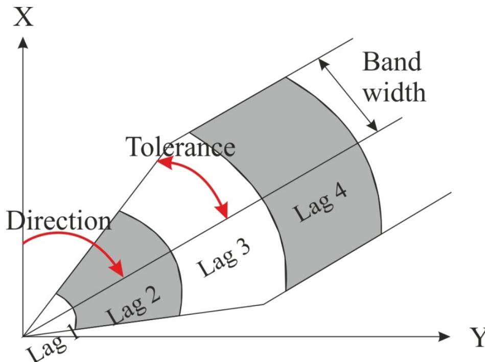
**Fig. 3.6.** Parameters of directional variogram
