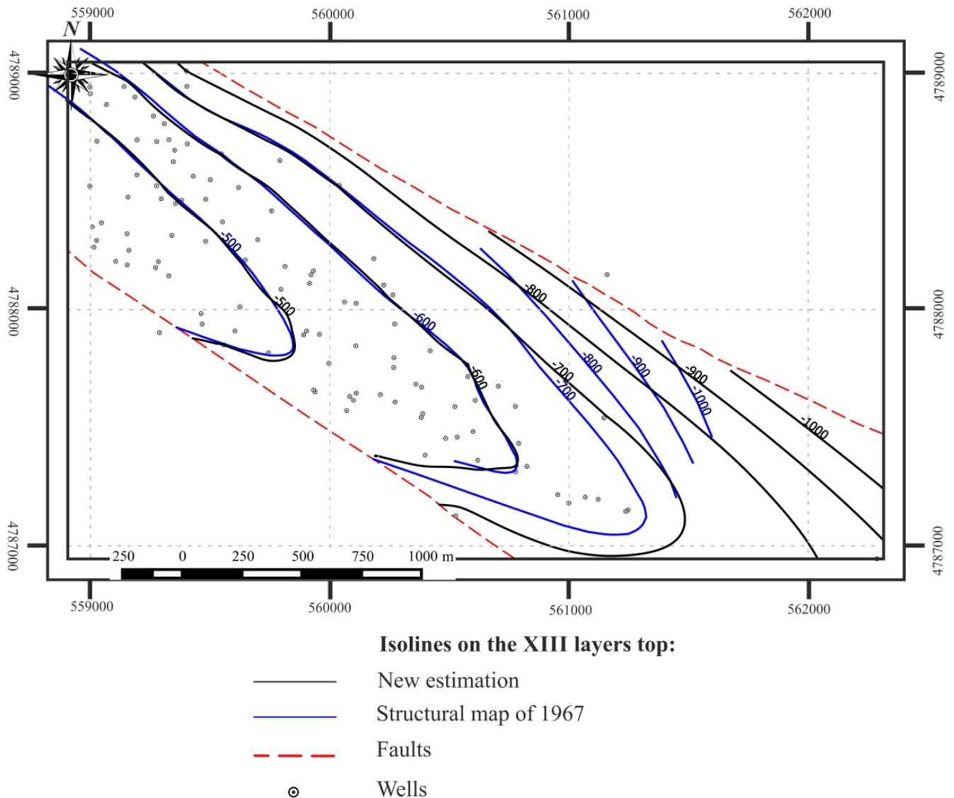
**Fig. 3.12.** Comparison of old and new structural maps of the top of the XIII layer
