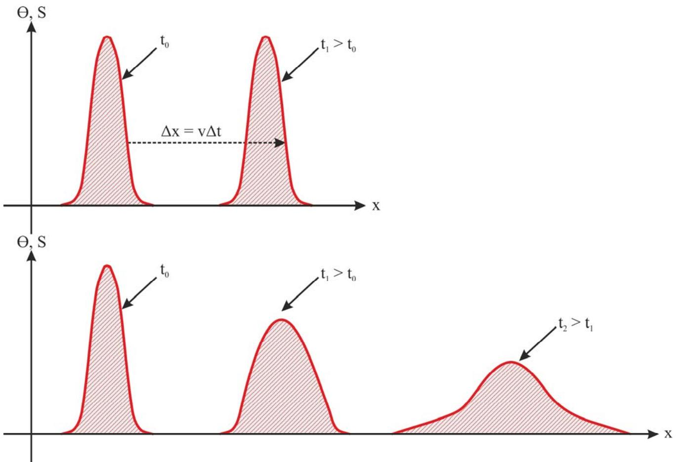
**Fig. 4.7.** Advection (top) and dispersion (bottom) processes in one dimensional example [Pruess, 2002]
