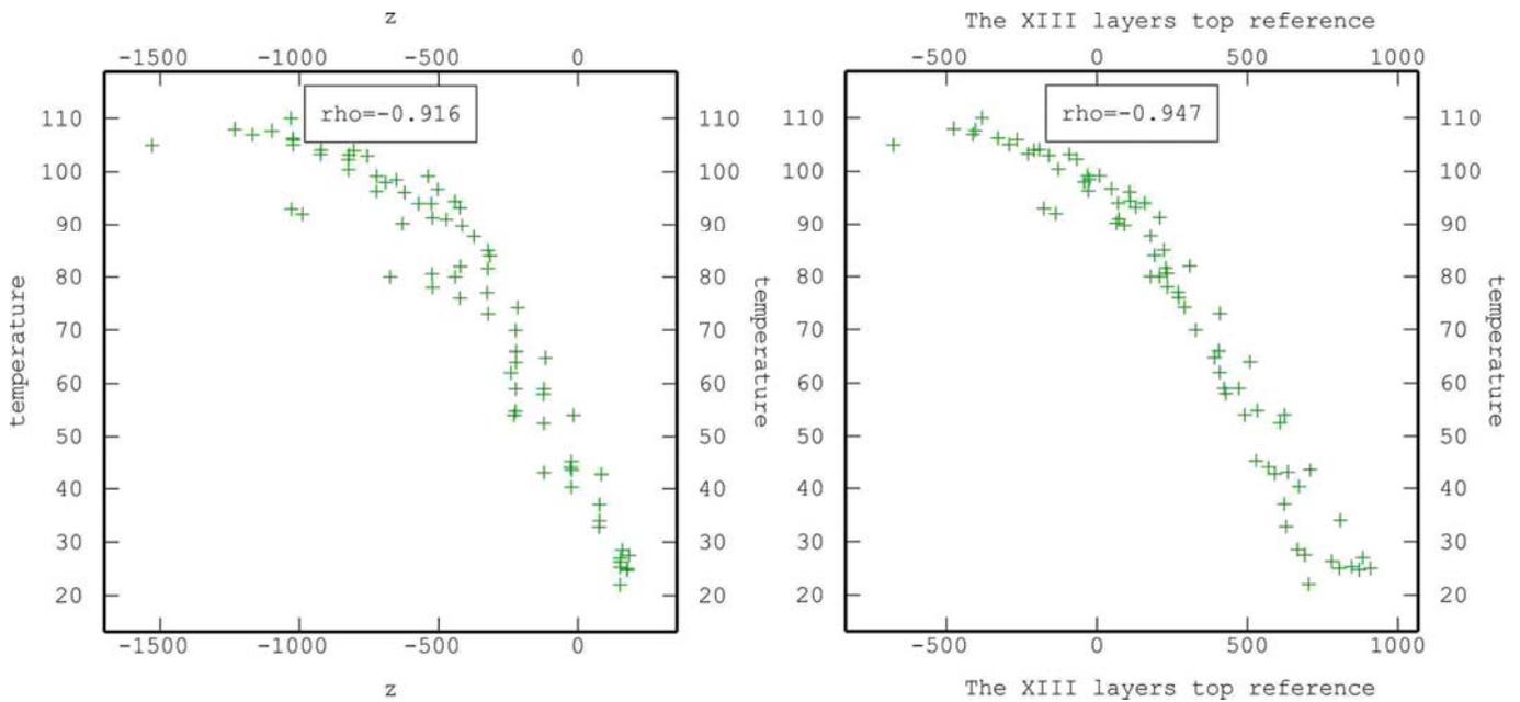
**Fig. 3.16.** Scatter-diagrams of the temperature versus depth in cases of two different reference planes
