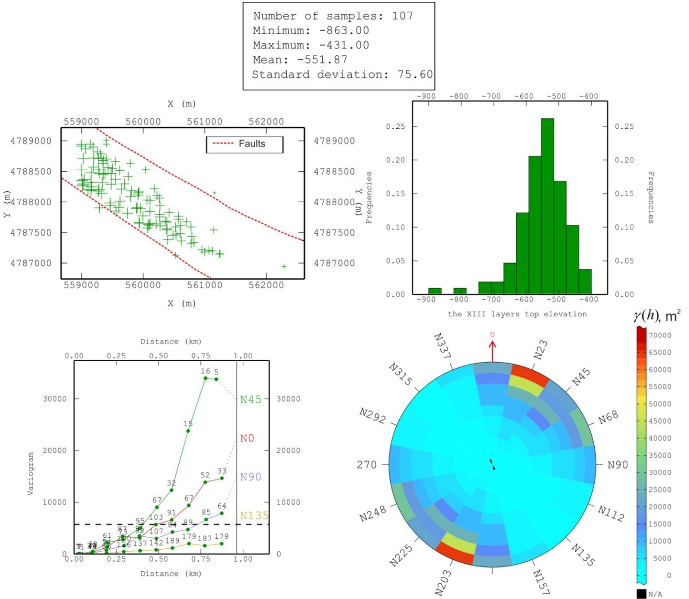
**Fig. 3.7.** Statistical assessment and directional sample variograms calculation (statistics, initial data location, histogram, directional variograms and variogram map)
