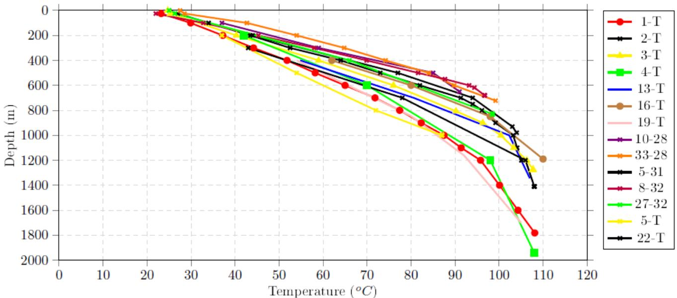
**Fig. 3.13.** Temperature measurement within the Khankala deposit of geothermal waters
