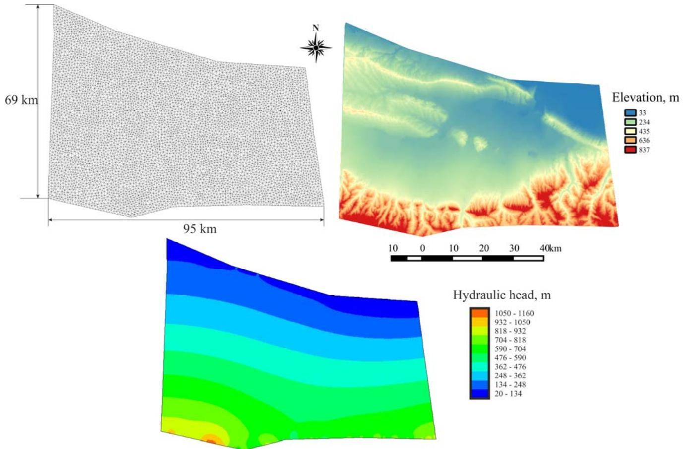
**Fig. 4.6.** Mesh, territory elevation and modelling results
