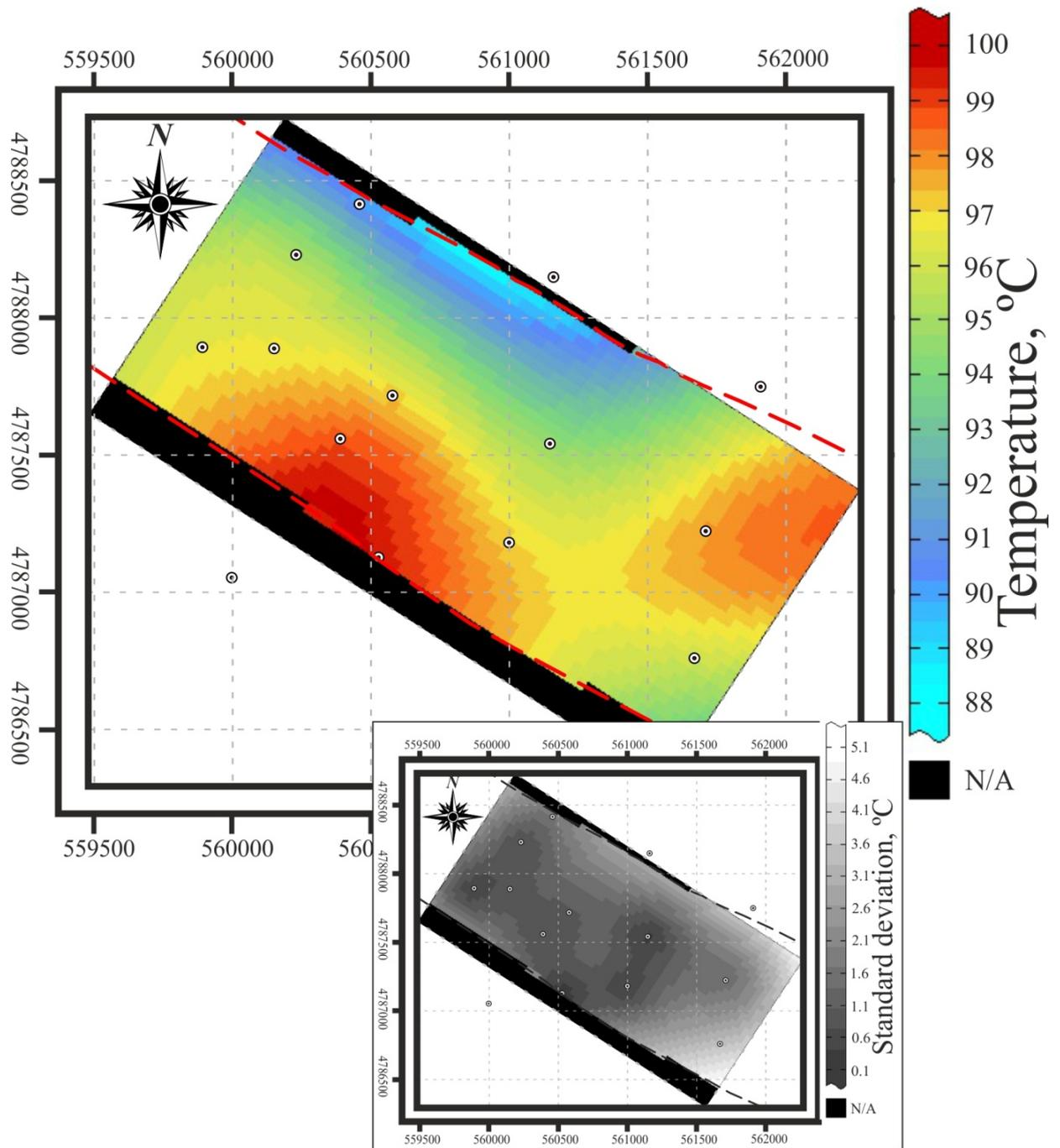
**Fig. 3.22.** Temperature within the XIII layer and kriging standard deviation
