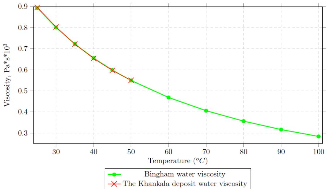
**Fig. 4.11.** Changes in water viscosity depending on the temperature according to Bingham and laboratory analysis
