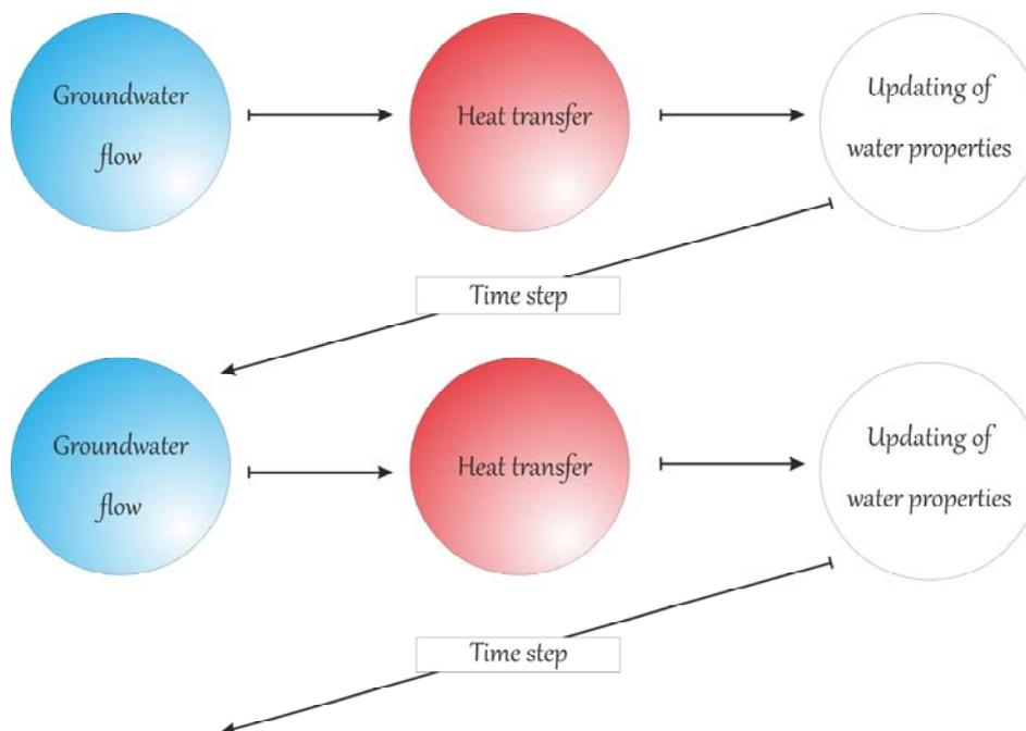
**Fig. 4.12.** Coupled processes of groundwater flow and heat transport
