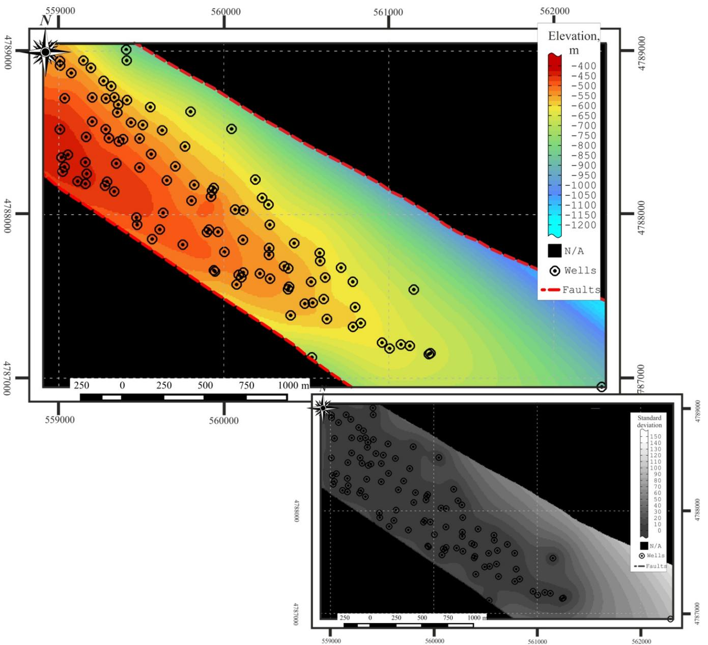
**Fig. 3.11.** Estimation of the elevation of the XIII layer and associated standard deviation
