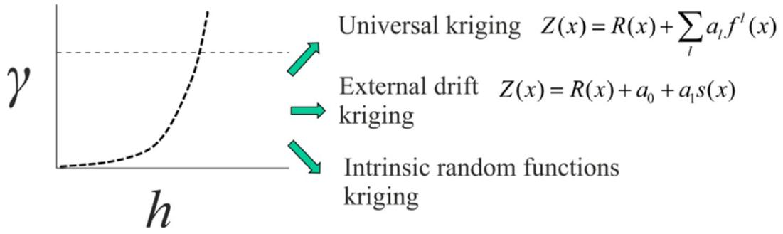
**Fig. 3.8.** Types of kriging used for non-stationary data
