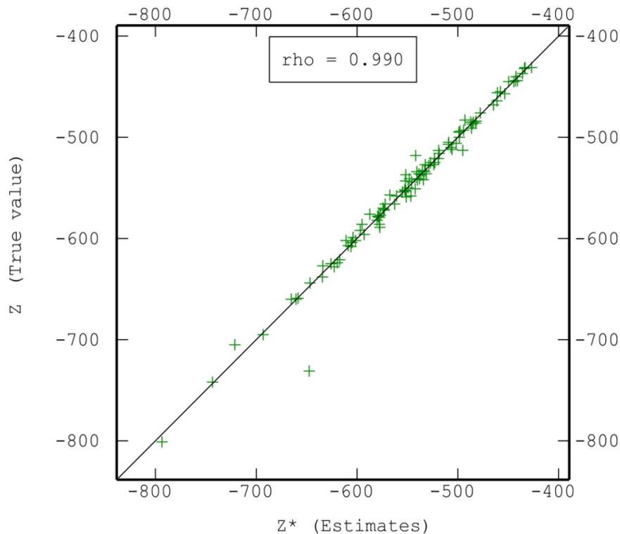
**Fig. 3.10.** Cross-validation of the model for the estimation of the XIII layer top elevation
