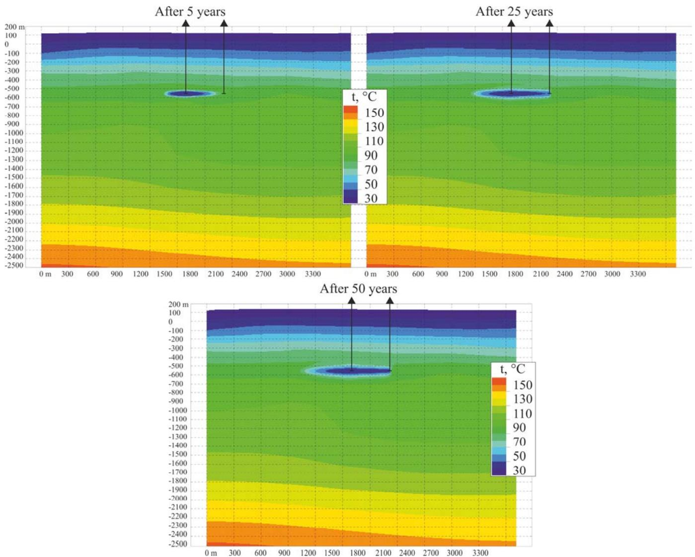
**Fig. 4.15.** The results of the modelling: temperature evolution in the XIII layer (side view, 450 m distance between production and injection well bottoms)
