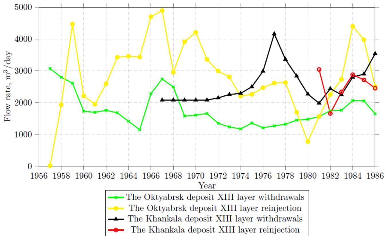
**Fig. 1.3.** The XIII layer production and reinjection [Krylov, 1987f]
