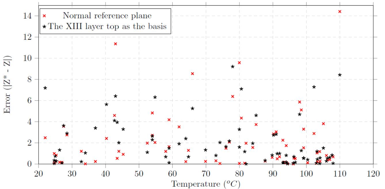
Fig. 3.19. Absolute errors for normal and modified coordinate systems
