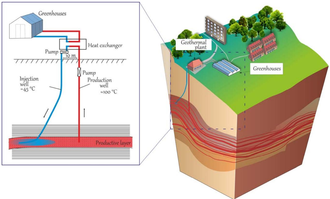
**Fig. 2.9.** Schematic drawing of the Khankala deposit geothermal circulation system (doublet)
