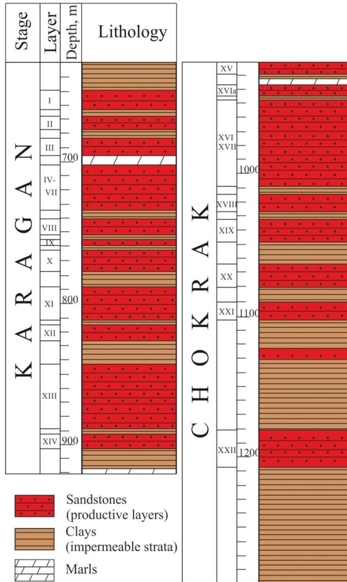
**Fig. 2.2.** Averaged section of the productive Karagan-Chokrak sediments at the Oktyabrsk anticline south-eastern dipping [Shpak, 1968f]
