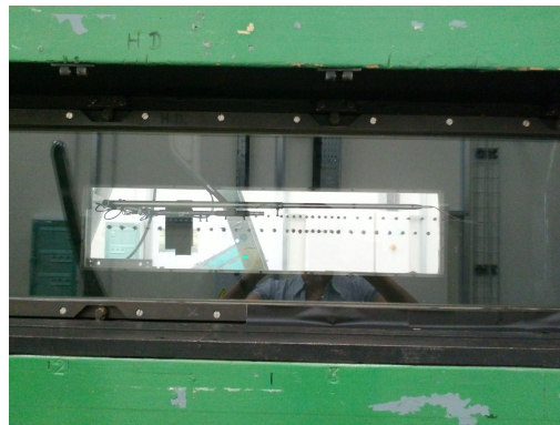
Figure 3.2. Prandtl antenna mounted on the travel system in the wooden test section.
