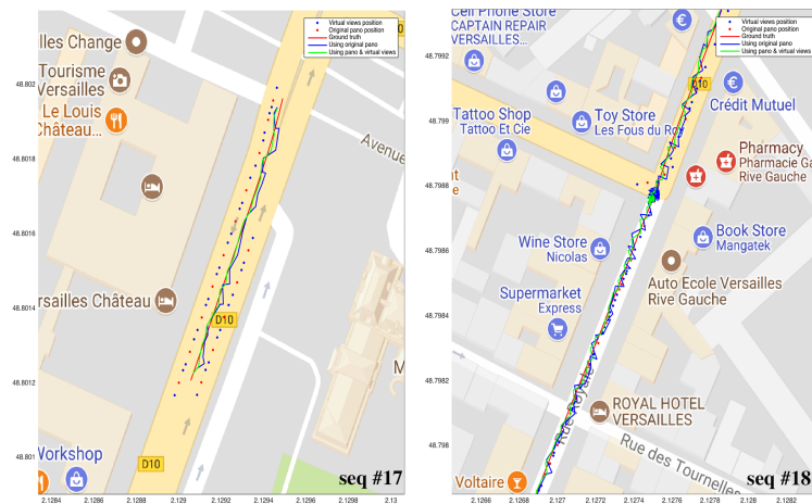
Figure 7.24: The localization output from sequences No.17 and 18 using original Street Views and synthesized virtual views. The positions of original panorama, virtual views and ground truth are noted in red points, blue points and red line respectively. The results from original Street Views and augmented virtual street views are in blue and green lines.
