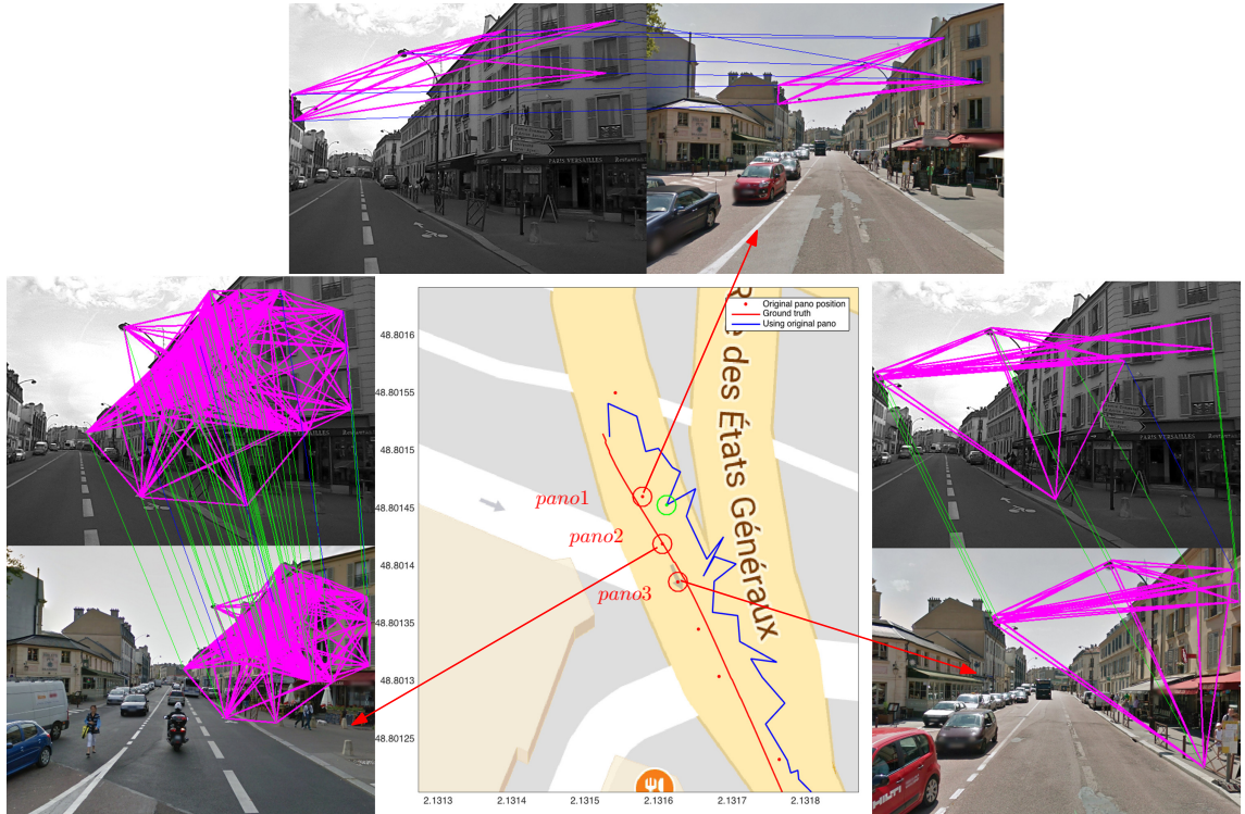
Figure 7.11: An example of 2 pairs of validated matches between a monocular image and its retrieved Street View images by kVLD descriptors. The positions of Street Views and the estimated localization are displayed in red and green circles respectively. kVLAD matches verified by ORSA are the green lines and those verified by graph matching are the blue lines.
