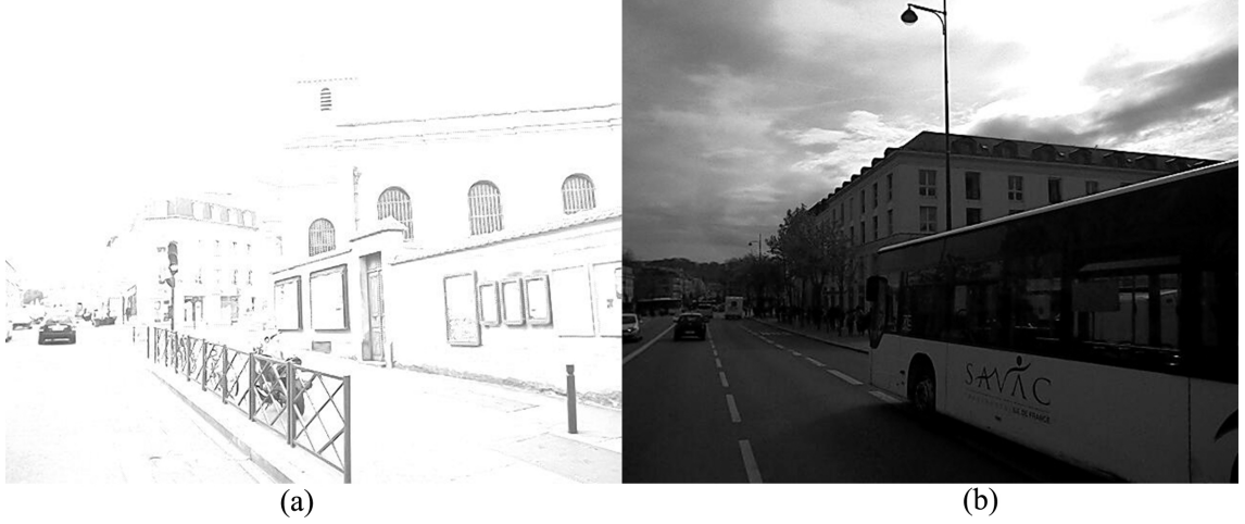
Figure 7.20: Some scenarios during localization: (a) Some big brightness blur frames were often captured in the initial step and they are ignored by our algorithms. (b) Noise from moving objects appears frequently in the urban environment.
