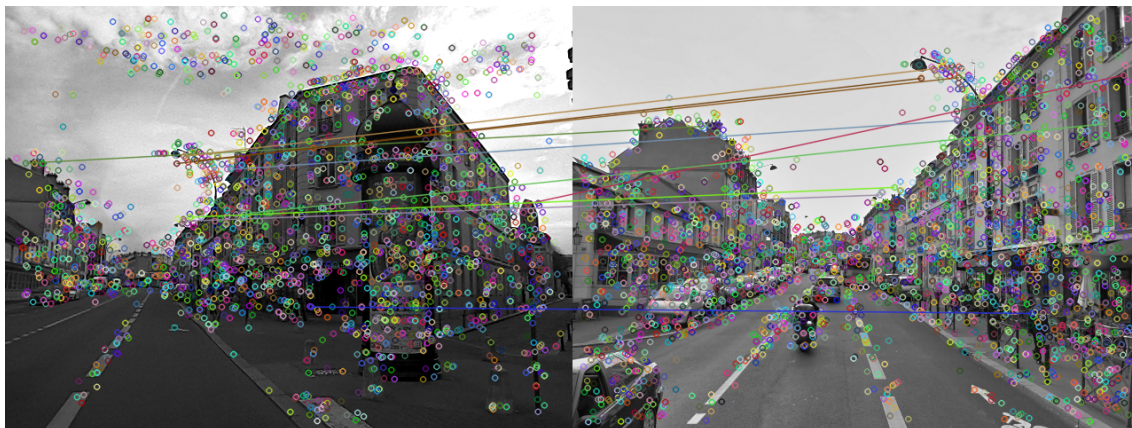
Figure 6.18: Final inliers detected by the SURF-SURF feature in Scenario #2. A lot of matches are detected but there are still false matches.
