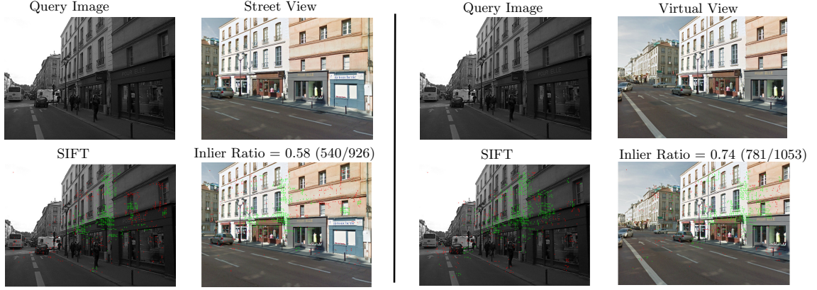
Figure 7.19: The same query image is matched with highly similar Street View retrieved by the BoW and with corresponding virtual view. The FLANN based matches are displayed in red and geometrically verified matches are shown in green. The inlier ratio is measured by proportion of geometrically verified matches.
