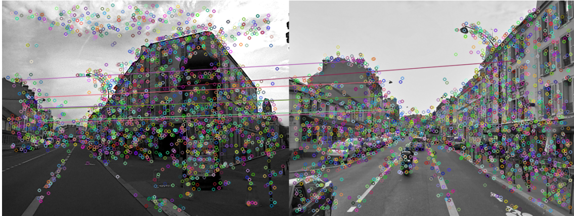
Figure 6.15: Final inliers detected by the SURF-SIFT feature in Scenario #2. SURF-SIFT still performs well for big different viewpoint but the detected number is small.
