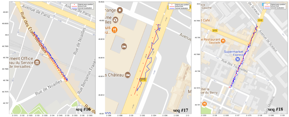
Figure 9.24: The localization output from sequence No. 16, 17 and 18 obtained by the convnet method. The original panorama position, the ground truth and the convnet results are noted in red point, red line and blue line respectively.
