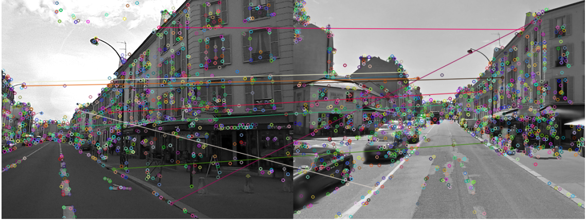
Figure 6.8: FLANN matching with SIFT features after ratio test, symmetric check and 8-point RANSAC selection.
