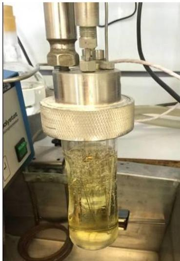
**Figure 2-8**View of the dilutor cell after introducing  $\text{CS}_2$
