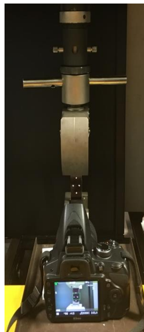
Fig. IV.2: Measurement system of composite tensile tests
