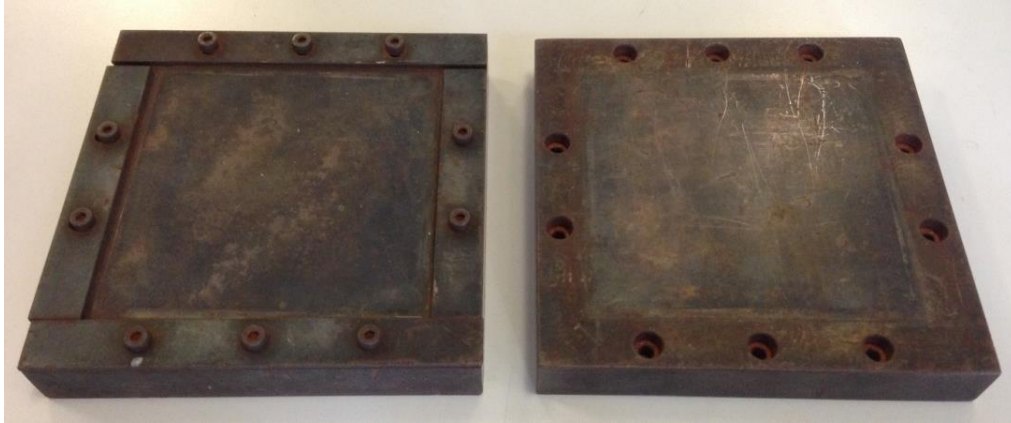
Fig. II.3 : Casing for the PEKK plates crystallization
