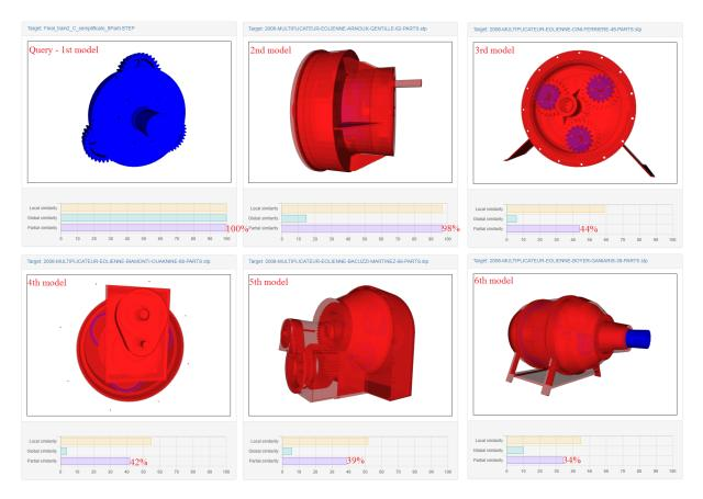
Figure 6.16: Retrieved models ordered according to the partial similarity criteria for the query model in Figure 6.15
