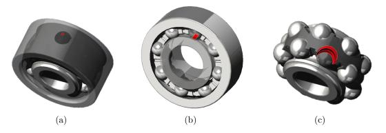
Figure 4.17: Examples of volumetric intersections of spherical parts
