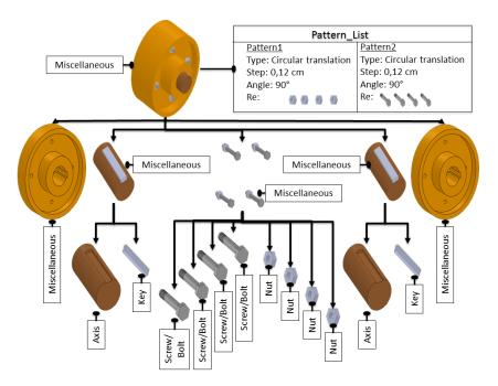
Figure 4.6: Example of structure layer of the EAM of an assembly model with its attributes
