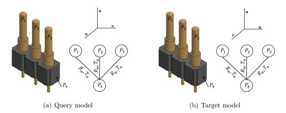
Figure 5.6: Example of the same object embedded in two different reference frame
