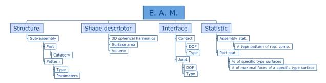
Figure 5: The multi-layered Enriched Assembly Model
