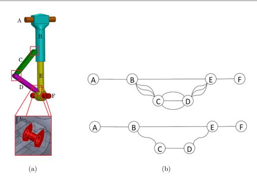
Figure 4.19: Assembly model example (a) and the reduction of its kinematic chain (b)
