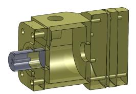
(b) Gear pump model with simplified components
