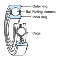
Figure 4.12: Bearing component and its constituting elements.
