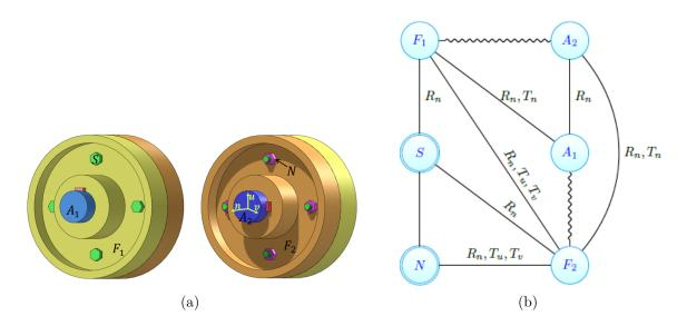
Figure 4.29: Example of a CAD model (a) and a part of its EAM descriptor (b)
