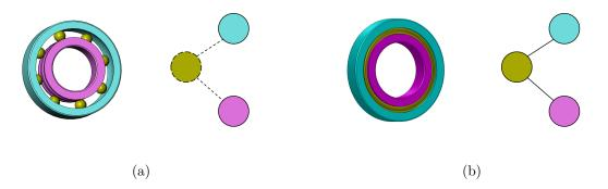
Figure 4.26: Abstract bearing definition (a) Bearing with ball pattern; (b) bearing with idealized pattern
