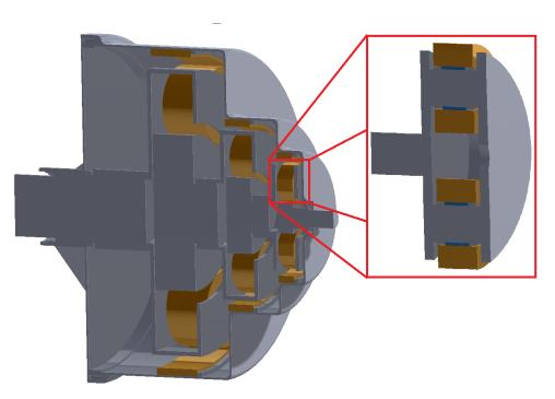
Figure 1.16: Gears and bearings embedded in their context of use
