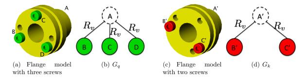
Figure 5.3: Example of two assembly models and their EAM attributed multi-graphs  $G_q$  and  $G_k$ .
