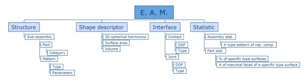
Figure 4.1: The multi-layered Enriched Assembly Model
