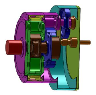
Figure 1.4: A DMU geometry of a wind turbine speed reducer
