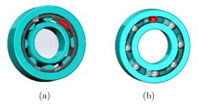
Figure 4.25: Example of different type of contacts between cage and rolling elements
