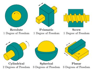
Figure 1.8: Lower kinematic pairs [6]
