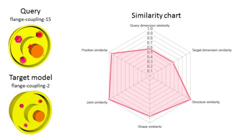
(a) Example of matching inspection for the third model in Figure 6.7 using the equation 6.4 as joint compatibility
