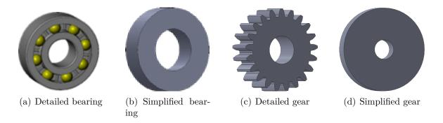
Figure 4.24: Examples of components with different shapes and functions
