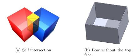
Figure 1.5: Configurations not allowed
