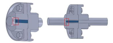
Figure 6.13: Different contacts between the key and the shaft of the query (left) and target (right) assembly models
