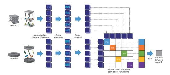
Figure 2.2: Example of the procedure to compute the distance in terms of shape and structure between two assembly models (Figure 5 in [61])
