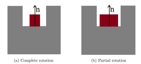
Figure 4.9: Models with same contacts and DOF but different allowed motions
