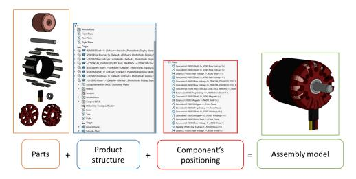
Figure 1.6: Assembly model of an electrical engine
