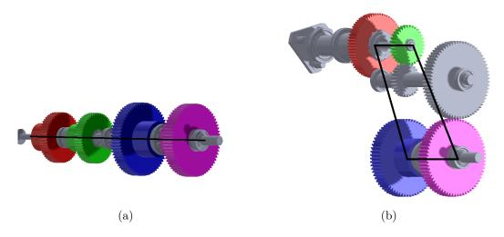
Figure 5.9: Example of assembly models with similar parts arranged in different configurations
