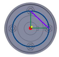
Figure 4.4: Example of attributes of a circular pattern
