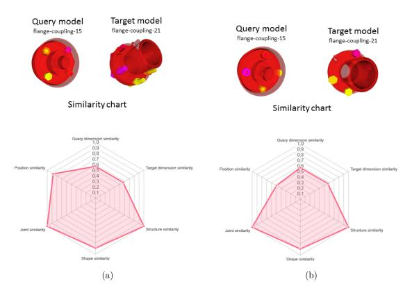
Figure 6.10: Two different results for the fourth model in Figure 6.7 where the arrangement of the parts is different and detected by different values of the position measure
