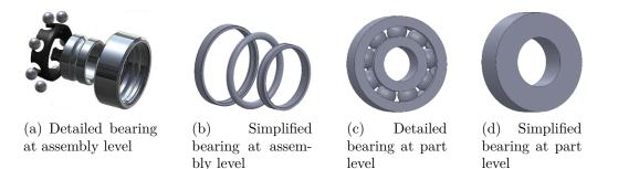
Figure 27: Examples of bearing components with different representations and resolutions
