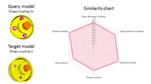
(b) Example of matching inspection for the third model in Figure 6.7 using the equation 5.1.8 as joint compatibility
