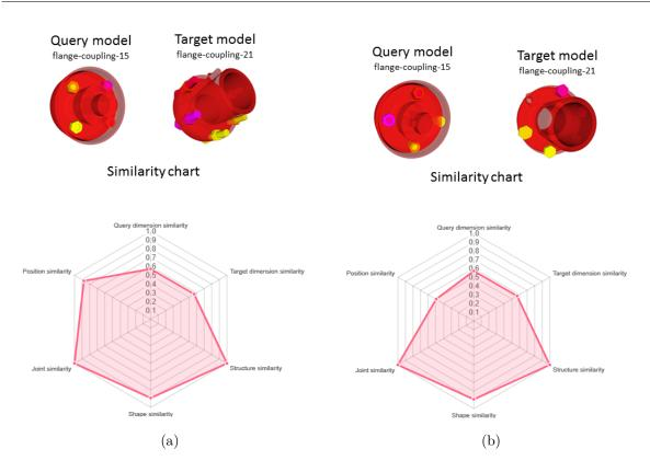
Figure 23: Two different results for the fourth model in Table 4 where the arrangement of the parts is different and detected by different values of the position measure
