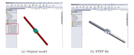
Figure 1.14: Example of information loss storing a model in STEP 214 format
