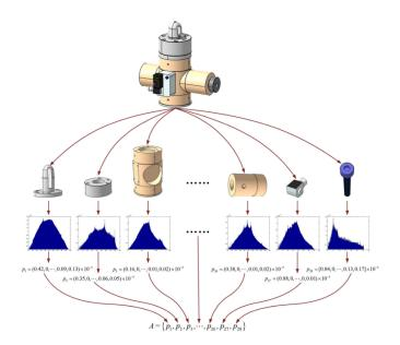
Figure 2.3: Example of the description of an assembly model (Figure 3 in [125])
