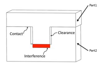
Figure 1.10: Interface relations between parts in an assembly model
