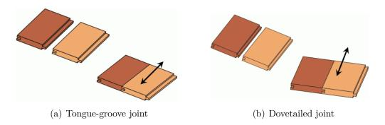
Figure 4.10: Same joint generated by different contacts
