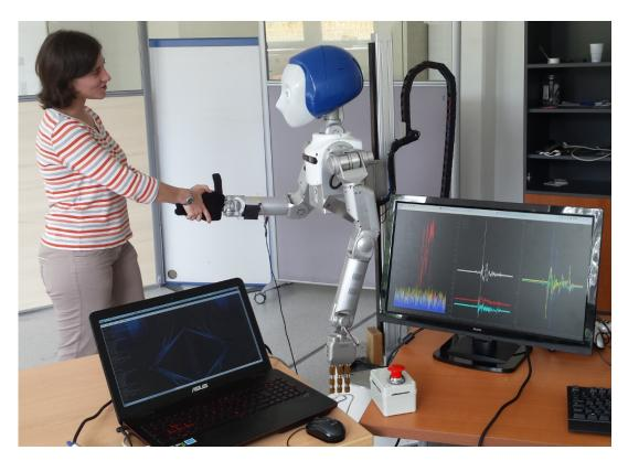
FIGURE 3.14: Human-Robot handshake using Meka humanoid robot
