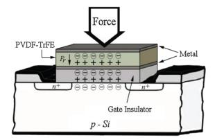
FIGURE 2.5: Schematic of a piezo-sensitive cell based on FET transistor (extracted from Adami et al., 2012)
