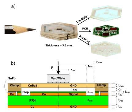
FIGURE 2.10: Modular multi-modal sensor (extracted from Mittendorfer and Cheng, 2012). a) Picture of a the full module; b) Schematic of a Piezo-capacitive cell.
