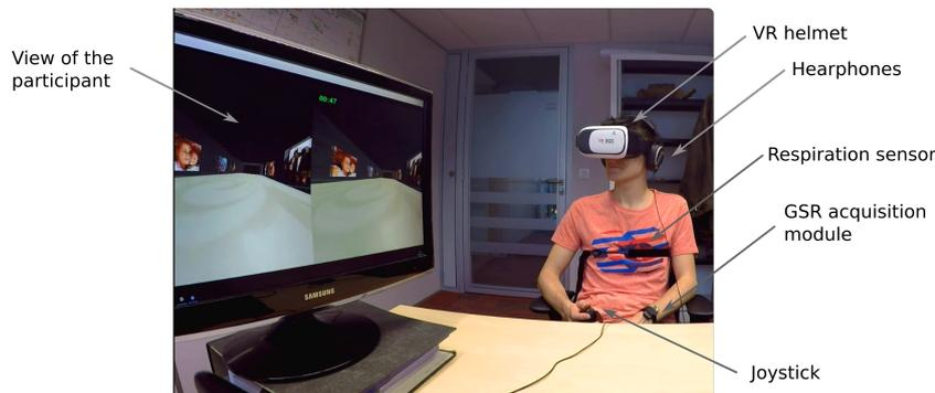
FIGURE 4.4: Experimental setup
