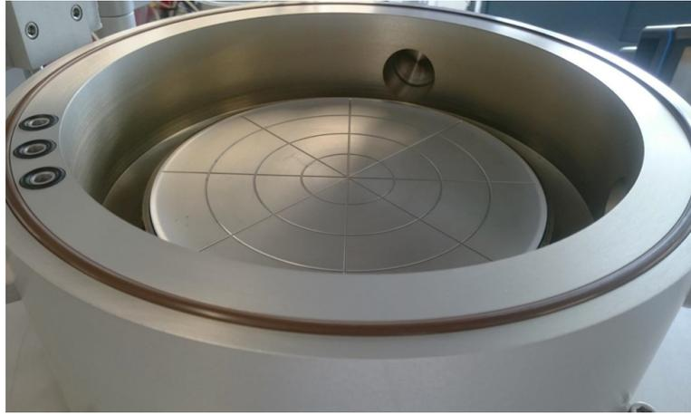
**Fig. II.2:** Picture of the substrate electrode in the RIE reactor (open chamber), the electrode has an external diameter of 8 inches (20.3 cm)
