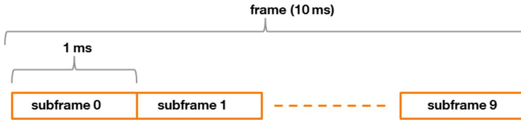
Figure 3.4: LTE-A Frame Structure
