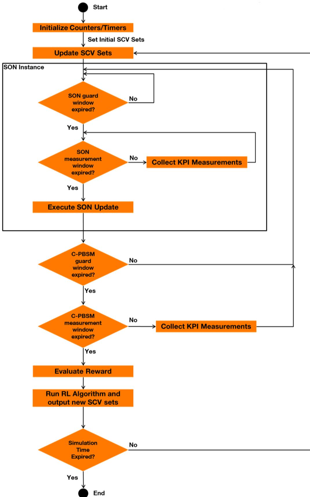
Figure 3.5: C-PBSM and SON Functions Simulations Block Diagram
