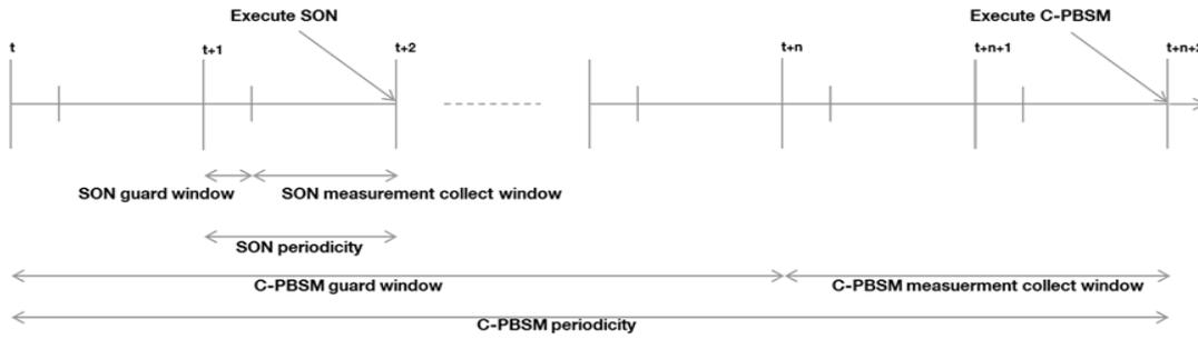
Figure 3.6: C-PBSM and SON Functions Timers
