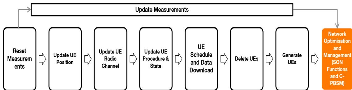
Figure 3.7: LTE-A Simulator Block Diagram
