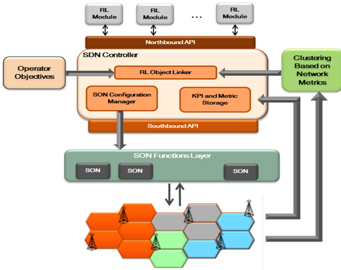
Figure 5.3: C-PBSM based on Distributed RL deployment through SDN
