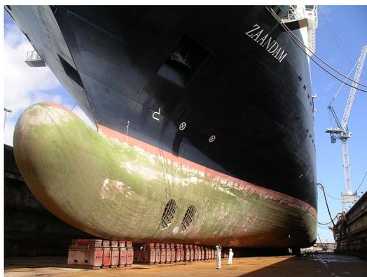
Figure 3.1: Bulbous bow of the passenger ship Zaandam in drydock (source: [72]). A bulbous bow is used to reduce its wave resistance.
