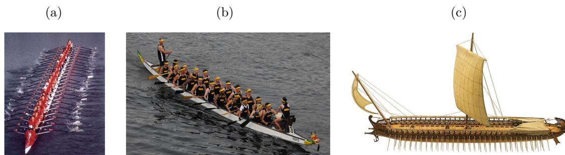
Figure 5.6: (a) Picture of the *Stämpfli Express*, a rowing boat with 24 rowers measuring 44 m (source: [101]). (b) Picture of a *Dragon* boat, a racing boat with 22 persons on board among which 20 rowers (source: [9]). (c) Wood model of a Greek trireme, a boat used in the antiquity which derives its name from its three rows of oars (source: [3]).
