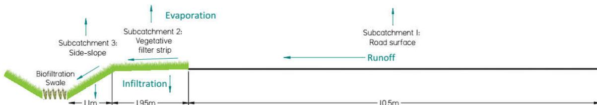
Figure 23 : Geometry of the modeled system
