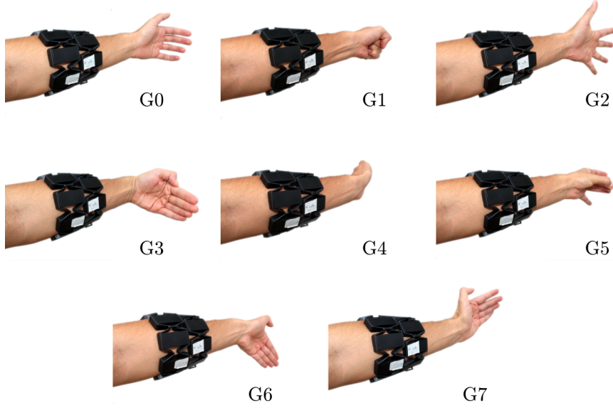
Figure 3.5: Representation of the library of gestures of the UC2018 DualMyo data set. By order, the gestures are: (0) rest, (1) closed fist, (2) open hand, (3) wave in, (4) wave out, (5) double-tap, (6) hand down, (7) hand up.
