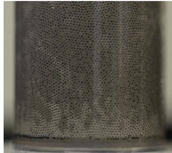
Figure 5.6: Bottom of cement foam sample 15 minutes after production containing TTAB,  $R = 300 \mu\text{m}$ ,  $W/C_f=0.69$  with perfluorohexane ( $\tau_y < 1 \text{ Pa}$ ). Sample diameter is 2.6 cm.
