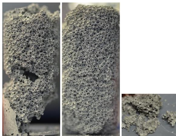
Figure 5.13: Comparison of samples with big bubble size (TTAB,  $\Phi=0.87\%$ ,  $R=1000$   $\mu\text{m}$ ) after free drainage ( $W/C_f=0.44$ , left) and when drainage has been prevented by rotation (center and right). Rotation sometimes leads to weak samples that break when they are demolded ( $W/C_f=0.49$ , right). Sample height is 6 cm.
