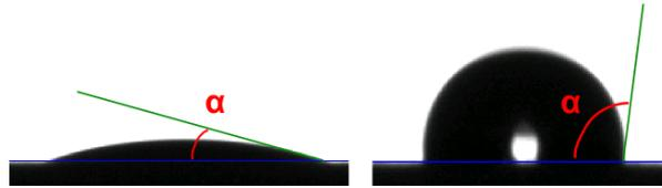
Figure 2.4: Example of pictures used for contact angle measurement. Left : reference sample,  $\alpha = 19.6^\circ$ ; right : sample with initial concentration of Bio-Terge of 25 g/L,  $\alpha = 103^\circ$
