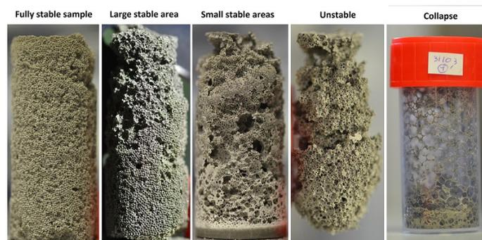
Figure 4.4: Example of samples illustrating each stability class. Sample height is 6 cm.
